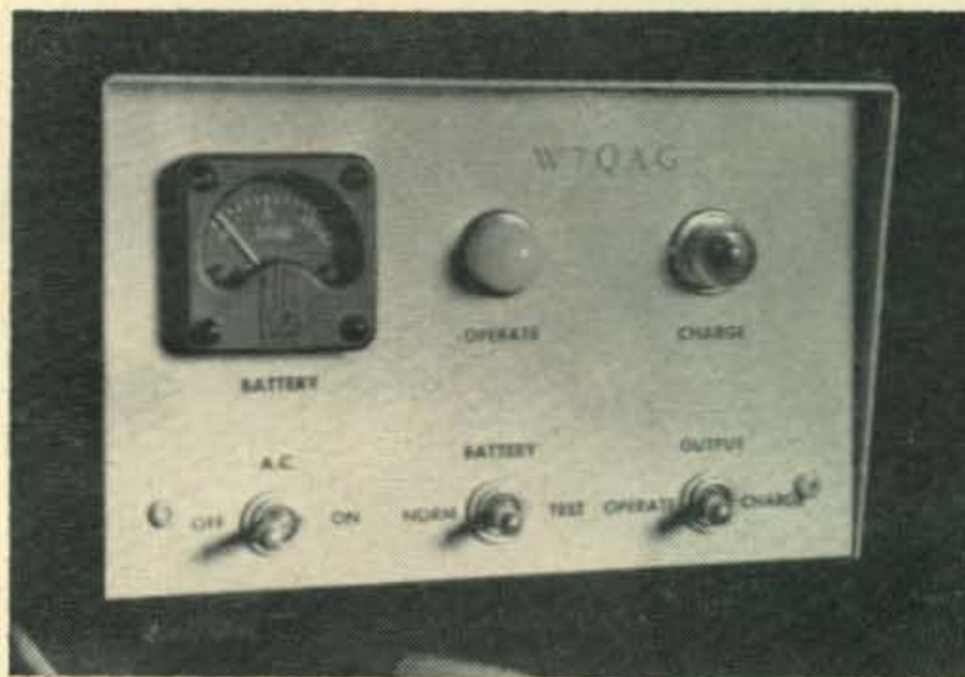
A power supply capable of supplying 12 volts d.c. for charging Alkaline batteries, doubling as a battery eliminator when portable operation is not required.
