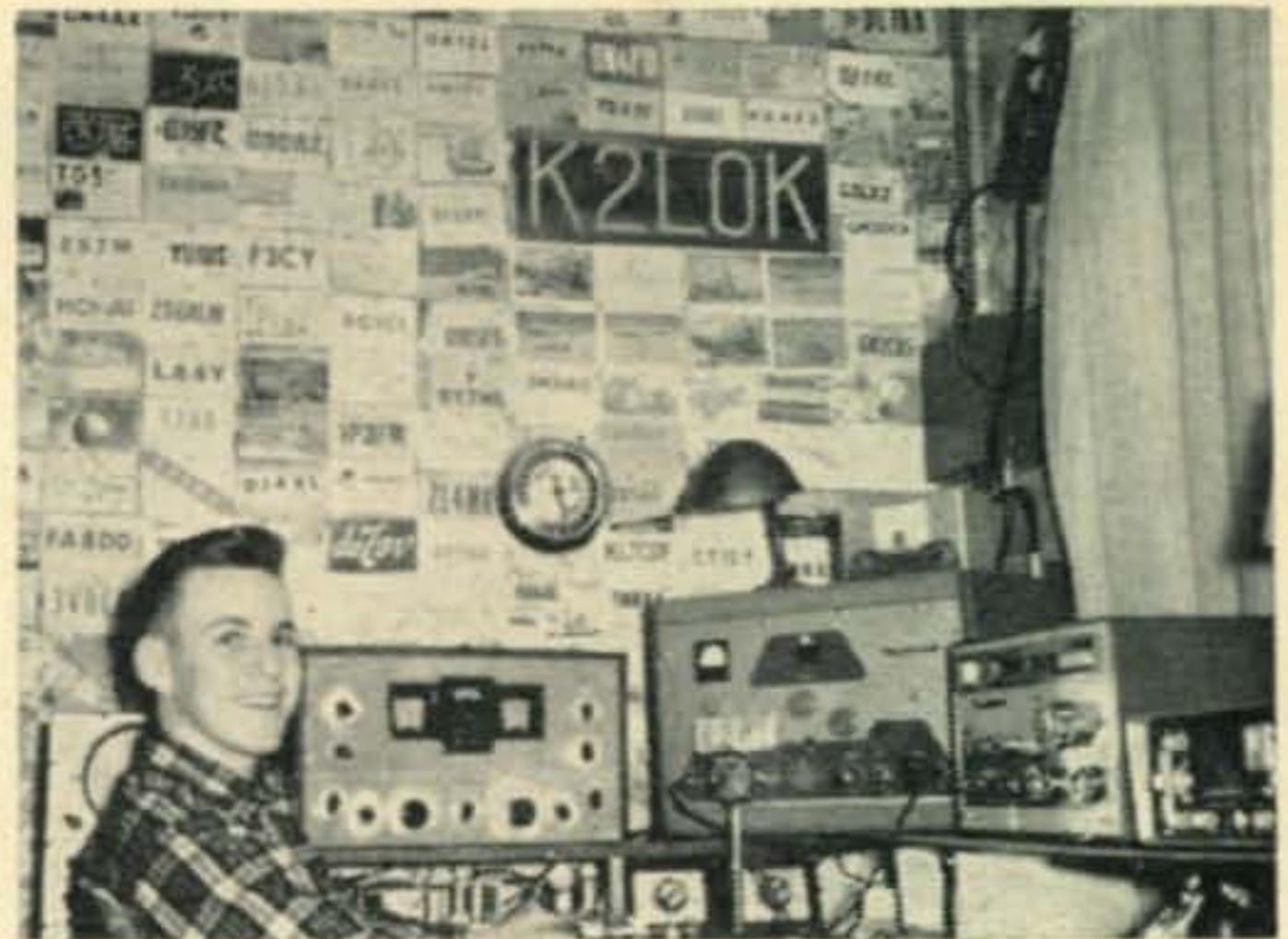
Here's New York state winner for 144 mc, Jeff Miller, K2LOK/2, in Chautauqua County. Equipment used was the Heath Seneca and HQ-129X with Ameco converter and preamplifier hooked into an 8/8 "J" beam up 50'. Elevation, 1750'. Congratulations, Jeff!
