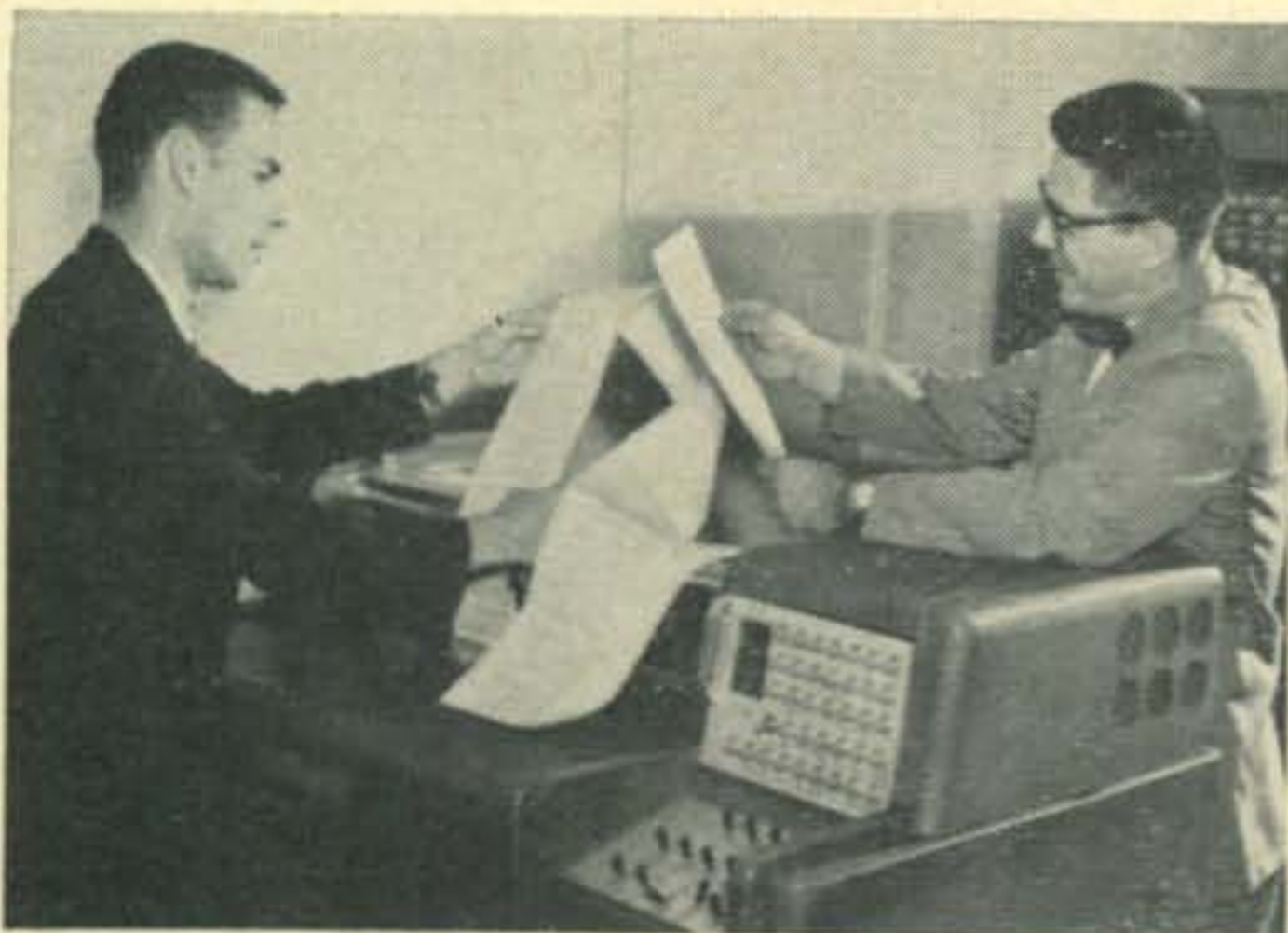
Computer operator Herb Chaplin (left) and the author inspect a strip of QSL's just printed out on the High-Speed Printer. Just visible over W3EFY's shoulder is one of the two circuit banks which control the reading of information from tape and its printing onto paper. A Uniservo serves as the input vehicle.
