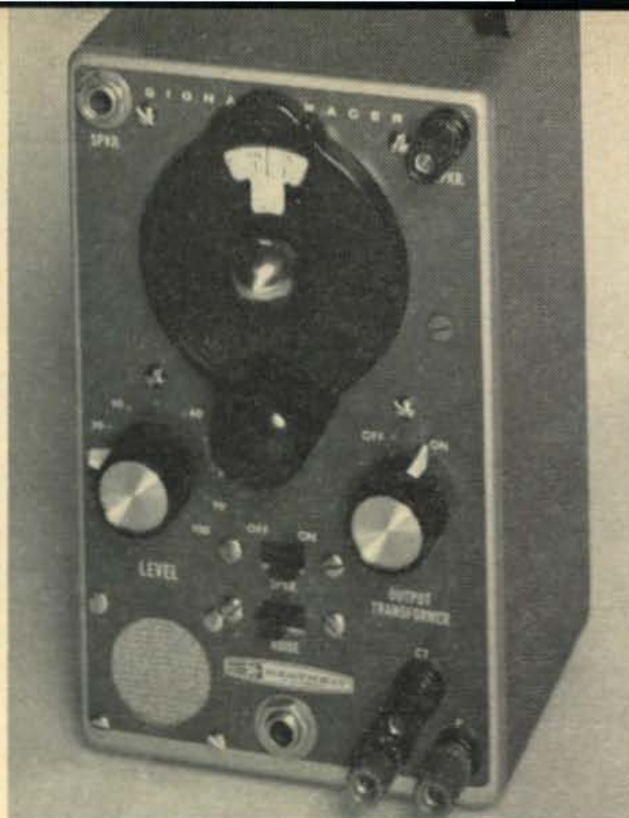
Front view of the combined audio oscillator and signal tracer. A 1½" speaker is now located where the tuning eye formerly was. The National dial covers the old speaker opening.
