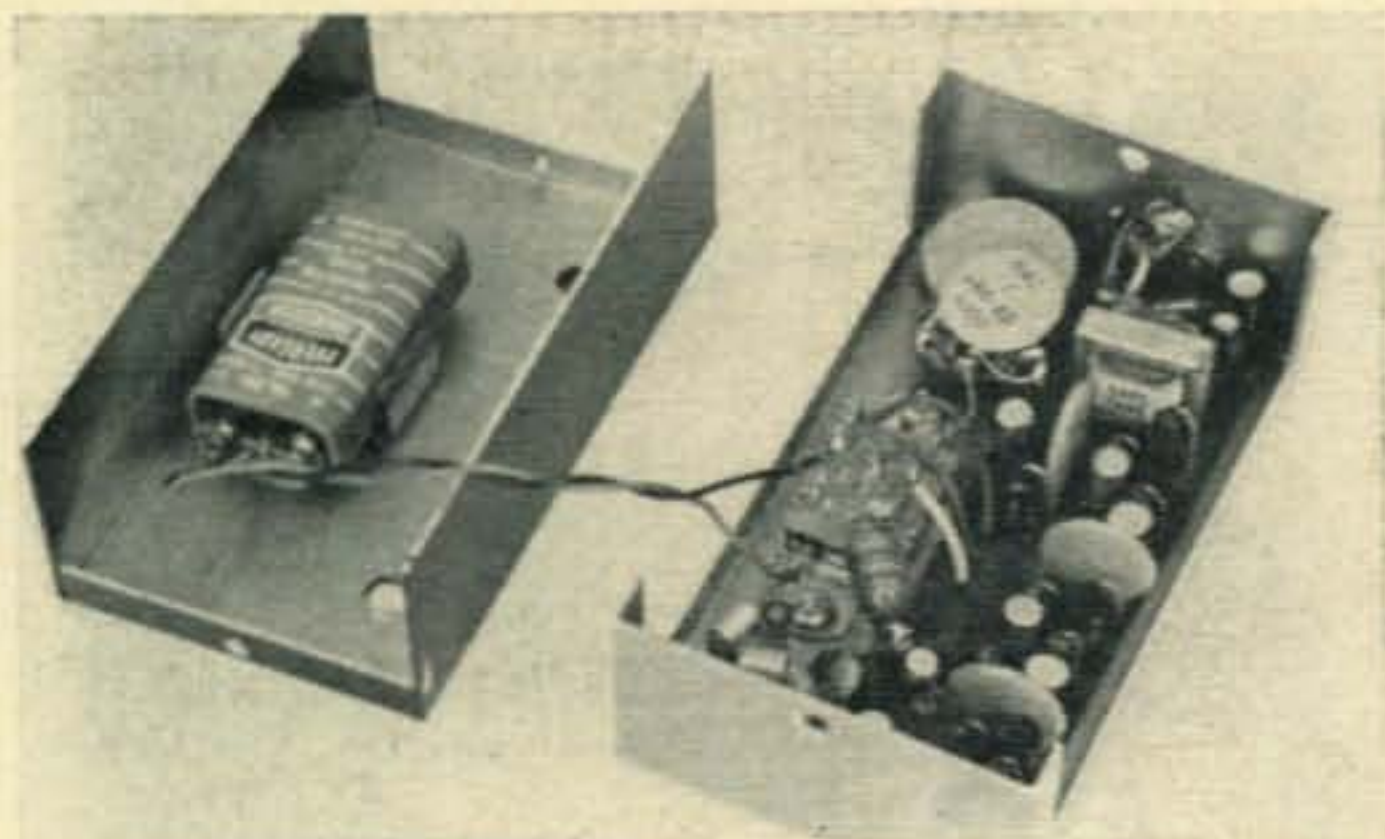
Interior view of the Model C-II. The three transistor stages are mounted on a small printed-circuit board at the right. The other round-ended objects are tiny electrolytic capacitors. A 9-volt transistor-radio battery is held in the cover at the left.
