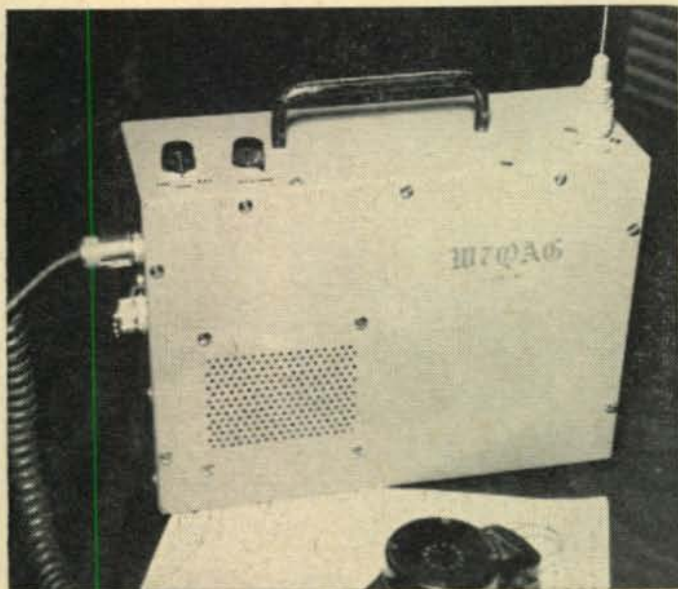
This lightweight 2 meter portable runs over 2 watts input and is completely self contained in a 4½" x 5" x 7" aluminum case.
