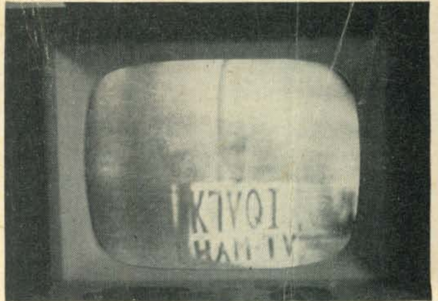
K7VQI's live amateur TV signals as received by K7JQJ four miles away.
