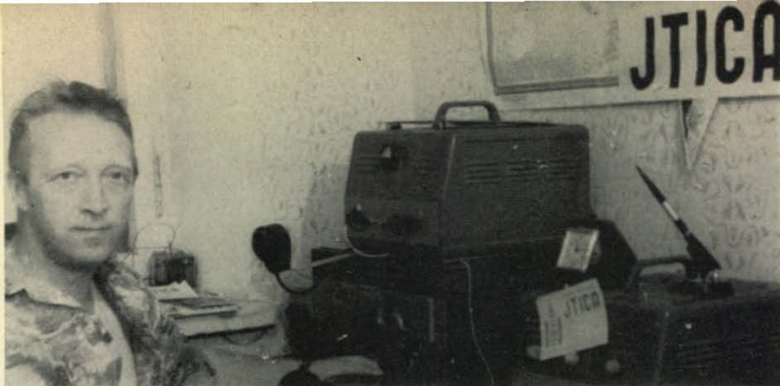
One of the most popular stations on the air at the present time is the gentleman shown here. Vlad, JT1CA put Mongolia on the Zone 23 s.s.b. map for the first time with this home brew rig. The transmitter runs 200 watts of s.s.b. or c.w. on 7 and 14 mc and c.w. on 3.5 mc (3510) the antenna is a ground plane. (Tnx W4CKB)
