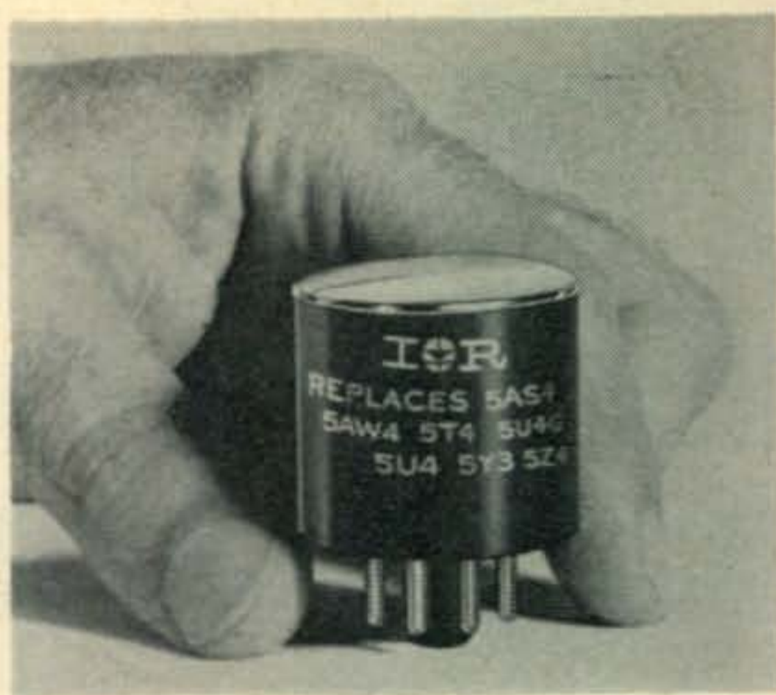
A quick and easy substitute for many rectifier tubes is this International Rectifier ST-14 silicon rectifier replacement unit, handling the 5Y3, 5U4, 5T4, 5AW4, 5Z4, etc. Some applications may require external voltage dropping resistors.
