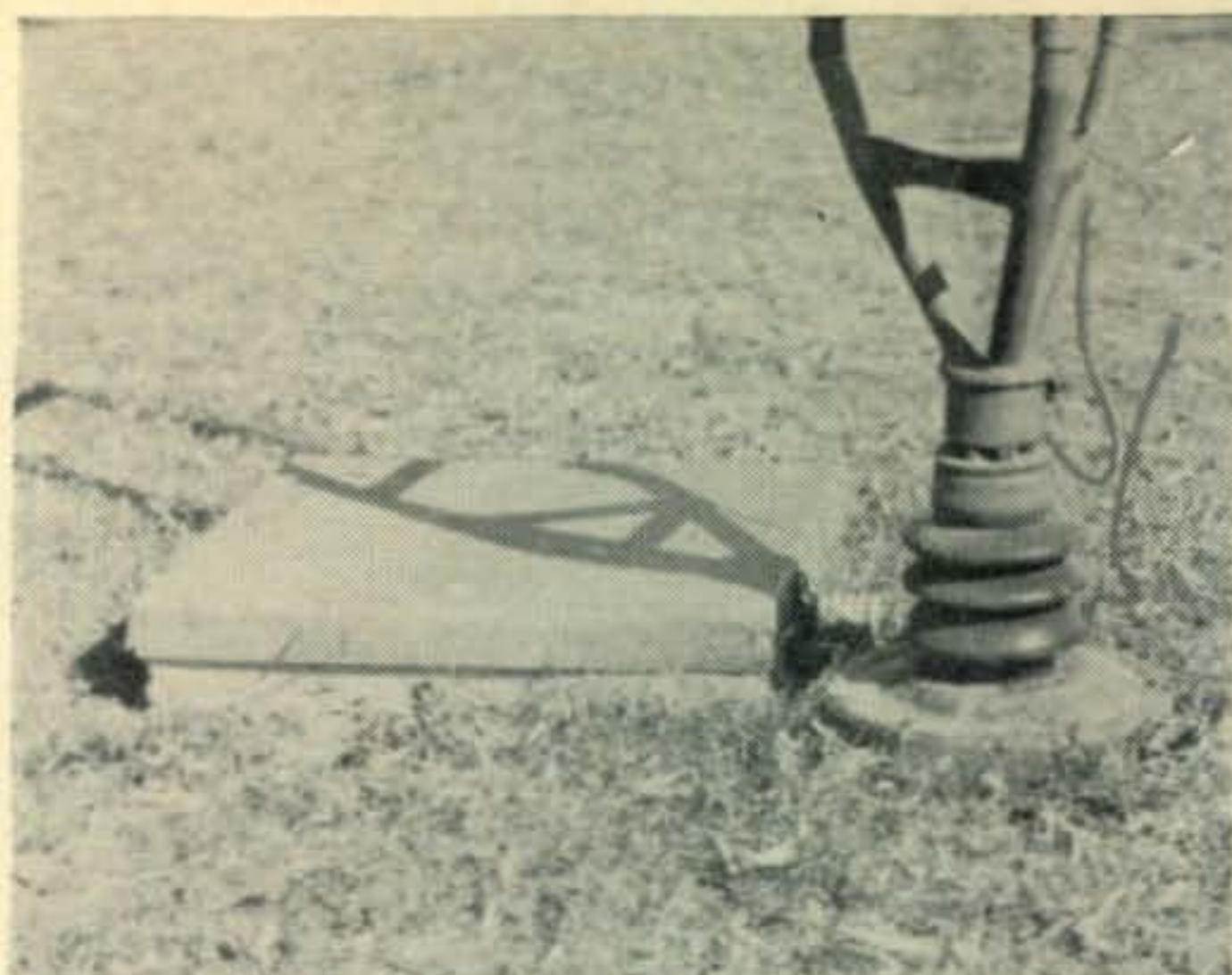
Fig. 1—(A) Construction of the ball-joint base. Sheet steel \frac{3}{8} " thick is used and the pieces are welded together as shown. (B) Lightning arrester details.
