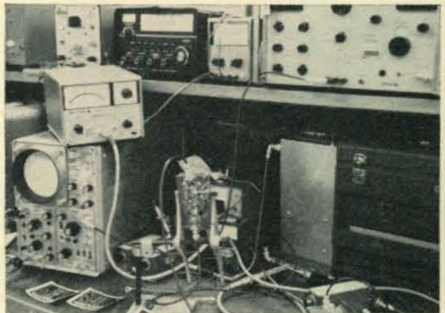
OSCAR III linear amplifier being tested at Project OSCAR Headquarters. The linear amplifier was measured to have a p.e.p. output of 1 watt, and is ready to go. (Photo courtesy WA6RDZ)
