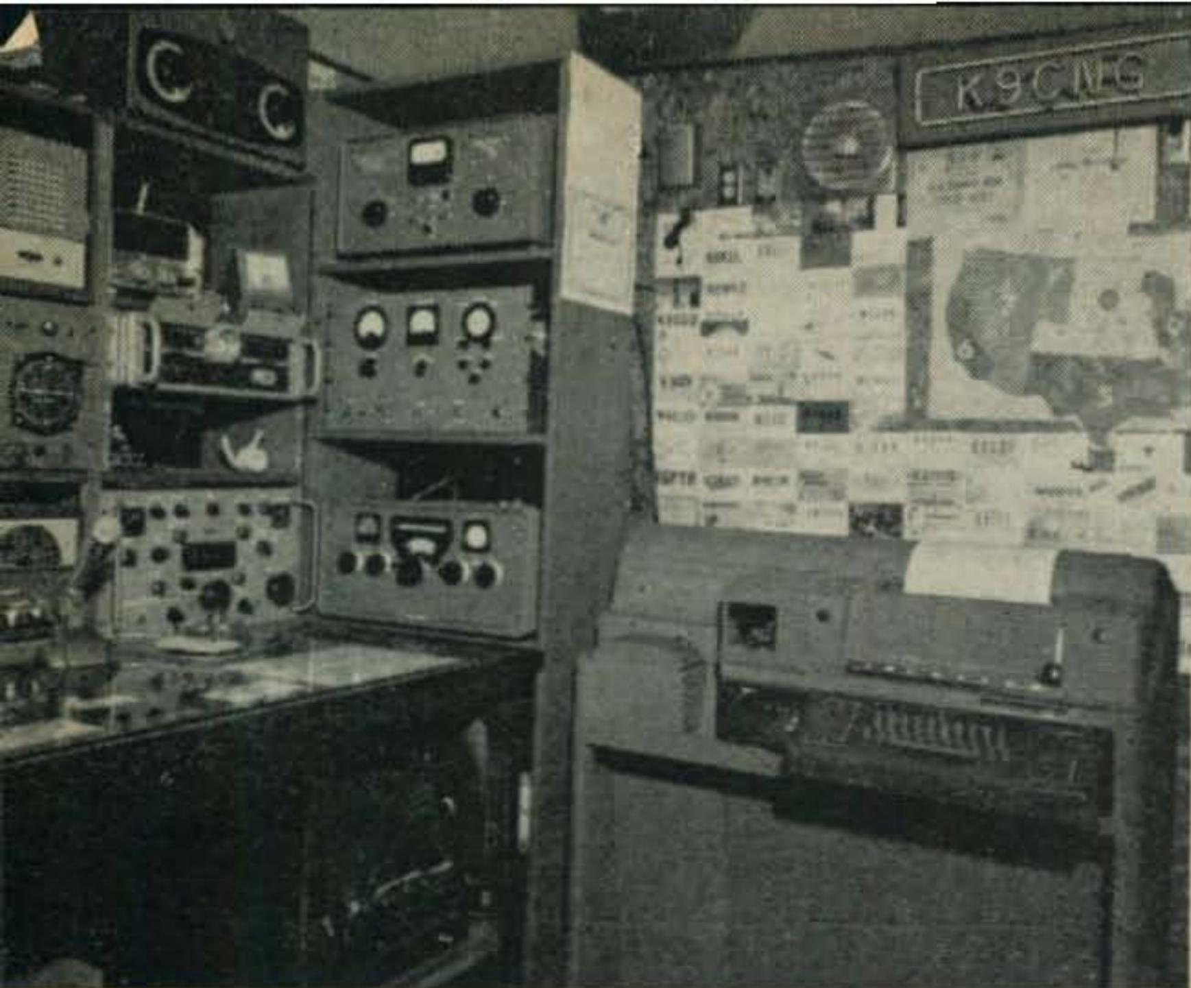
K9CNG of Vandalia, Illinois operated by Al Hourigan, uses a Model 28ASR and a Model 14 typing reperforator. Receiver is a 390A and the TU is a CV-89 and the transmitter is a 200-V.
