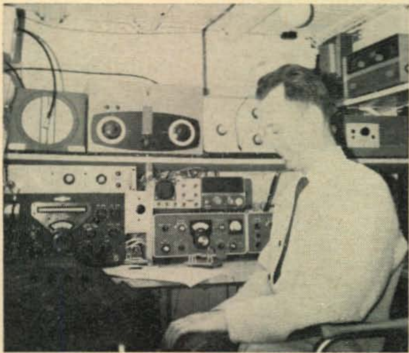
Finn Rambech operating LA6VC at Trondheim, Norway. A 32S3 is frequency-shifted by a Lorenz tape printer with keyboard. Antennas are a 3-element tri-bander up 50 feet, a 10/80 meter vertical, a sloping dipole for 80 and a 10/40 meter ground plane. Finn also works 144 mc with a 10-element yagi.
