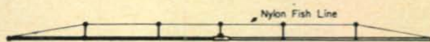
Fig. 2—The director and reflector would sag without the support shown above. Nylon fish line, 100 lb. weight, is stretched through five 5" TV stand-off insulators.
