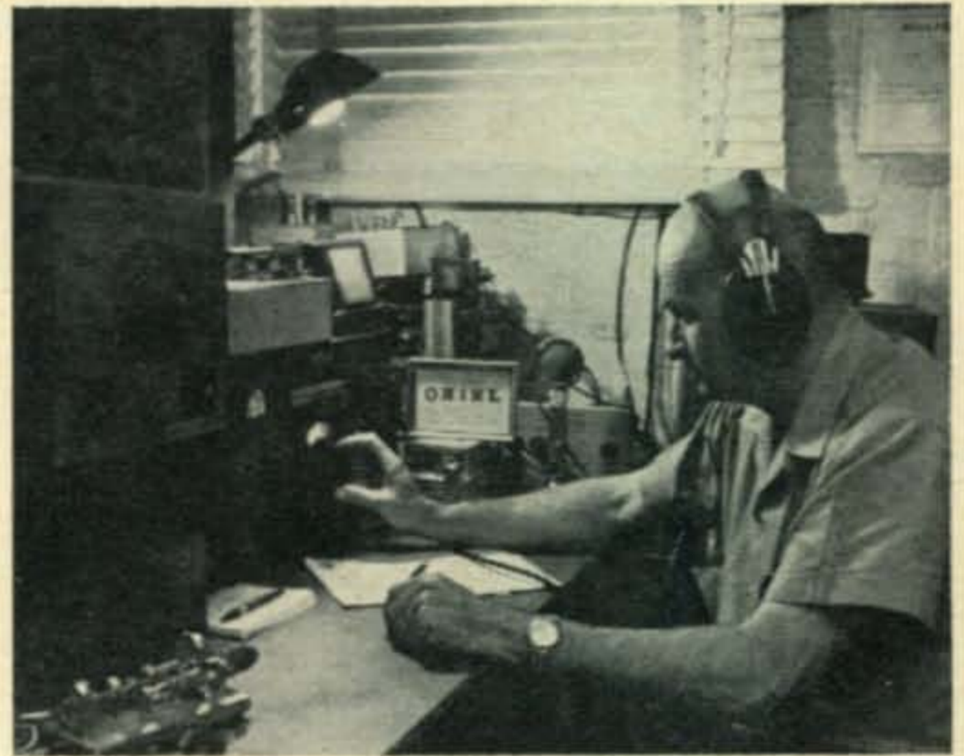
Bill Conkel, W6DNG, of Long Beach, California shown operating the rig with which he established the first two-way 2 meter moonbounce QSO with OH1NL. Running a full kilowatt of c.w. power, the rig uses a pair of EIMAC 4X250B's in the final.
