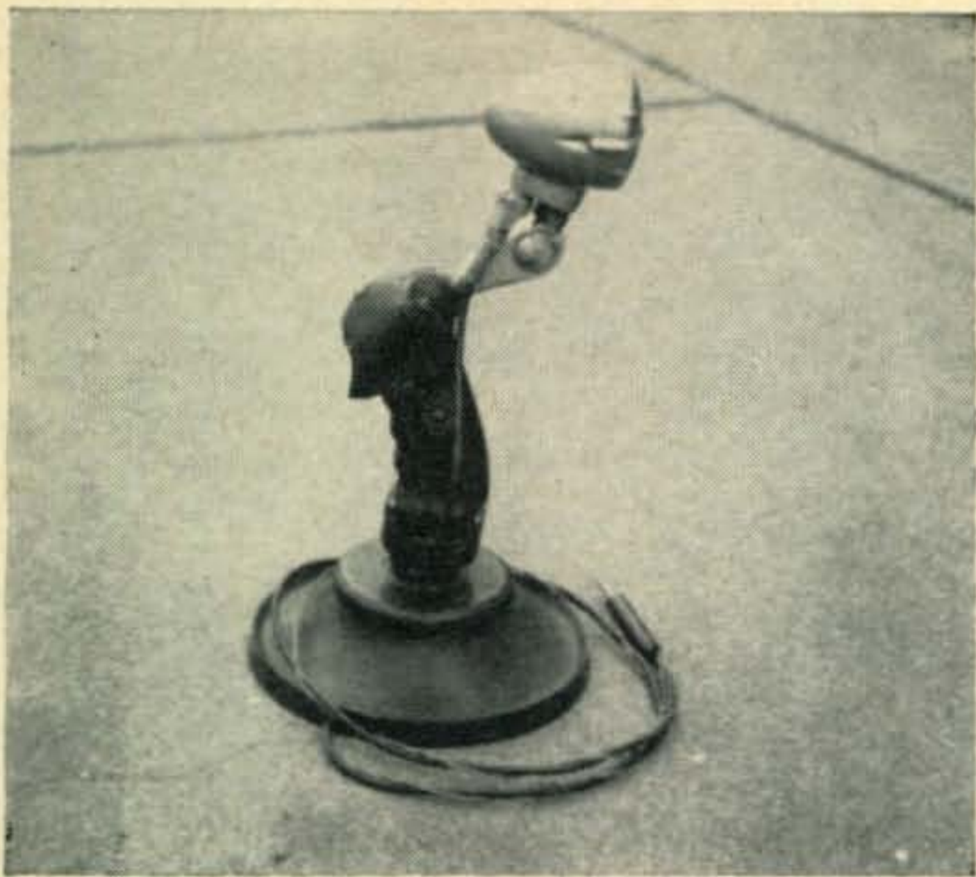
The finished mike stand is made from a surplus gun control assembly mounted on a discarded lamp base. The total cost was one dollar.
