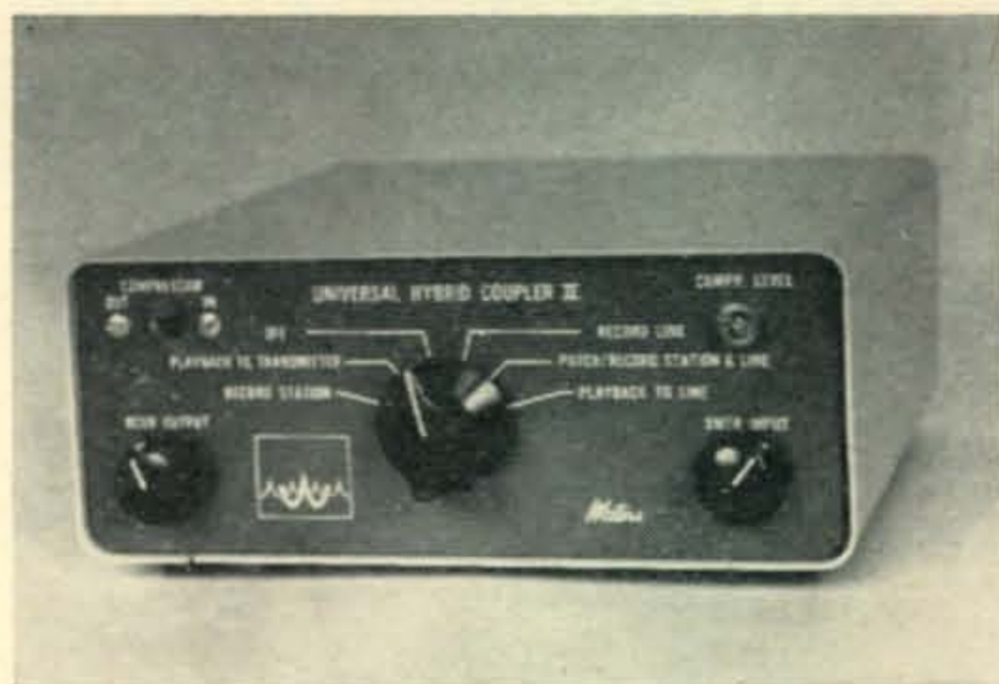
The Waters Universal Hybrid Coupler (Model 3002). The function switch is at the center with the Rcvr Output at lower left and the Xmtr Input at lower right. The Compressor switch is at the upper left, the Compression Level (screw-driver adjust) at upper right. The panel is gray, the case is light gray.
