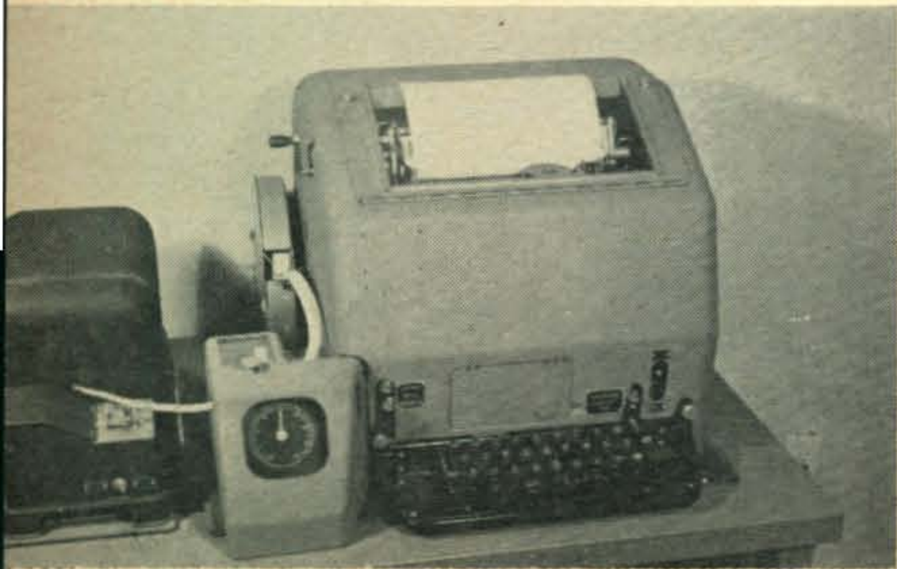
Fig. 10—Teletype Model 19 tape set. The unit on the right is a Model 15 page printer. The left unit is a Model 14 transmitter distributor. The center unit is a perforator-counter, the function of which is explained in the text
