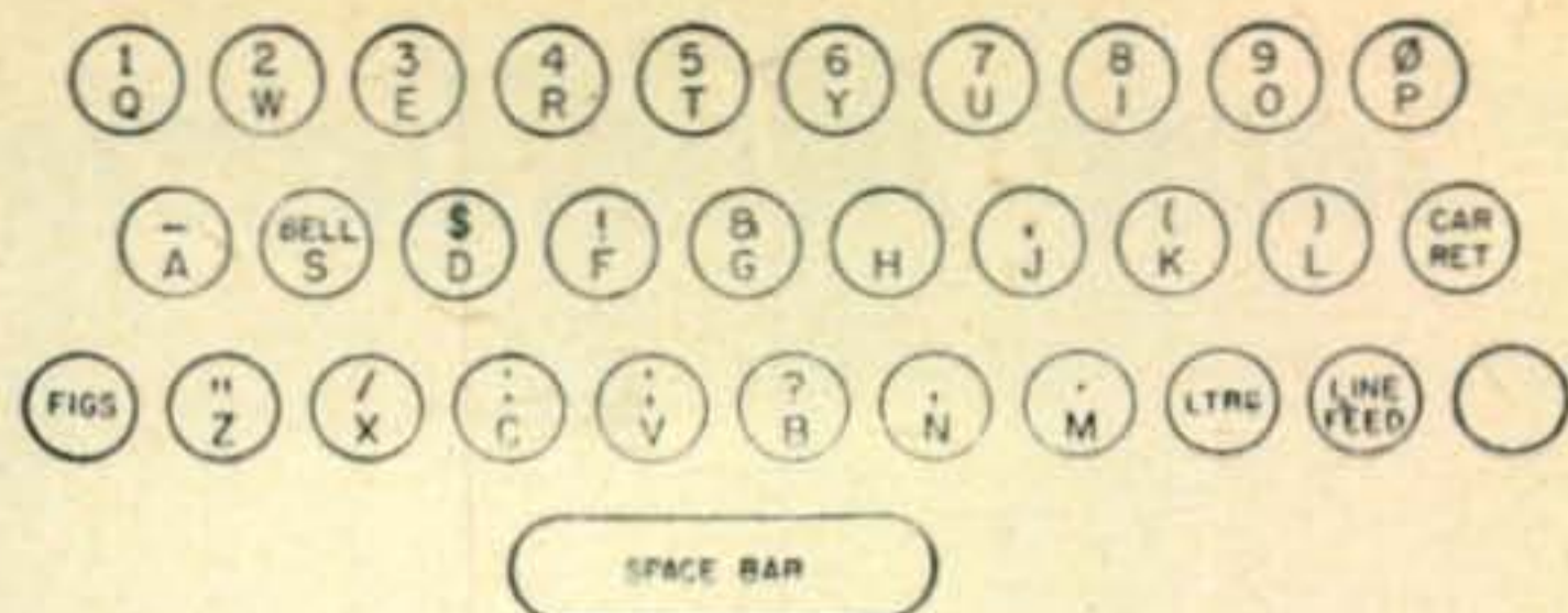
Fig. 12—The most commonly used RTTY keyboard arrangement.
