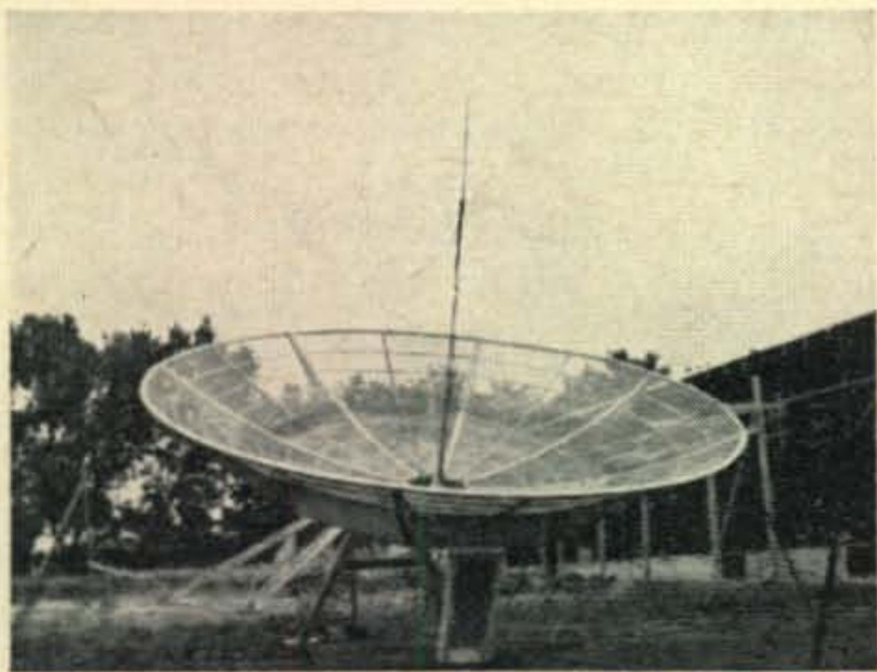
W9GAB's moonbounce antenna system consisting of a 15 foot homebrew parabolic reflector fed with a dipole and reflector. Transmission line is 15 feet on RG-33U.
