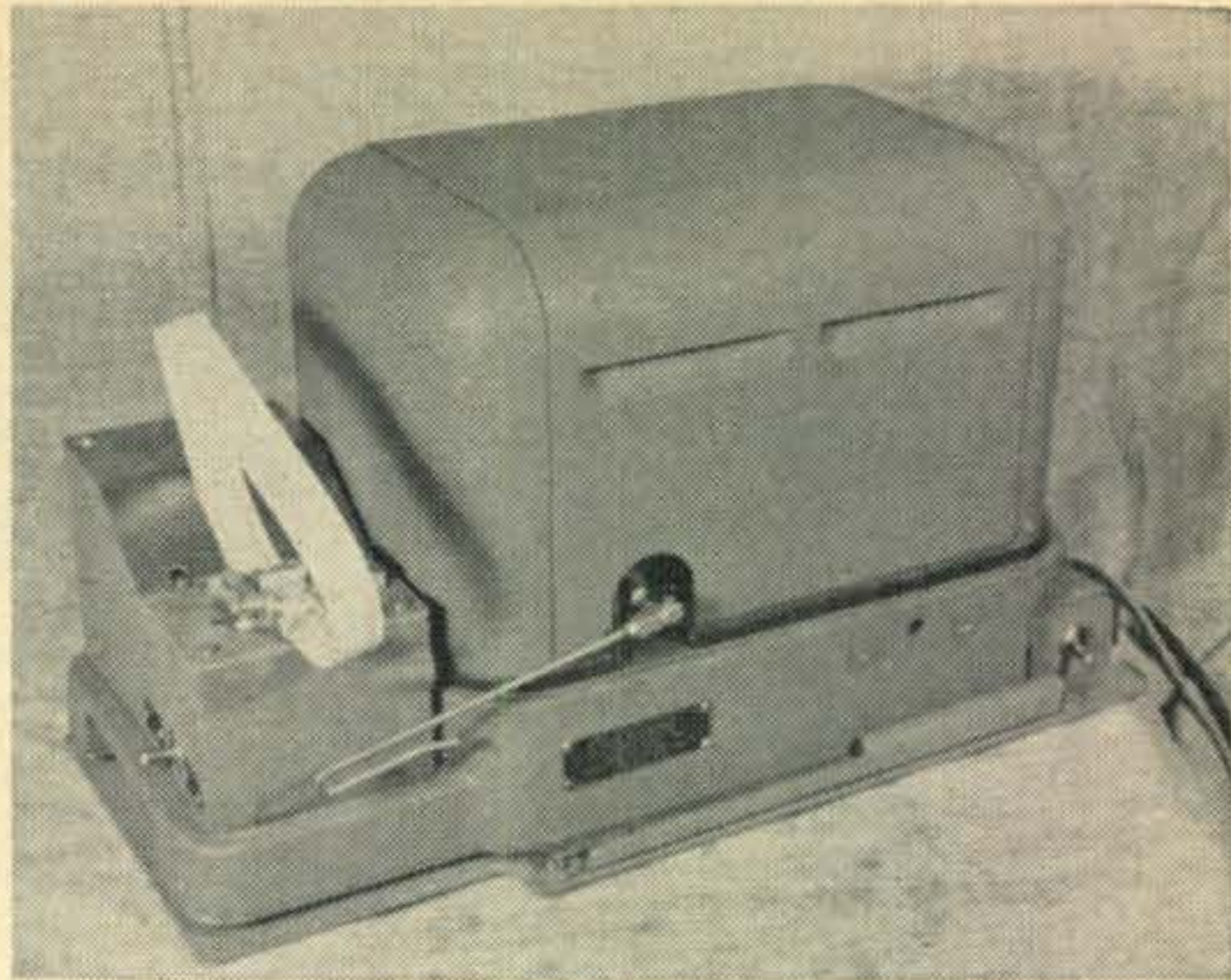
Fig. 8—Teletype transmitter—distributor Model 14 used to transmit pre-punched tapes at speeds up to 60 w.p.m. The closed loop tape repeats the message until the machine shuts down.
