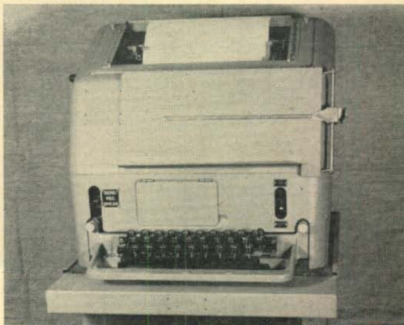
Fig. 4—Teletype Model 15 page printer used for both Transmit and Receive functions.
