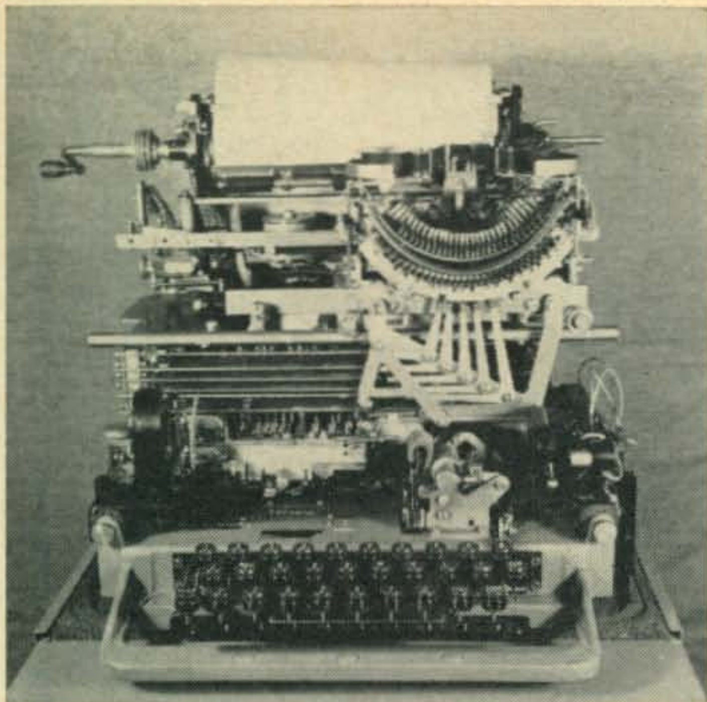
Fig. 5—Interior view of the Model 15 page printer.
