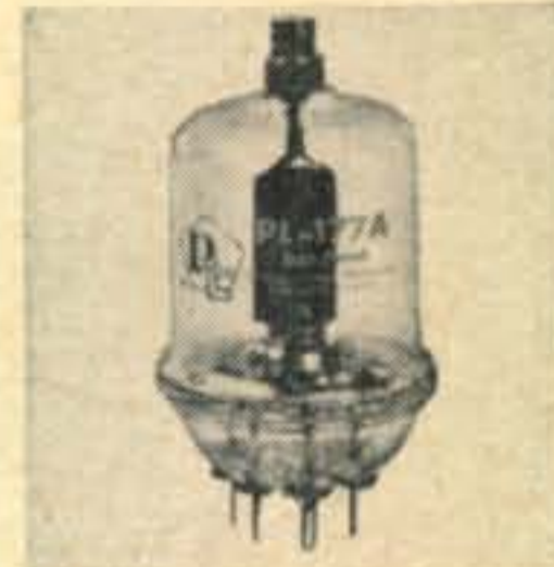
PL-177A 75W beam pentode. To 175mc. Highly efficient at plate voltages as low as 600v.
