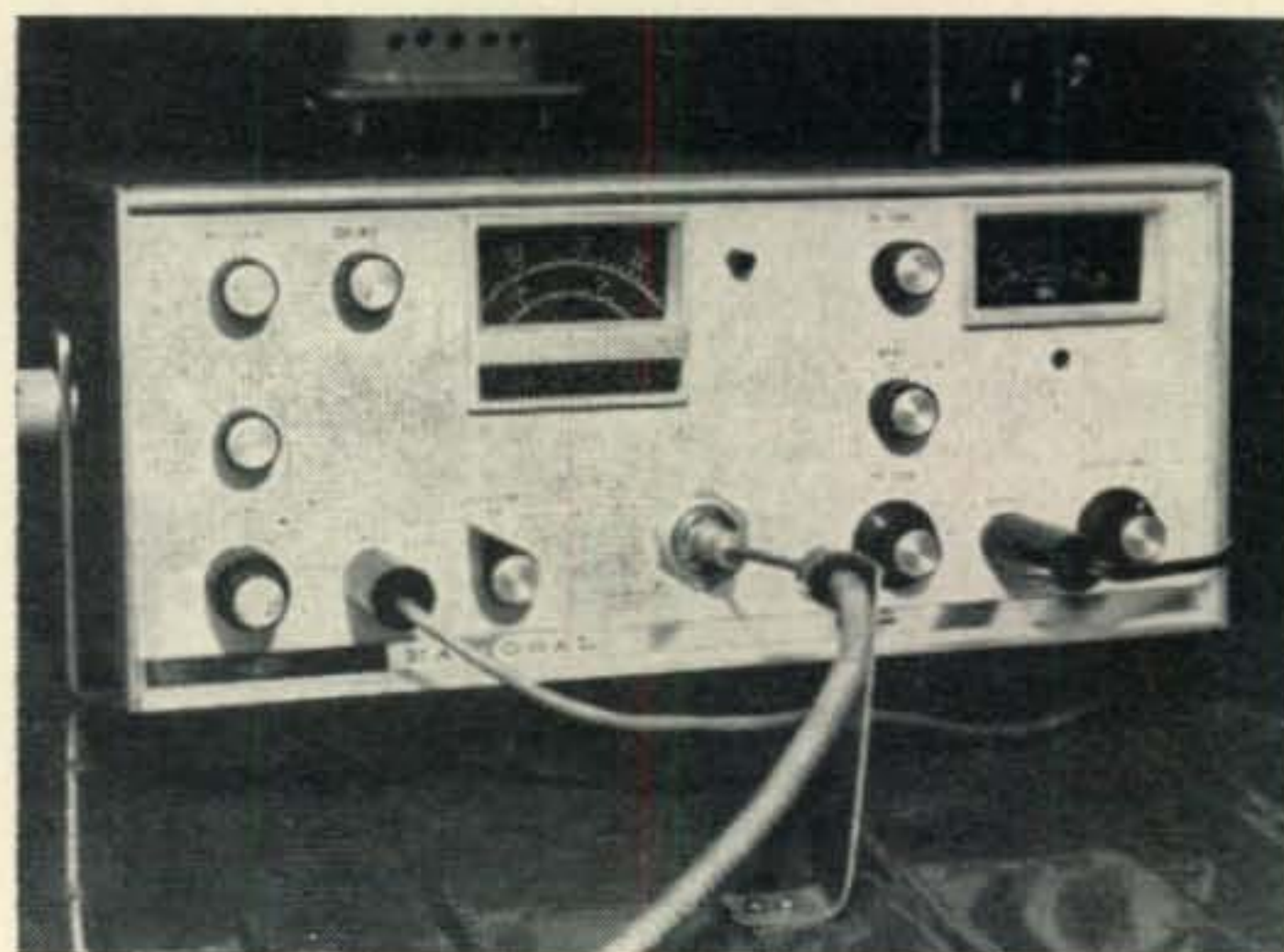
Close-up view of the NCX-3 showing the flexible cable support bracket and the coupling to the receiver.
