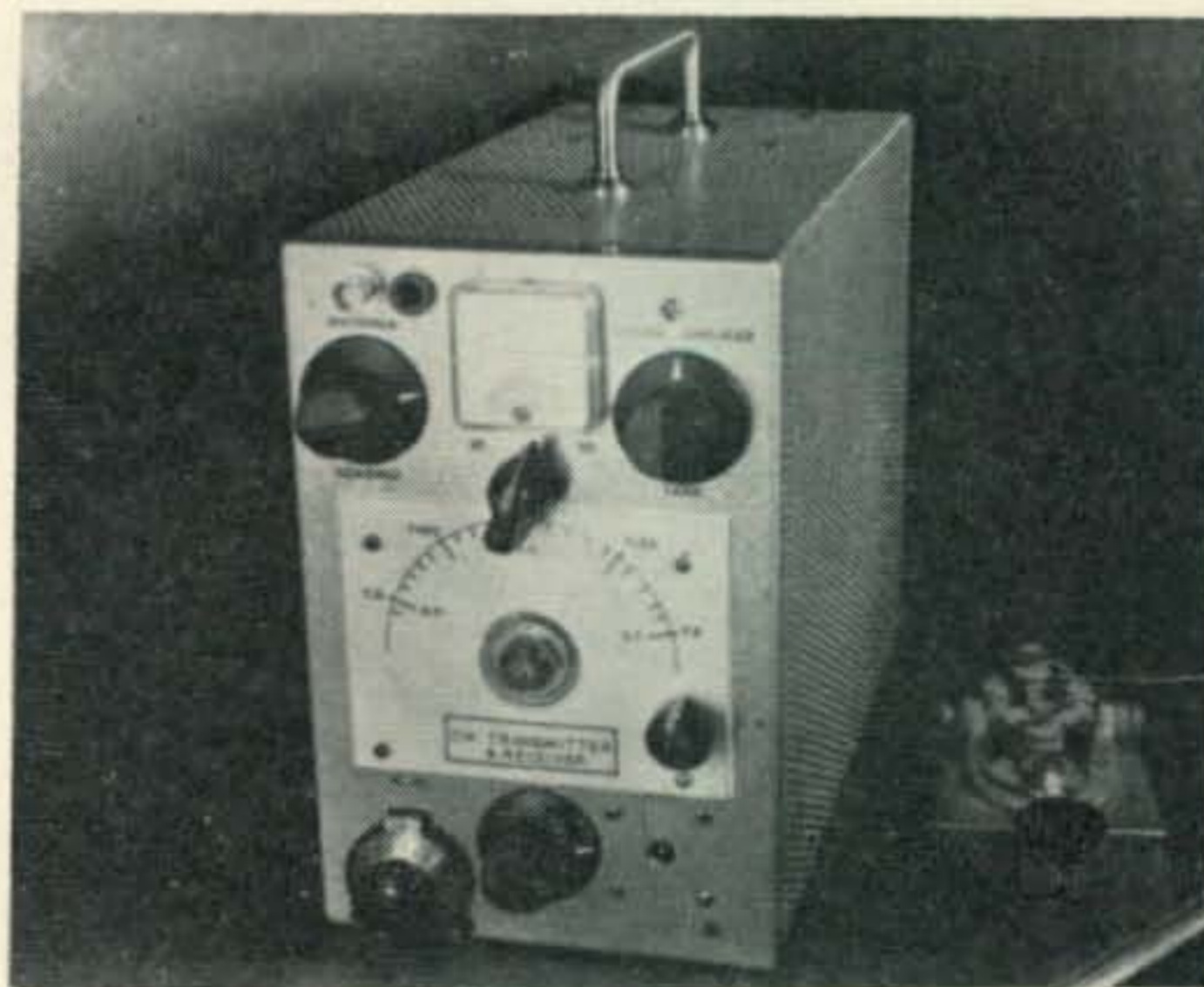
Front view of the 80-40 meter c.w. transmitter-receiver vacation package shows the control layout. The controls are from left to right on the bottom, v.f.o., AUDIO GAIN, RECEIVER TUNING. The b.f.o. can be adjusted through the hole in the panel to the right of the AUDIO GAIN control. The transmitter controls across the top are LOADING, BANDSWITCH and TANK TUNING.
