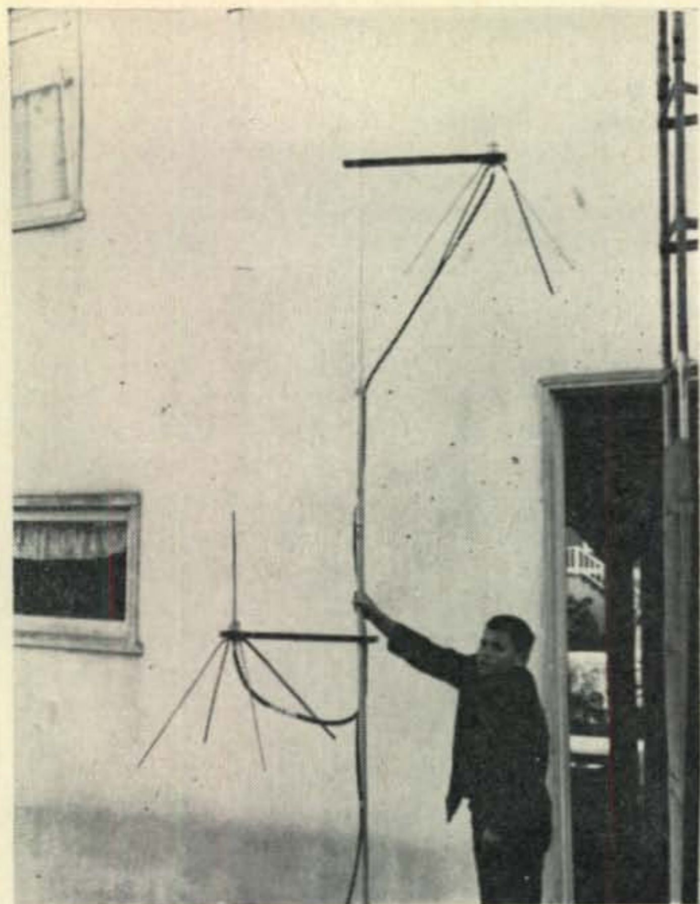
Two 2 meter dipoles are shown set for bi-directional operation. This will provide from 2 to 3 db gain in both directions. Note how the feed cable for the lower antenna is brought up from the bottom to try to reduce minor lobes. The lad with the happy expression is Tom, the author's son.
