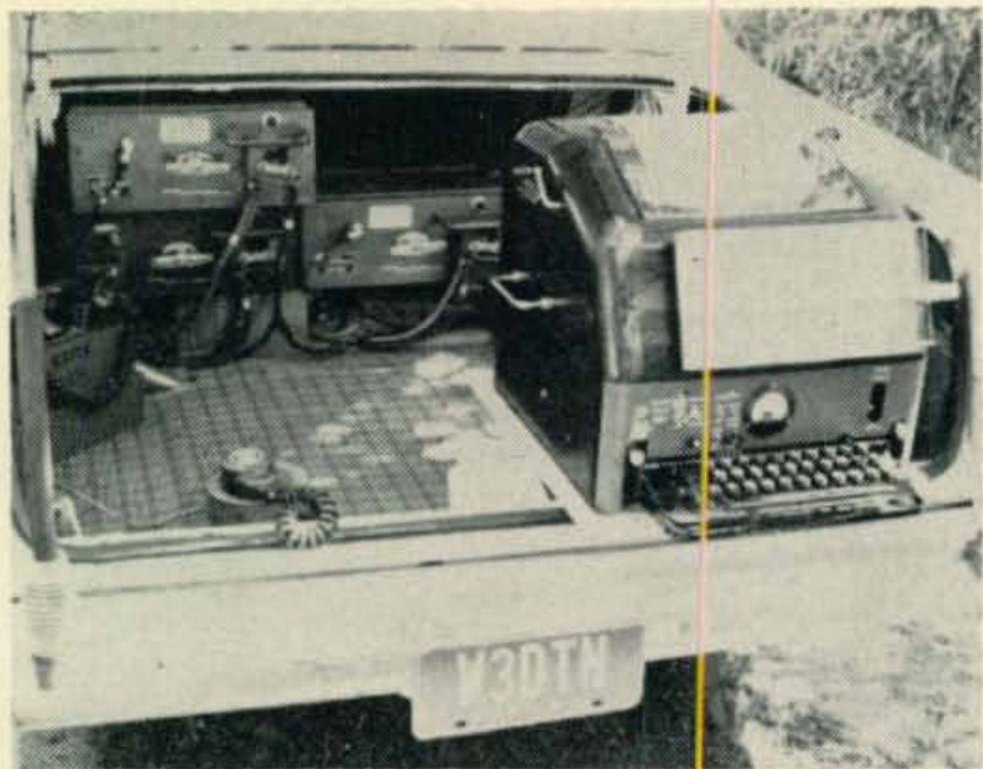
Inside the trunk of W3DTN mobile RTTY. Note the three Motorola f.m. sets; one for 52.60, one for 146.70, and the third on the local radio club channel.
