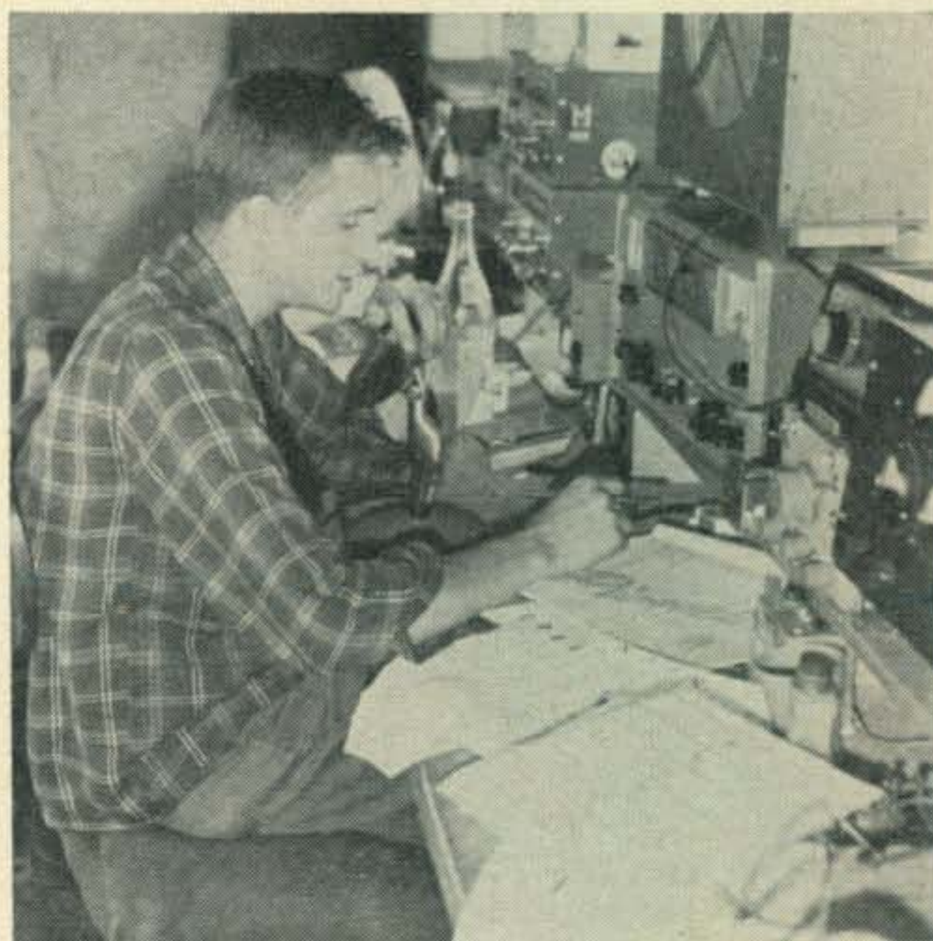
Here's a shot of Les Johnson, WA2WCE, hard at work hamming it up from his converted Navy bus. Les and WA2GHN frequently operated portable from Howard Hill, near Mayville, New York with a homebrew 4-125A final at 300 watts, excited by a homebrew "Lil Lulu." Receiver is an HQ-110 with Ameco converter. Antenna—and remember this is a portable job—is a stacked 6 over 6 wide-spaced Telrex configuration at 50 feet for six meters.
