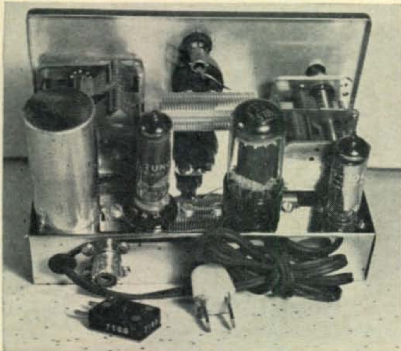
Rear view of the 16 watt crystal controlled oscillator shows the filter on the left, followed by the 50HC6 oscillator, 50L6 power amplifier and an 0A2. The antenna tuning capacitor (a dual 365 mmf broadcast variable with both sections paralleled) is on the left. The plate circuit is tuned by the two gang broadcast variable on the right but only the large section (365 mmf) is used. The coil is mounted on porcelain feed through insulators obscured by the tubes. The output indicator neon bulb can be seen just above the meter on the front panel. The SO-239 antenna connector is on the rear chassis lip to the left.
