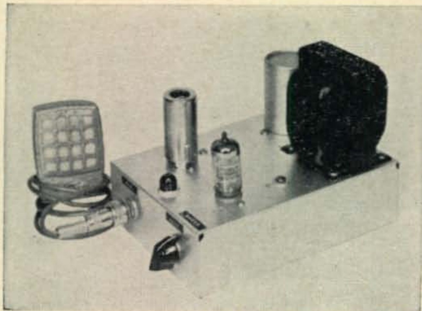
View of the Vox Key showing the simple arrangement of parts. Note the indicator lamp up front.
