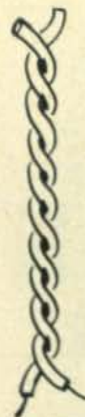
Fig. 1—A gimmick condenser. Notice the ends are not soldered together. To decrease the capacity, simply trim the twisted wire shorter.
