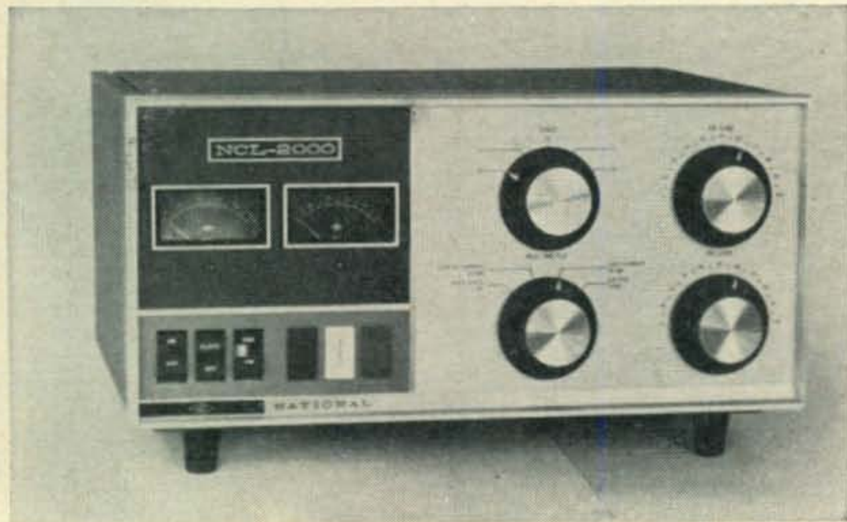
The NCL-2000 linear power amplifier. It is housed in a perforated tilt-up cabinet and has a heavy extruded-aluminum panel. Plate meter is at left with multi-meter at right of it. The power, plate, and c.w./s.s.b. rocker-type switches are at lower left with the indicator lamp bezels at their right. The bandswitch is at top center with the multi-switch below it. The P.A. tuning and loading are at right.
