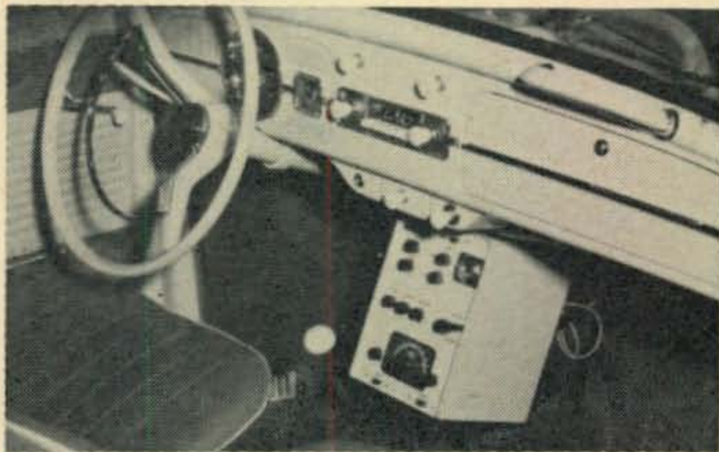
View of the repackaged Gonset IIB snugly hung under the dashboard of the VW. It does not interfere with the driver or passenger.
