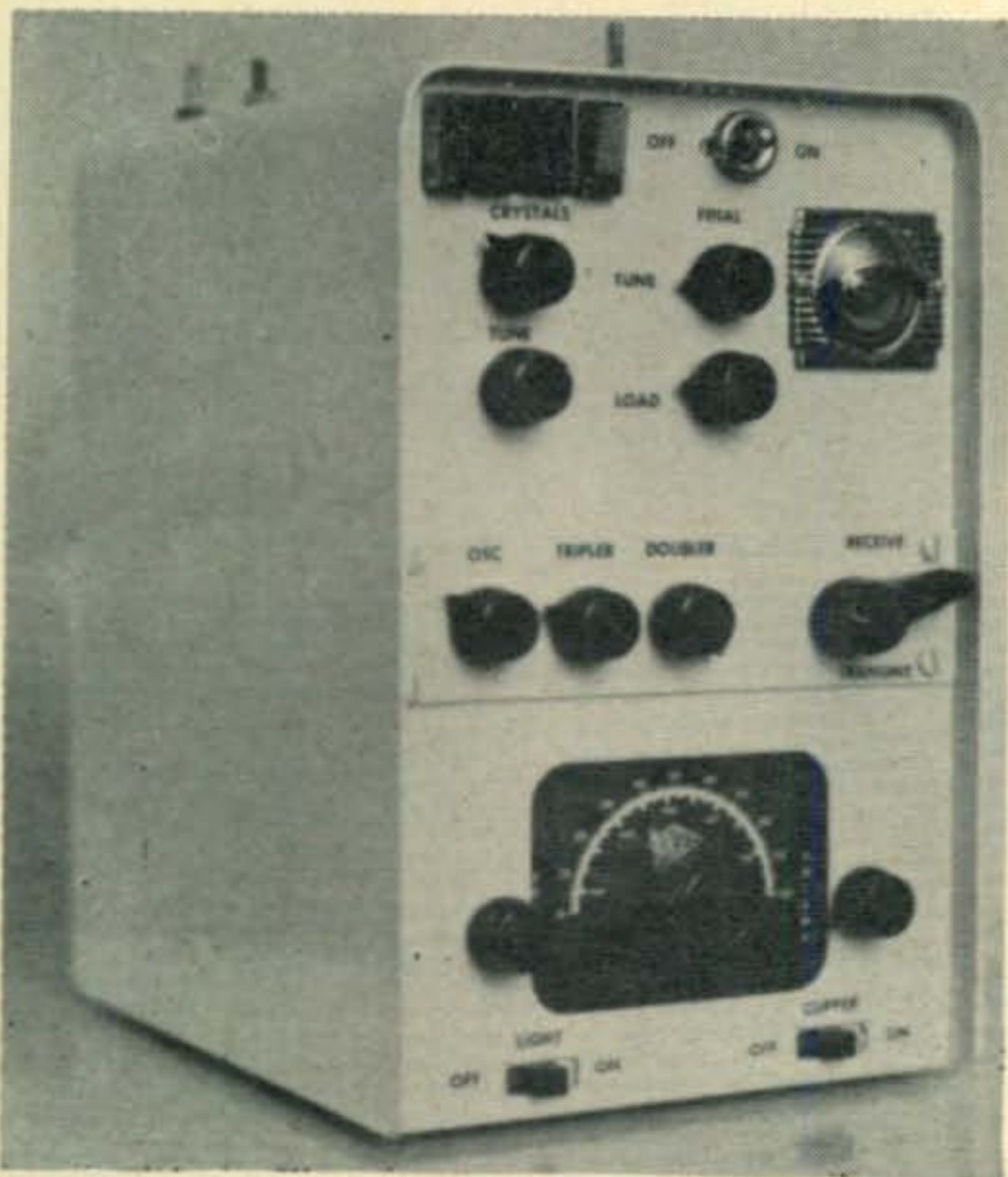
Front view of the Gonset 11B repackaged in the V.F.O. case. The power supply is located behind the rear seat and the car speaker is used for the receiver. The ON-OFF switch that was added is at the right of the crystals.
