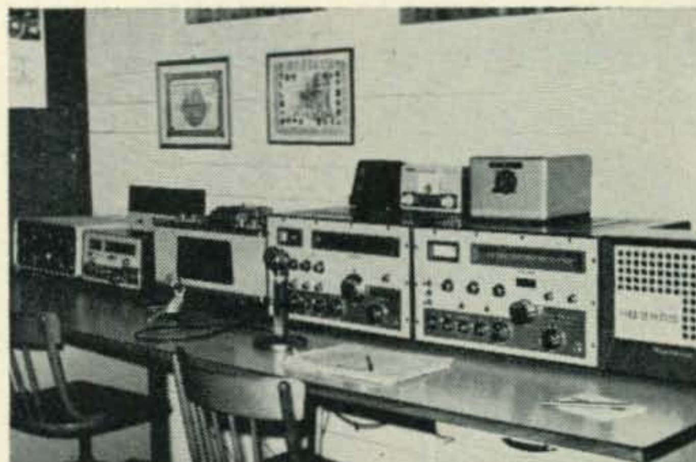
This neat station is HB9RAS. The station was set up at the Swiss National Exhibition in Lausanne. Equipment includes HX-10 and HX-20 transmitters, RX-1 and SB-300 receivers. Antennas are a TA-33 Jr. and a two band dipole for 40/80. (Tnx HB9RO).
