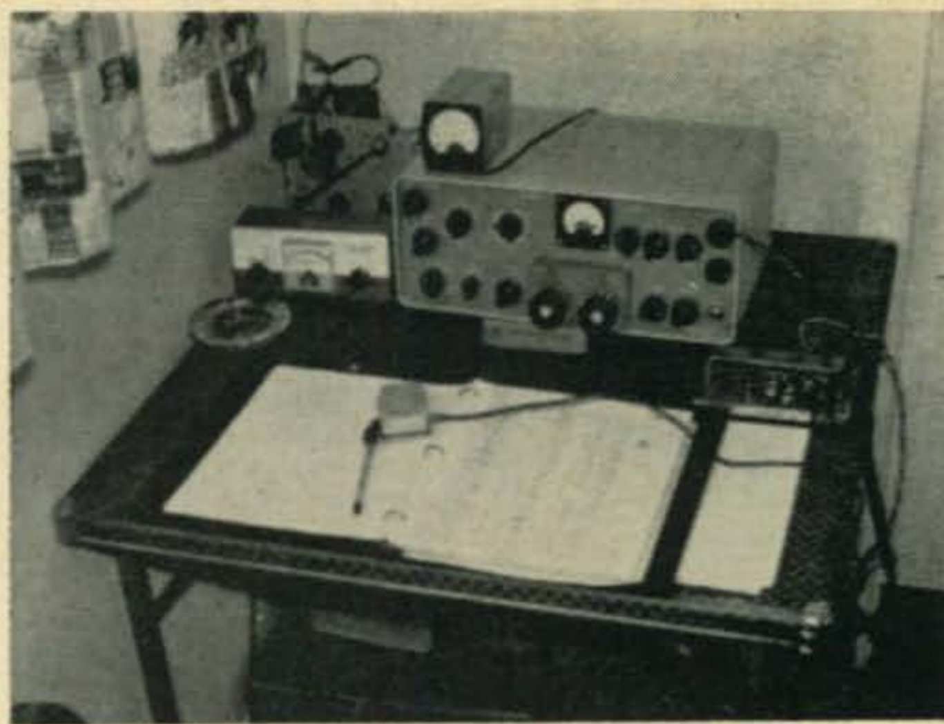
The operating position at VK2AGH/LH, l. to r. s.w.r. meter, tuning unit, a.c. voltmeter on top of the Wagner transceiver and keyer paddle to the left.
