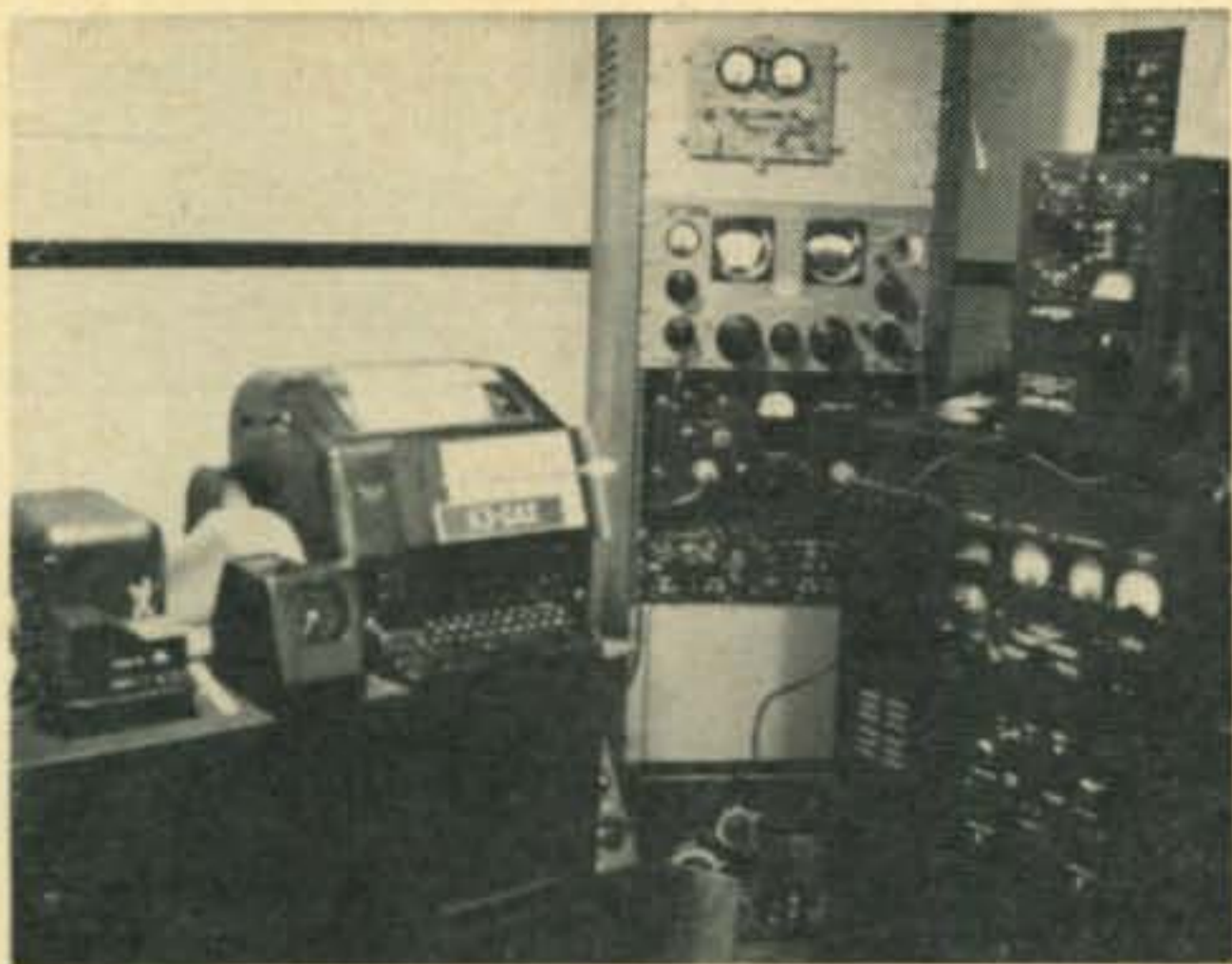
K3GAX at Glen Burnie, Maryland. The machine is a Model 19, the transmitter is a BC-610, and the receiver is a Super-Pro.
