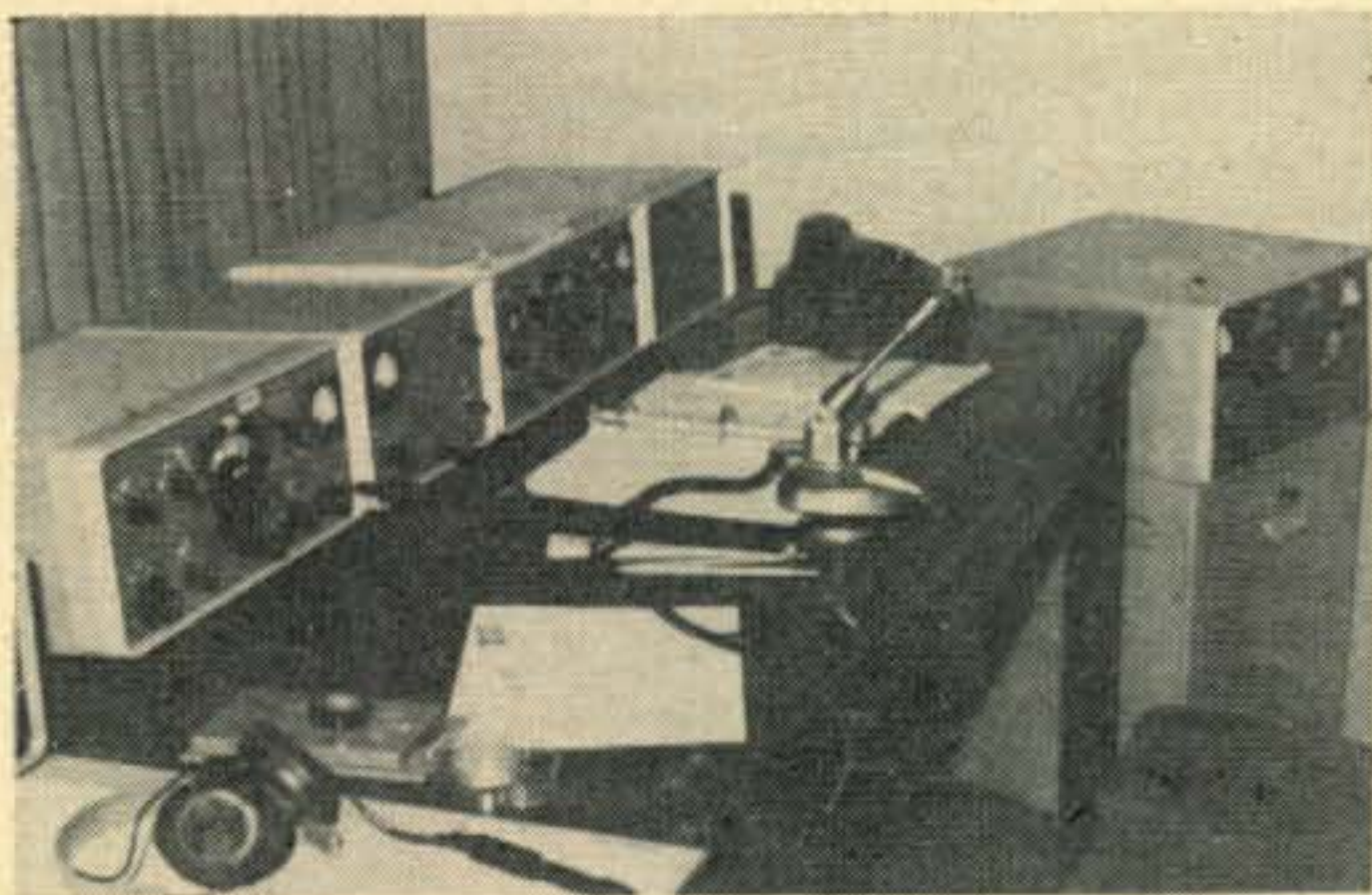
The "S-line" at W6EE on 20 meter s.s.b. On 20 meters, 14.3 mc was chosen for the Oscar prediction broadcasts. Equipment was fixed-tuned to this spot and all controls marked for easy check and adjustment.
