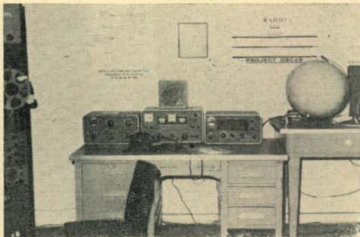
The 80 meter s.s.b. position of W6EE. Complete kilowatt s.s.b. station was loaned to Project OSCAR by Hammarlund Co. At left is rack of 145 mc tracking equipment in use at Project OSCAR HQ.
