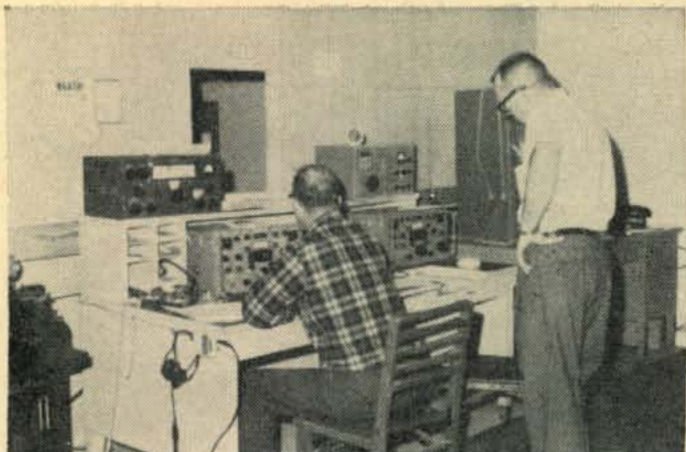
The c.w. operating position at W6EE. Separate kilowatt transmitters were used on 80, 40 and 20 meter bands. Walt Read, W6ASH, at key, with RTTY operator Bob Walton, W6CYL, as observer.
