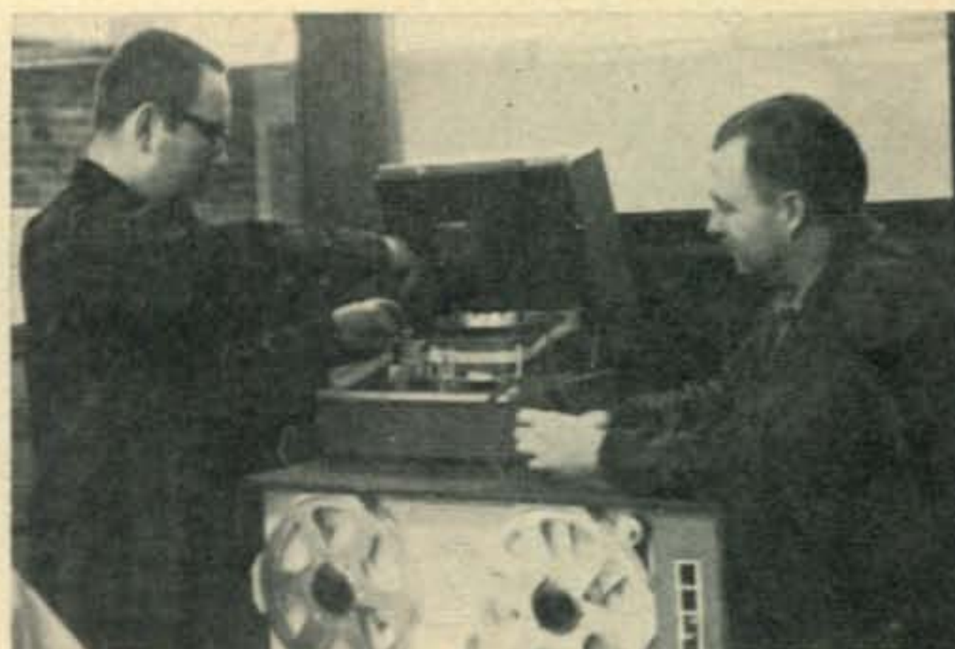
Gary McGill (no call) and Bill Walters, W6MKE (right) prepare the Foothill College 1620 computer to run weekly prediction tapes for orbital parameters of OSCAR III. Computer was adjusted to punch 5-unit RTTY tape that could be immediately transmitted on the air by W6EE.
