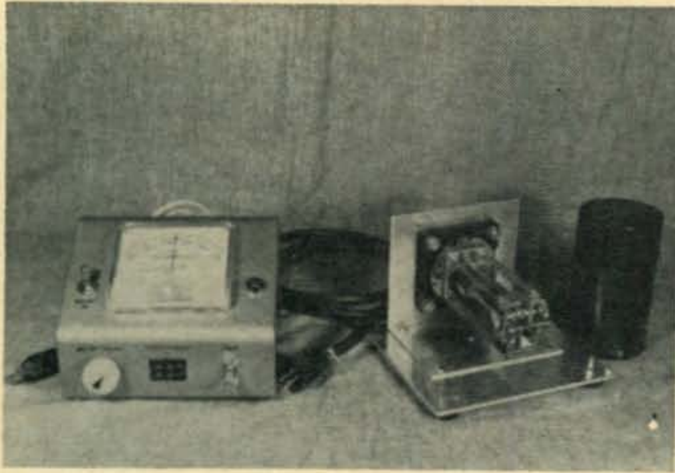
Fig. 64—Homebrewed Polar Relay Test Set is made in two sections. The relay test socket is separated from the main unit by a four foot cable.
