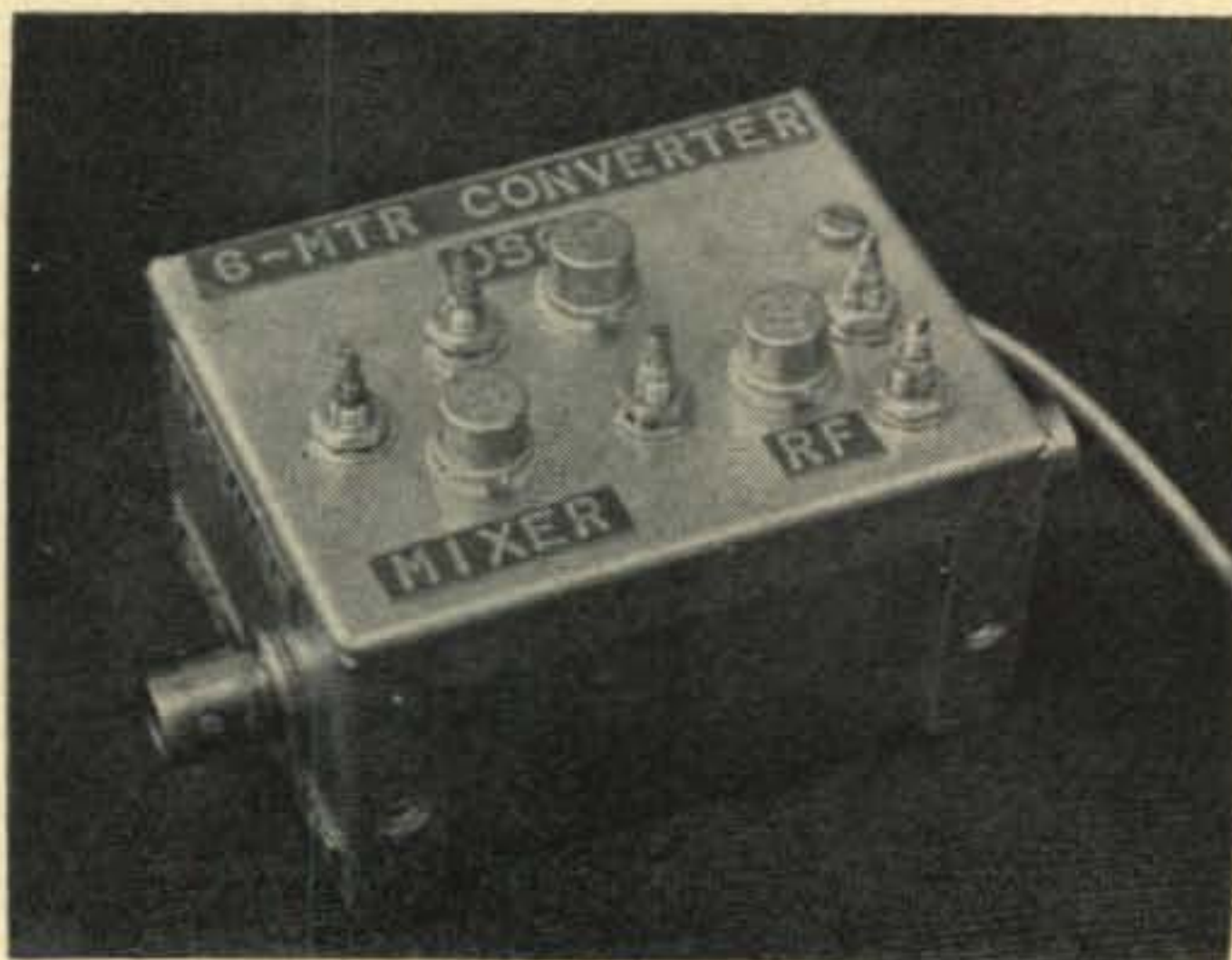
Top view of the 6 meter converter shows the location of the major components.
