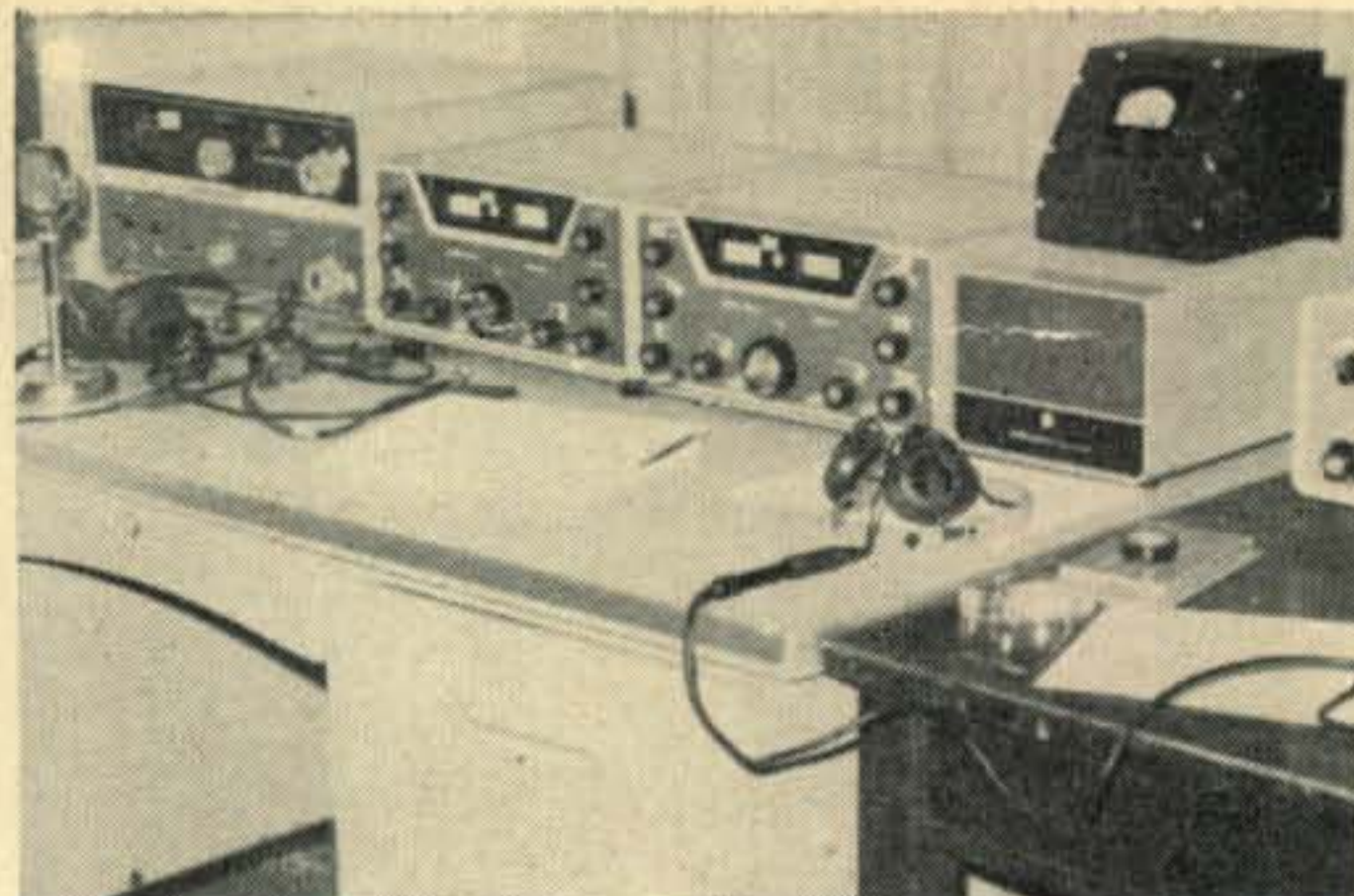
The Hallicrafters 40 meter s.s.b. position. All s.s.b. transmitters were capable of control from a single microphone and tape recorder for simultaneous prediction broadcasts on 3 bands.
