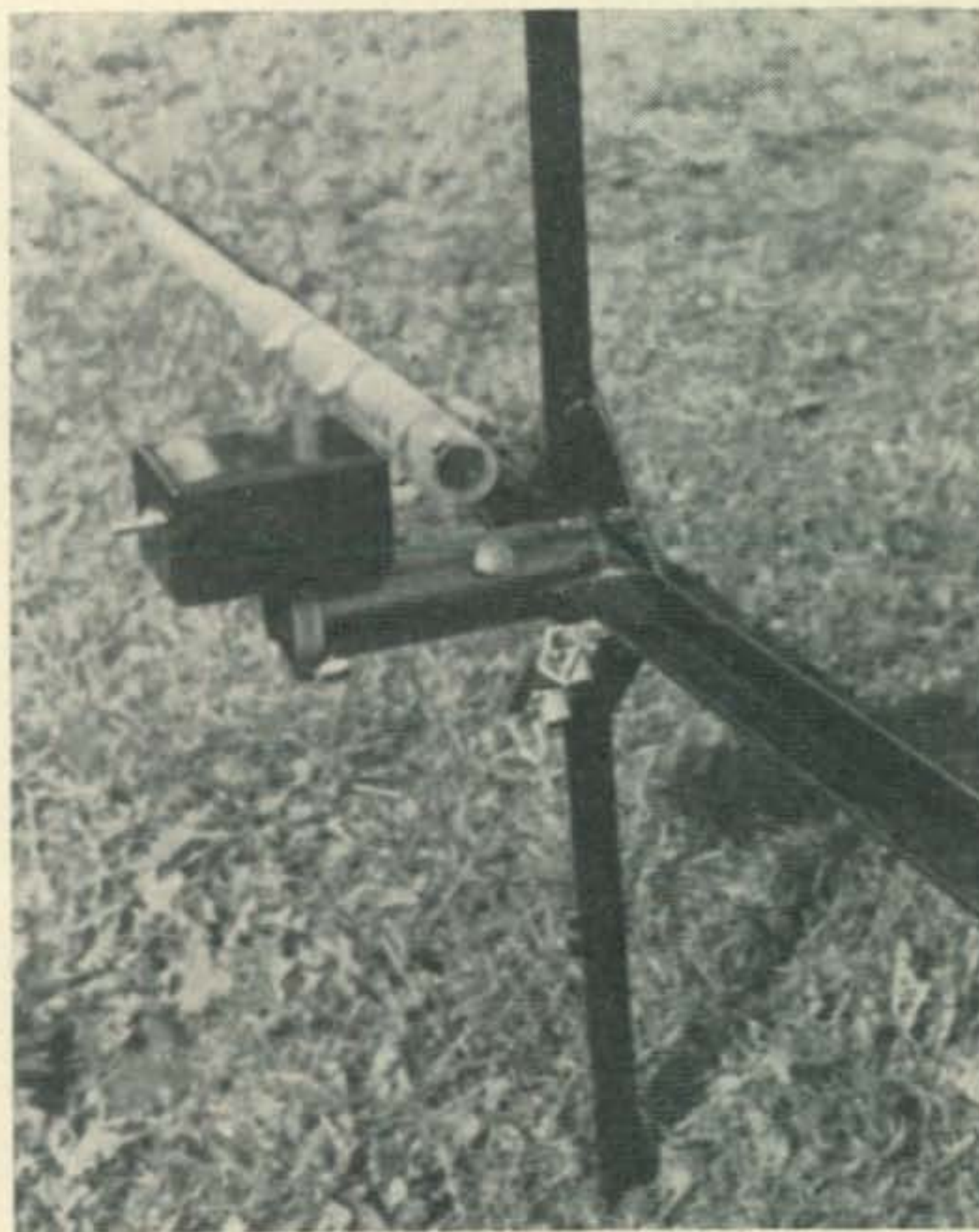
The element mounting cross. Large size industrial hose is used to insulate the elements.
