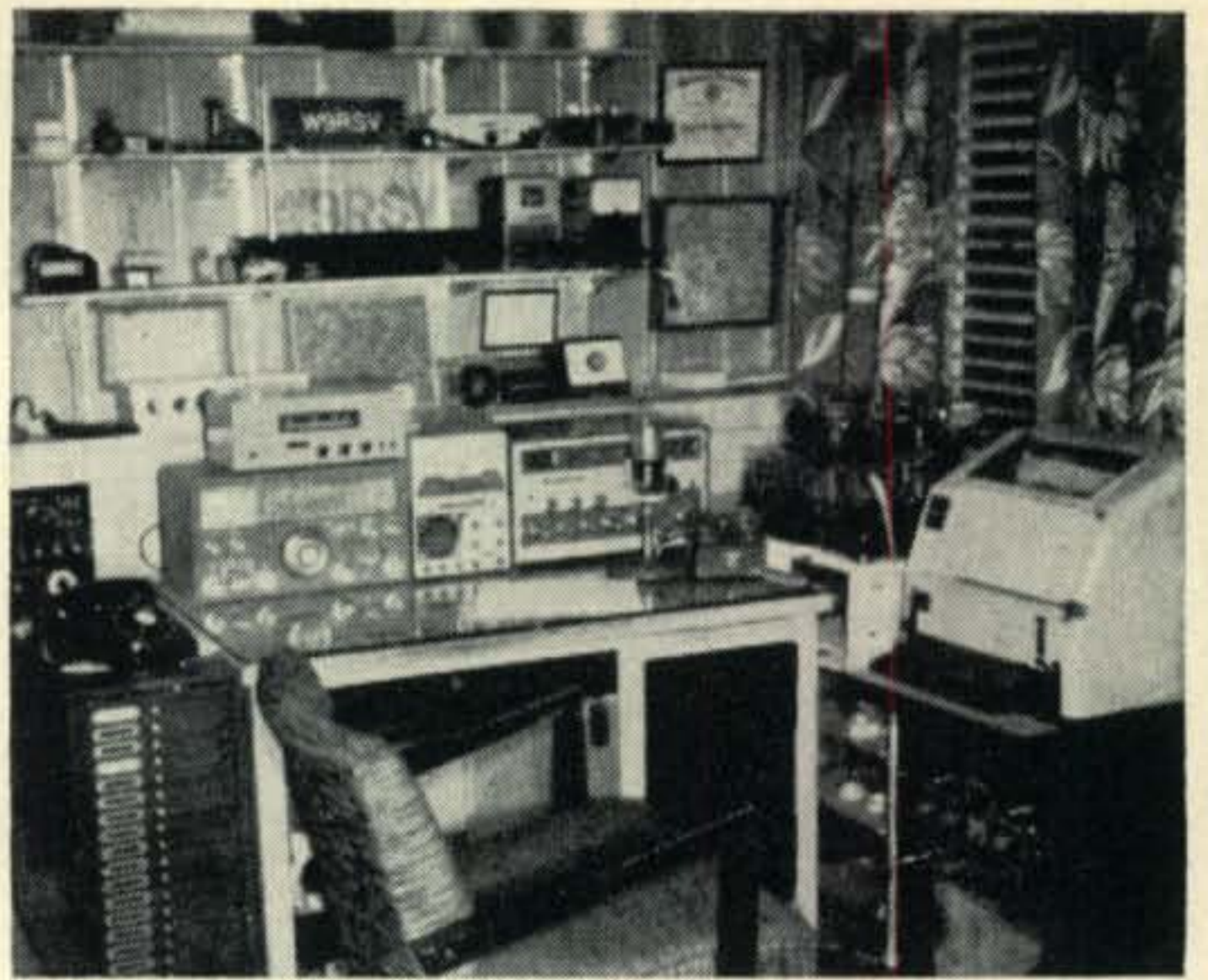
W9RSV, Chicago, Illinois, operator: Dick Kempa, transmitter: DX-100, receiver: NC-88, machines: Model 15 and an FRXD, converter (TU): Twin City TU with HO-10 'scope.
