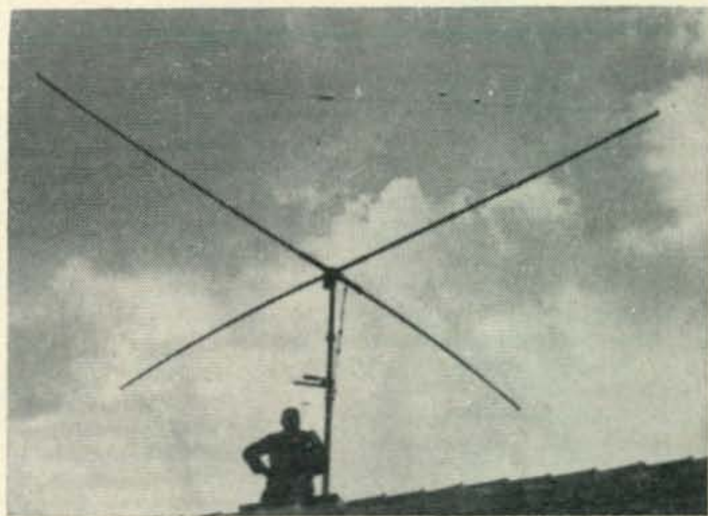
The X beam for 20 meters installed on the roof at DJØBV. The rotator is in the attic.
