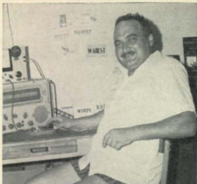
Jean, 5R8CB, at the operating position of his rig in Diego-Suarez. Jean built the rig himself. It runs 30 watts. The receiver is a much-modified vintage, 1947. The antenna is a rotary dipole.
