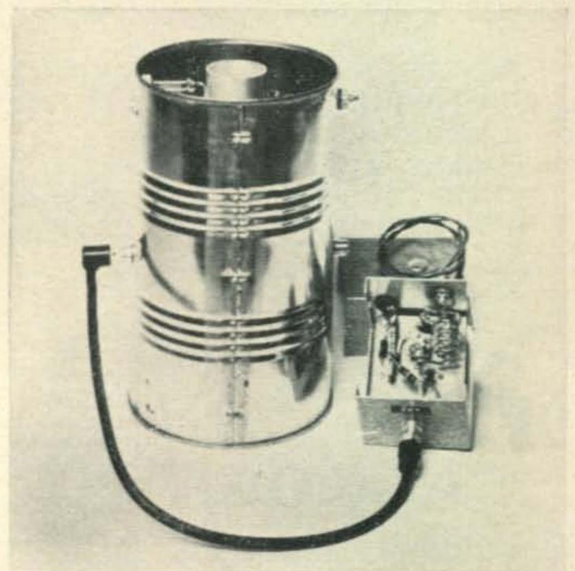
Preamp for 2 meter f.m., shown with external high-Q coaxial cavity re-entrant filter, necessary in high density areas.
