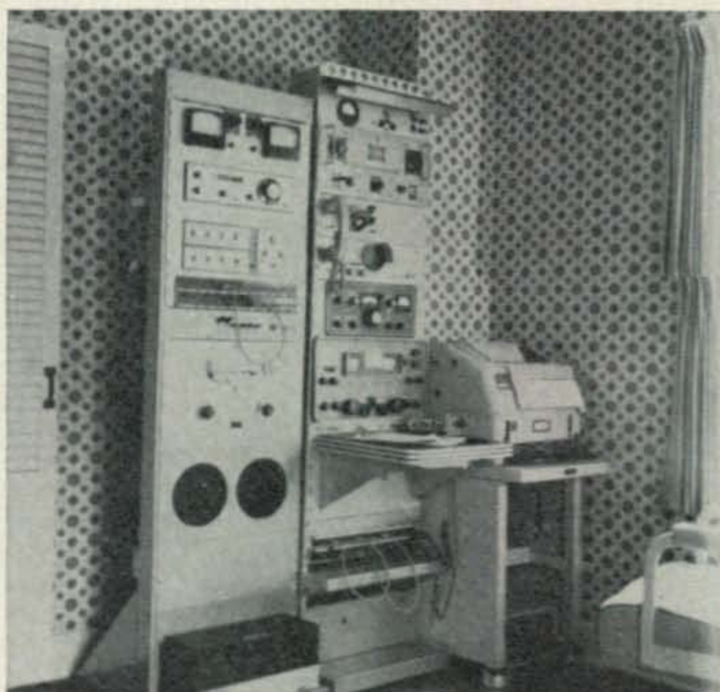
WA8GVK at Muskegon, Michigan. The right-hand rack is the RTTY station. (The left-hand rack is hi-fi audio.) The AN/FGC-1 has been re-racked in the rear, except for the patch panels. A TT-63 Regenerative Repeater, near the top, is used in conjunction with the AN/FGC-1. Below the 'scope tuning indicator is a 32S-1 and an HQ-180 receiver.
