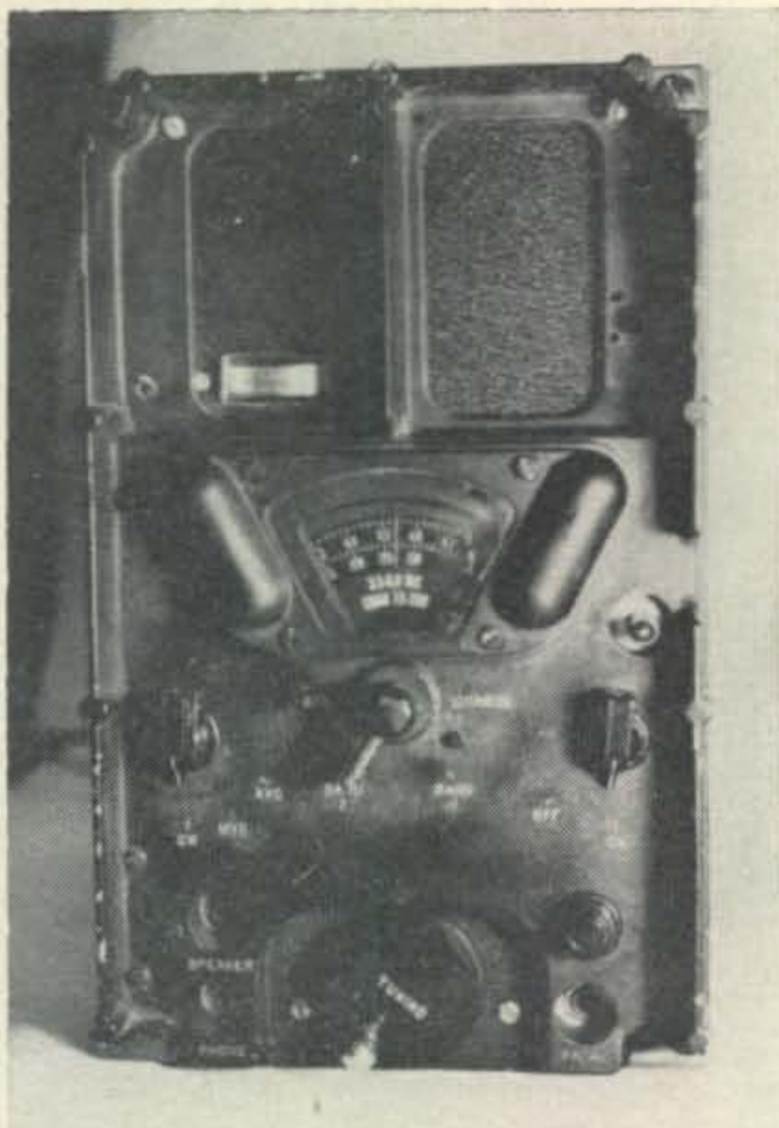
Front view of the BC-652A receiver used to cover 40 and 80 meters.
