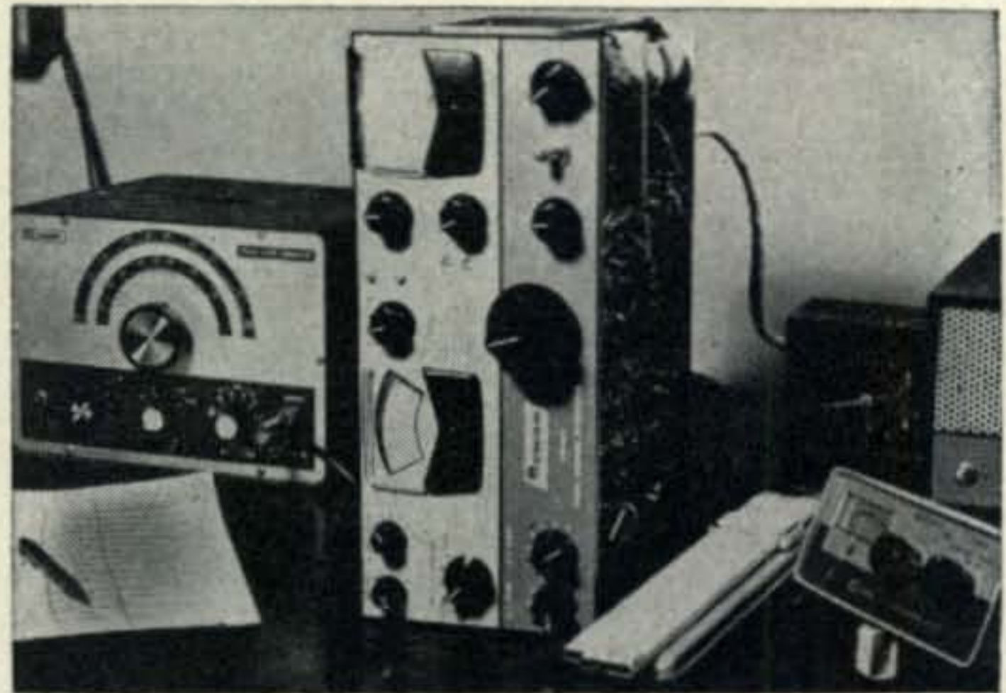
Fig. 1—To run a frequency response curve on your s.s.b. transceiver all it takes is an audio generator and s.w.r. meter with power output measurement facilities. It is not necessary to take the top and bottom off the transceiver. They were removed here to make adjustments.
