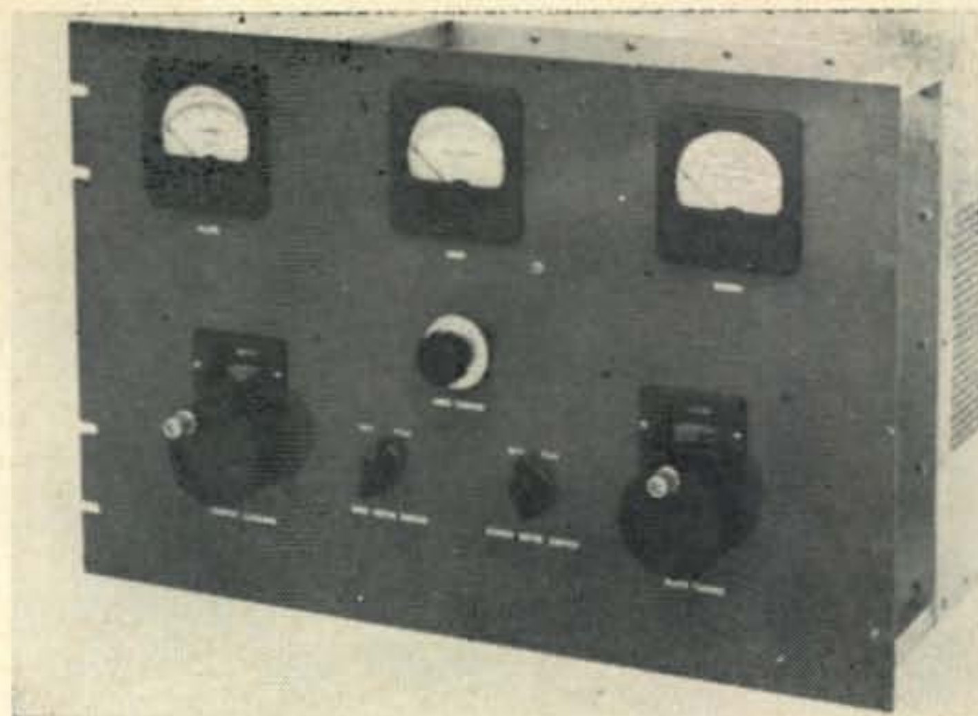
Fig. 8—Front view of a compact two kilowatt p.e.p. linear amplifier for the v.h.f. man. This high power 144 mc linear is suitable for s.s.b., a.m., f.m. or c.w. operation, requiring less than 10 watts drive power to reach the maximum legal amateur power level. The amplifier is mounted behind a standard 12 1/4" relay rack panel. Across the top of the panel (l. to r.) are the plate, grid and screen milliameters, with the grid tuning capacitor ( C_2 ) centered below. At lower left and right are the counter dials for the OUTPUT LOADING control and PLATE TUNING ( C_3 ). Between the counter dials are the grid and screen meter reversing switches. The amplifier enclosure is spaced behind the panel by sections of rectangular aluminum rod and the 4CX1000K mounts in a horizontal position within the enclosure. At the right end of the enclosure are the ventilation holes above the anode of the tube.
