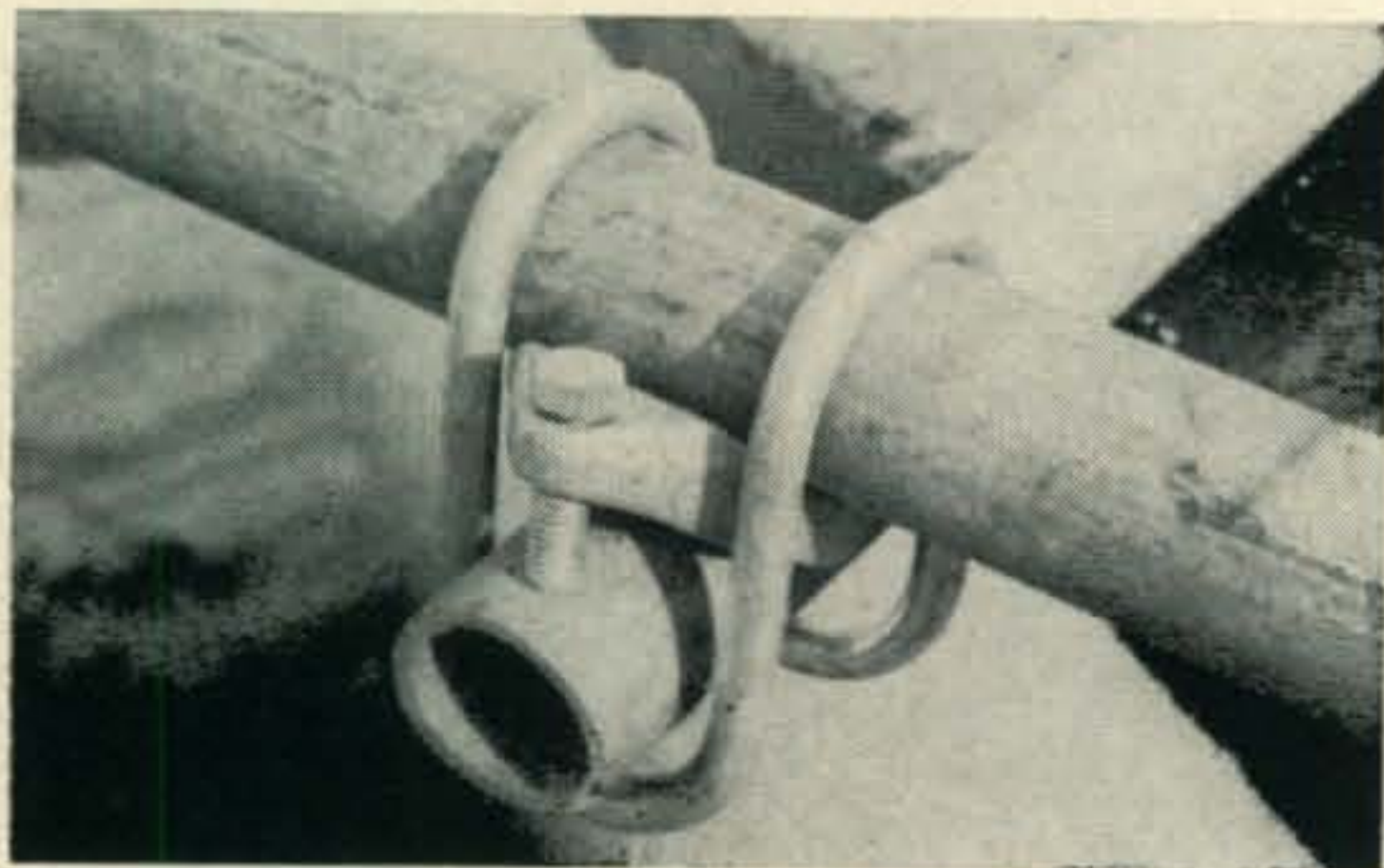
View of two interlocked members of the array using a one bolt adjustment Rota-Lock made by the Up-Right Scaffolds, 1013 Pardes Street, Berkeley, California.
