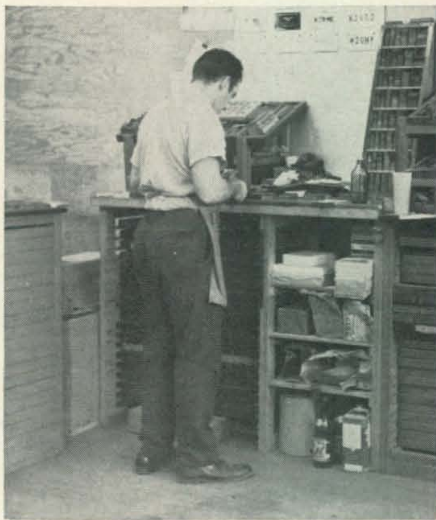
Isaac Luttrell puts together the type for a QSL card. Above his work area is a board displaying some of his designs. The rack of little wooden blocks on the right contains spacers to fill out the QSL frame.
