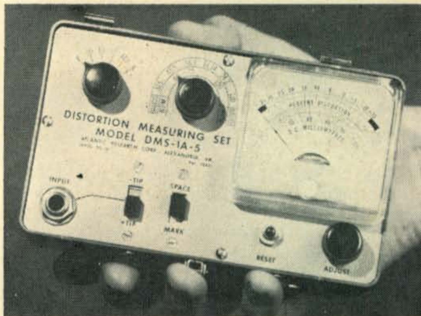
Fig. 111—The model DMS-1A-5, an improved distortion measuring set with direct meter calibration.
