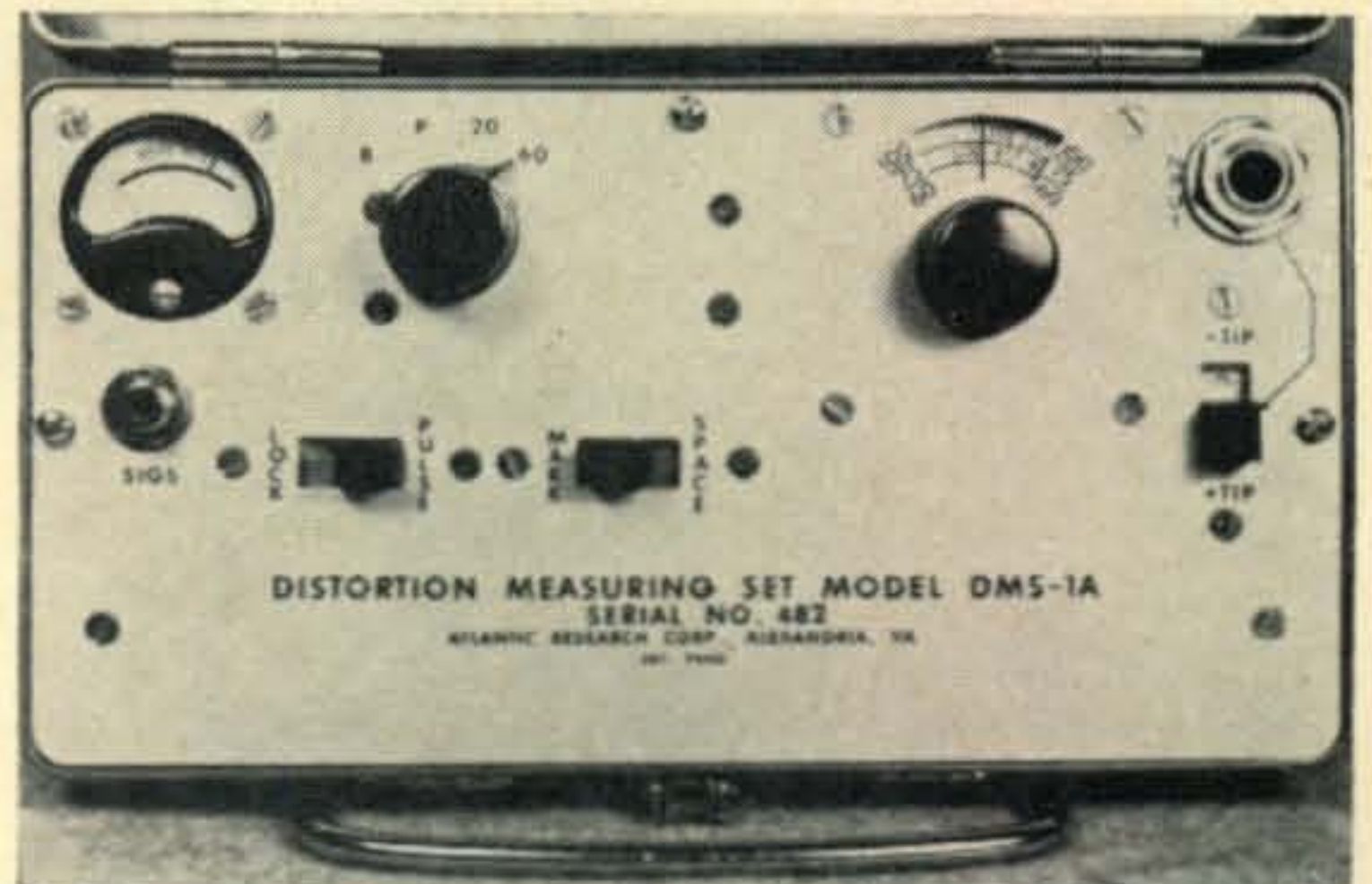
Fig. 107—Close-up view of the DMS-1A Distortion Measuring Set showing control locations and designations.
