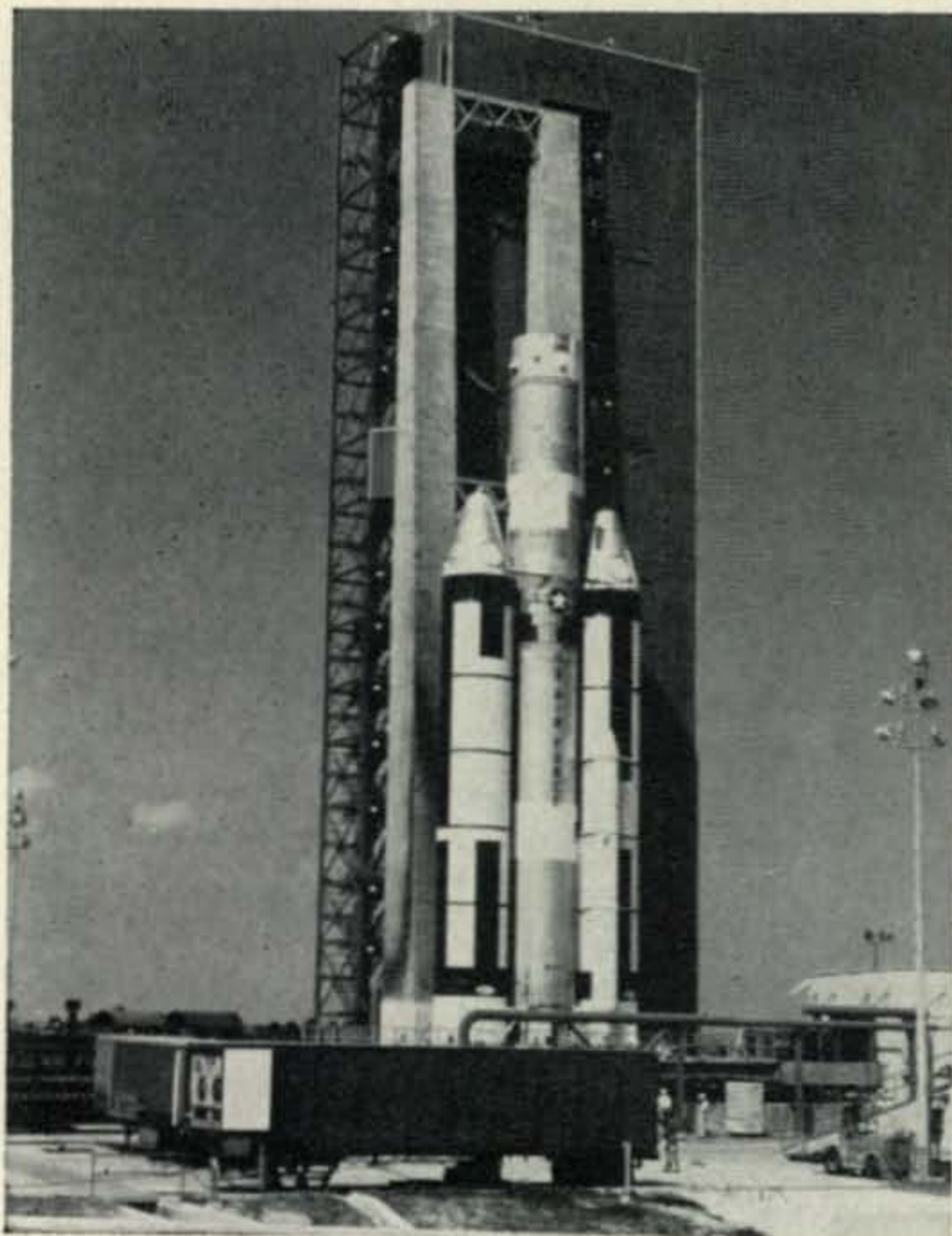
The triple-barreled Titan III-C booster being moved to Pad 41 at Cape Kennedy for a December 21 launch. The booster stands as high as a 12-story building. The "transtage", or third-stage of the center portion of the Titan III-C has not yet been installed. The OSCAR IV satellite, and the other payloads carried into space by Titan III-C were contained in the transtage. (U.S. Air Force Photo).
