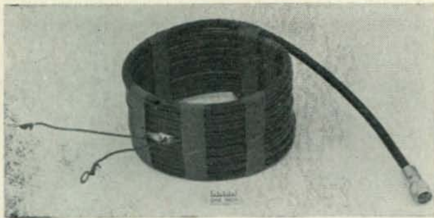
Fig. 4—A coaxial balun made by WA6JSA. A single length of coaxial cable was wound on a suitable form and fixed in position with vinyl tape. The balanced connections at the center of the winding are made by short lengths of #12 wire, and the "top" end of the coil has a PL-259A plug affixed to it for connection to the station transmission line.
