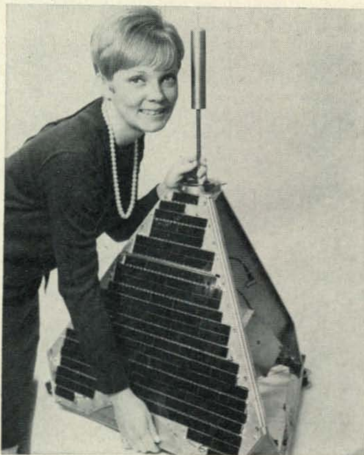
OSCAR IV gets a fond farewell embrace from Mrs. Kathleen Licari at the TRW Amateur Radio Club, prior to the satellite's shipment to Cape Kennedy for launch. The 432 mc transmitting antenna is extended at the top of the satellite. Solar cells cover all surfaces of the satellite so that it can receive energy from the sun in any position. (Project OSCAR Photo).
