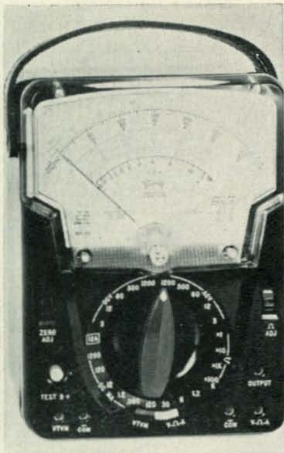
A combination v.o.m. and battery-operated v.t.v.m. The latter measures only voltages up to 120 v.d.c.
