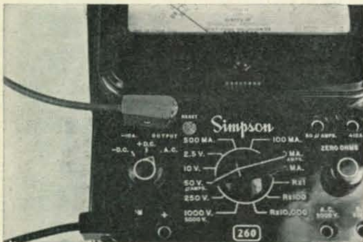
The OUTPUT position of the v.o.m. is used to measure a.c. impressed upon d.c.
