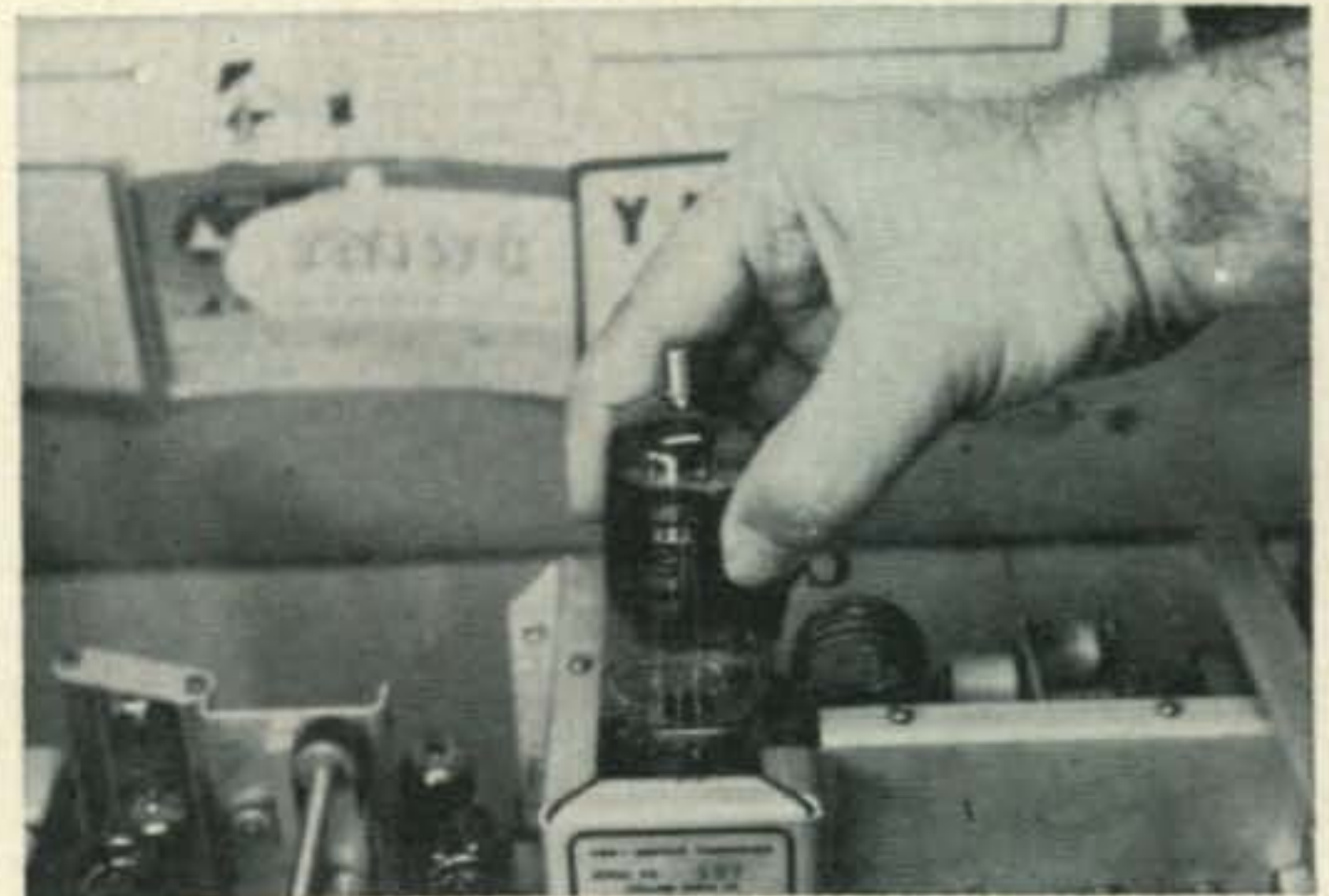
After the modification, install the 6HF5's, drive twice as hard and get twice the power.
