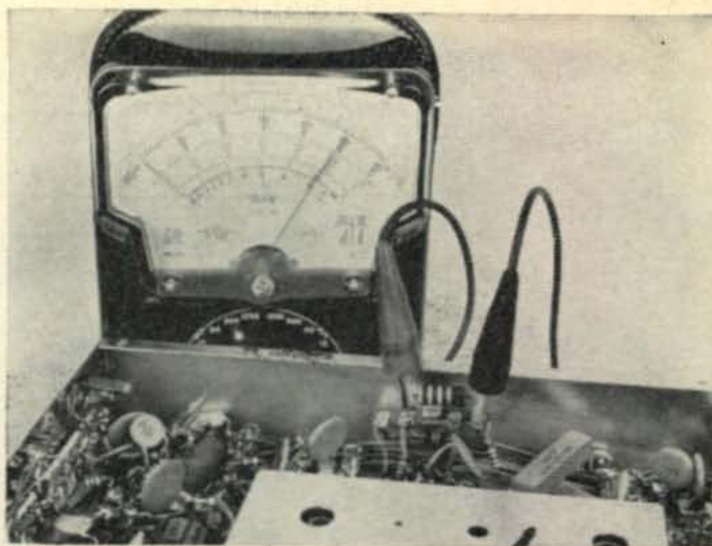
Measuring current by the indirect method.
