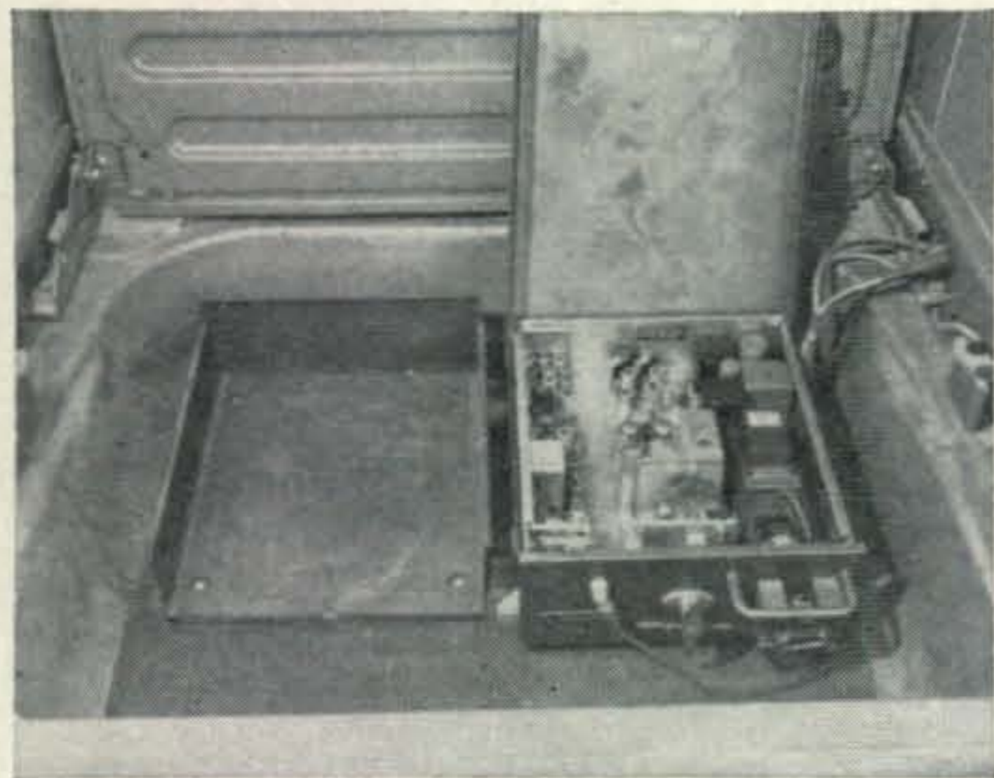
Mobile installation in the rear luggage well of a Chevrolet 1965 station wagon. Shown is the Motorola-80D for 2 meters. On the left is the empty bottom half of another split case for a future 80D for 6 meters.
