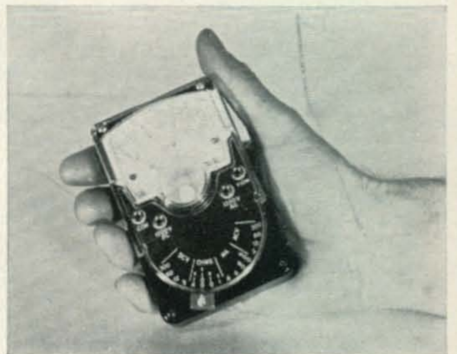
A pocket-size v.o.m. that has a 20,000 ohms/volt d.c. sensitivity, 5,000 ohms/volt a.c.
