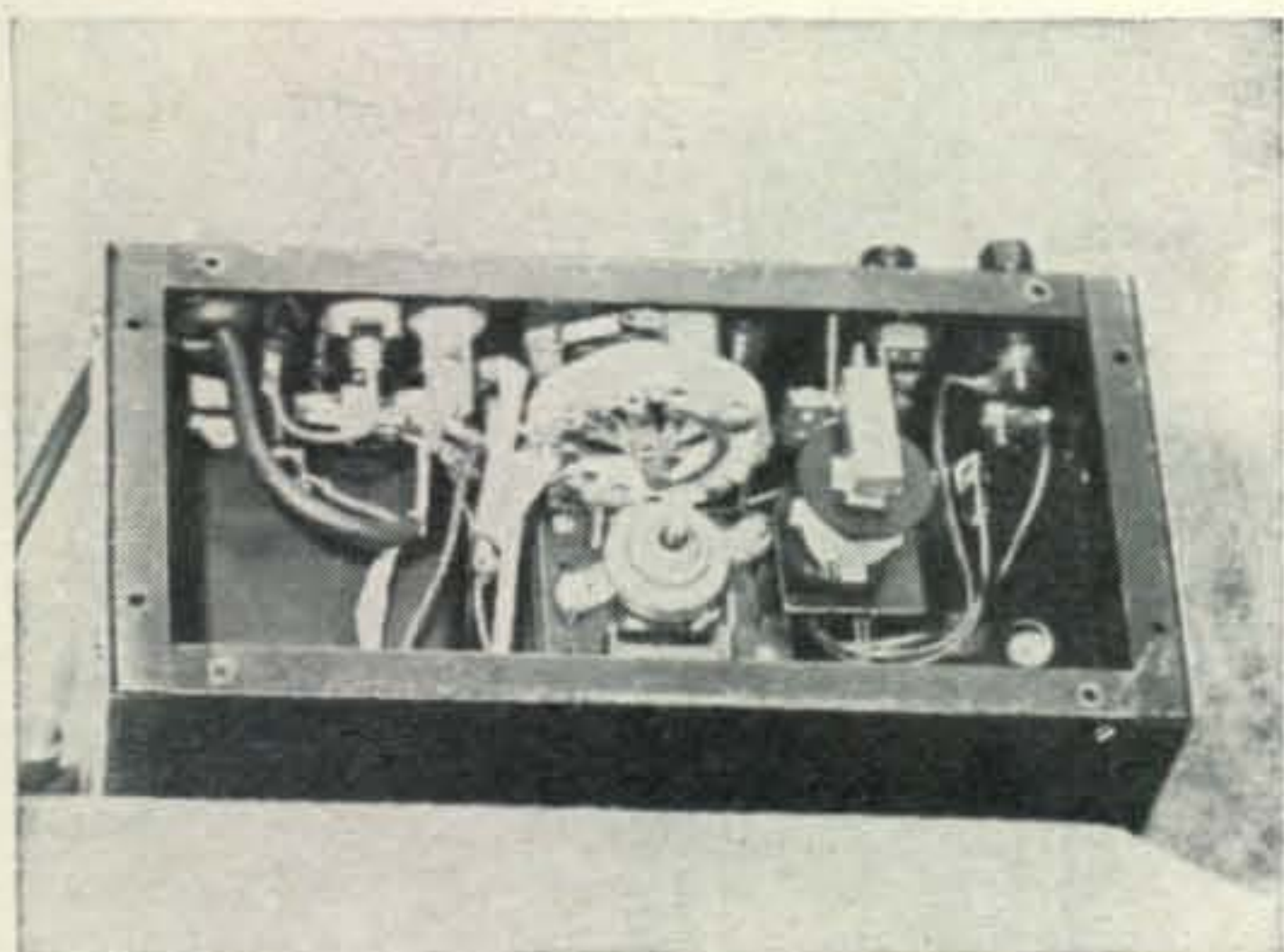
The underside of the chassis is dominated by the tap switch and the blower motor.
