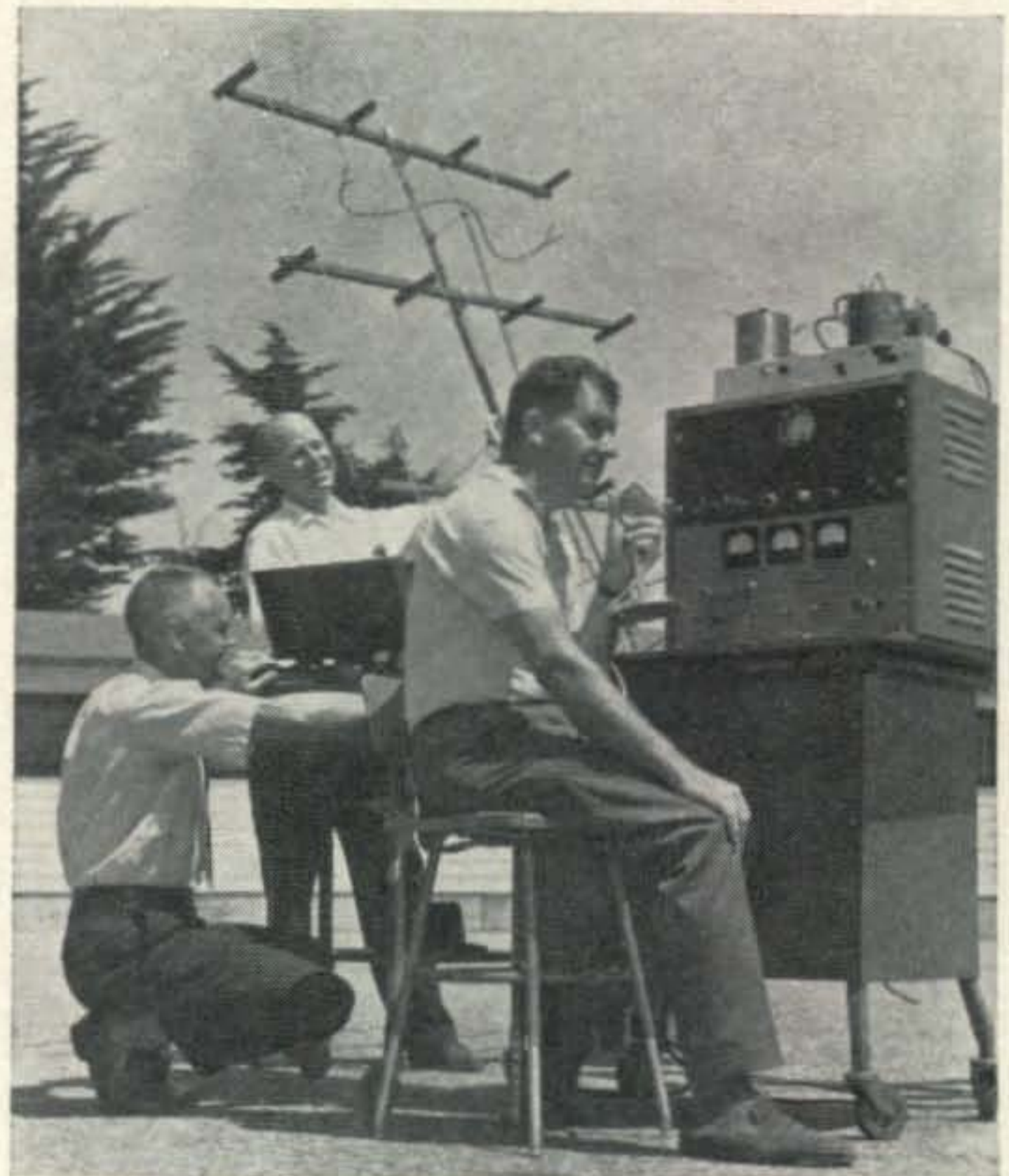
Outdoor moonbounce station, California style. In center is W6YK (see letter, April column); right with mike is K1LSY/6; at left, kneeling, WA6VTY. Antenna shown held by W6YK is a 32-element collinear extended made of aluminum clothesline for 432 mc. Gain measured at 18.5 db over tuned dipole.
