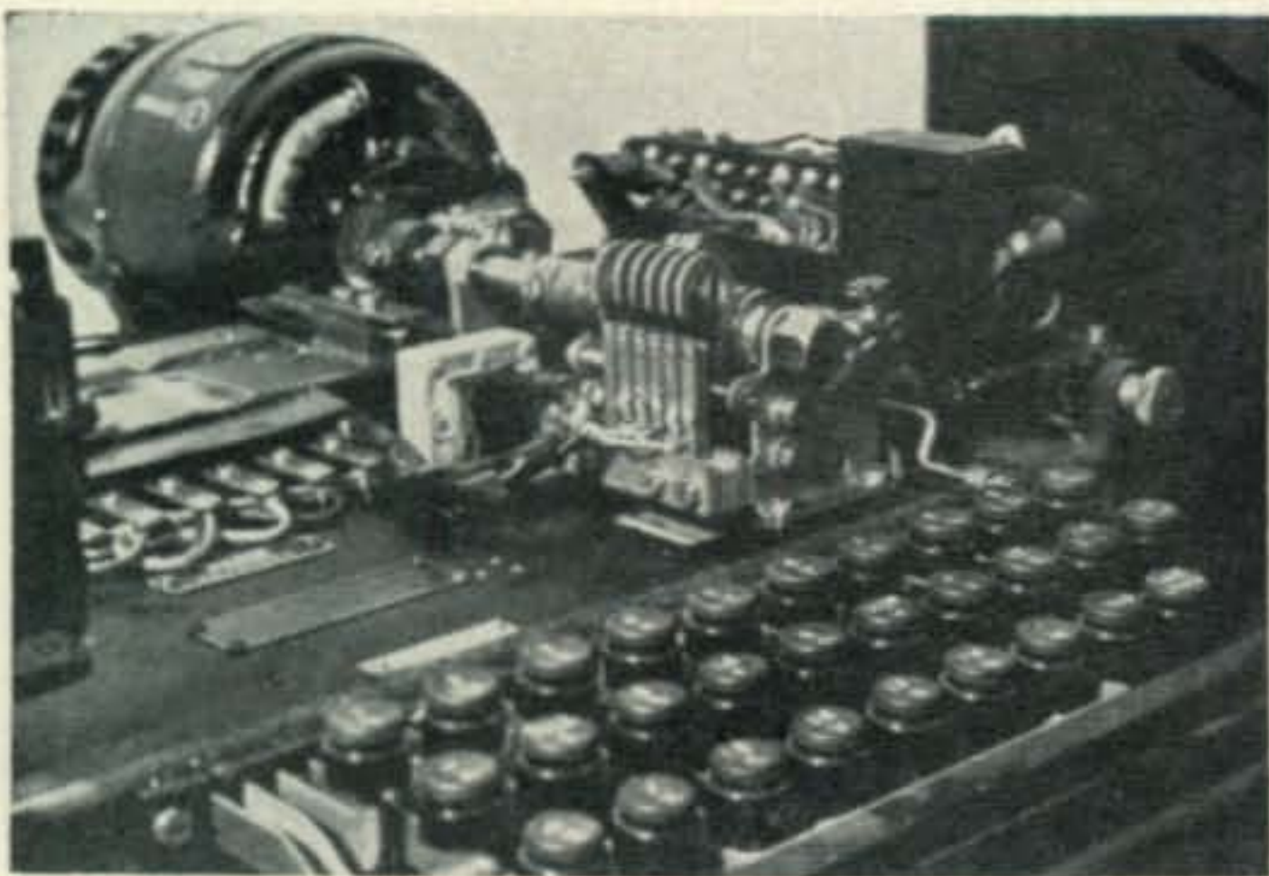
Solenoid mounting on Teleprinter keyboard base plus wiring of teletype keyboard transmitter contacts.
