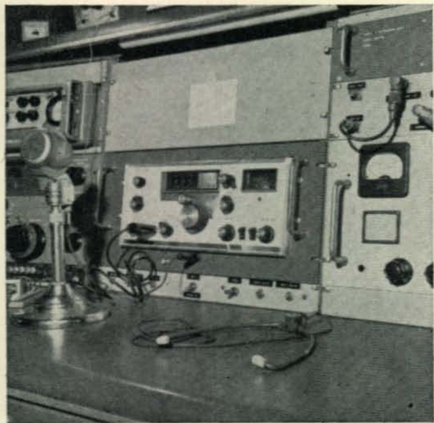
Fig. 1—The NCX-5 mounted in the rack. The connectors directly under the unit are extended from the rear of the transceiver for the key and headphones.
