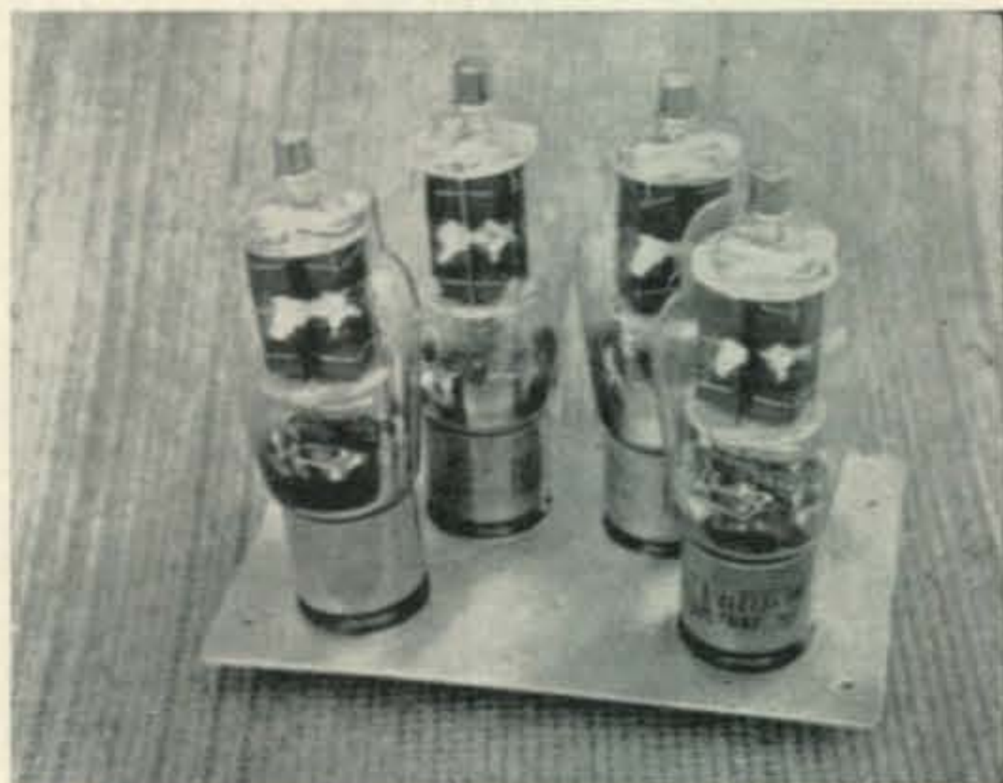
Shown above is a sub chassis with four 837 tubes mounted. This is all the mechanical work needed to adapt the linear to different tubes.
