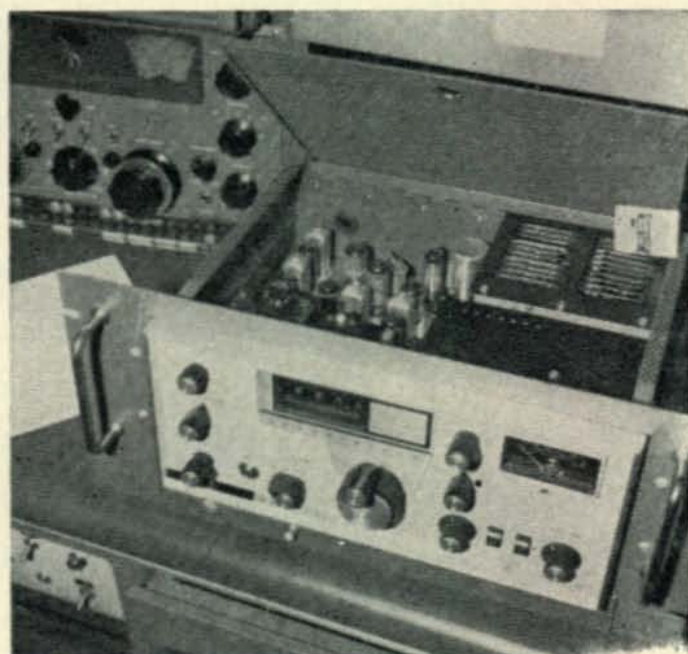
Fig. 4—View of the transceiver with the rack extended and the lid raised for adjustments.
