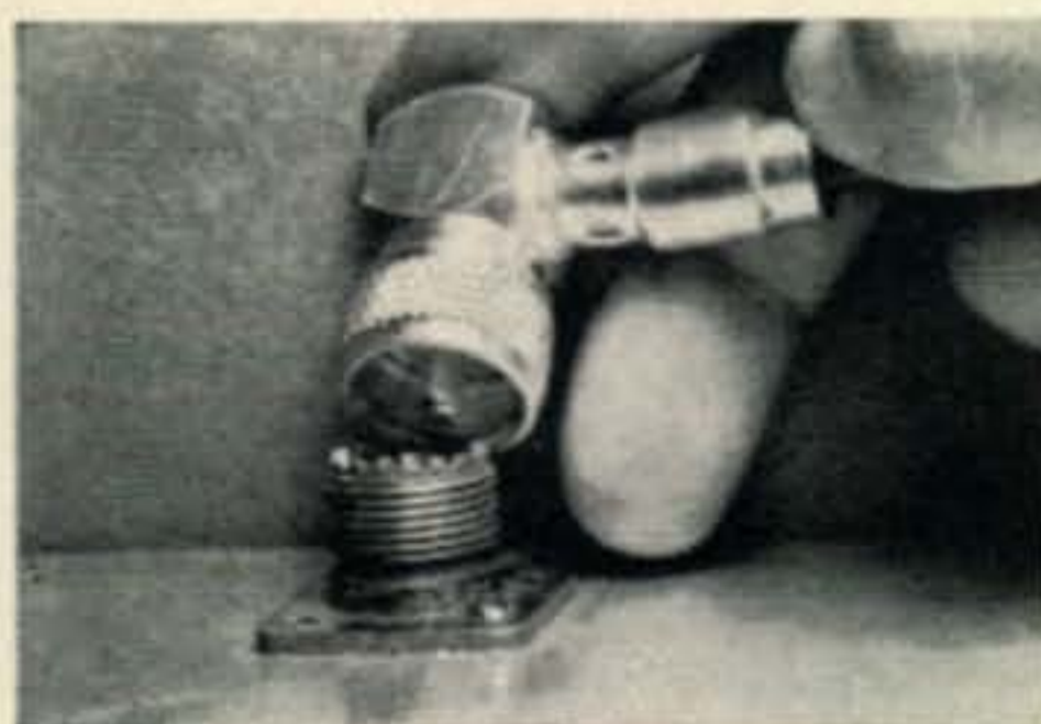
Fig. 4—A handy connector unknown to most amateurs, this right-angle u.h.f. plug makes it easy to connect cables to chassis connectors on the back of low- and medium-power equipment. A right-angle plug is shown as it is connected to the back of an antenna tuner.
