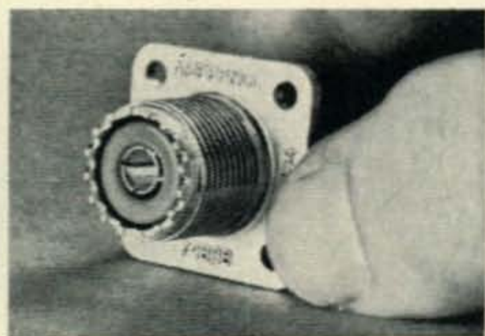
Fig. 5—The most common type of u.h.f. chassis connector, the SO-239 is a mica-filled, bakelite-insulated model with excellent environment-resisting characteristics. Like all UHF-type connectors, it is made of silver plated brass. These two metals provide a rugged combination.
