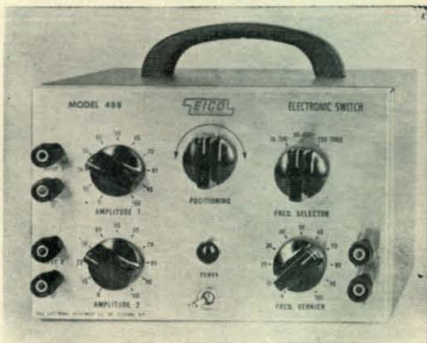
An electronic switch that enables superimposed or dual displays to be obtained on the oscilloscope.
