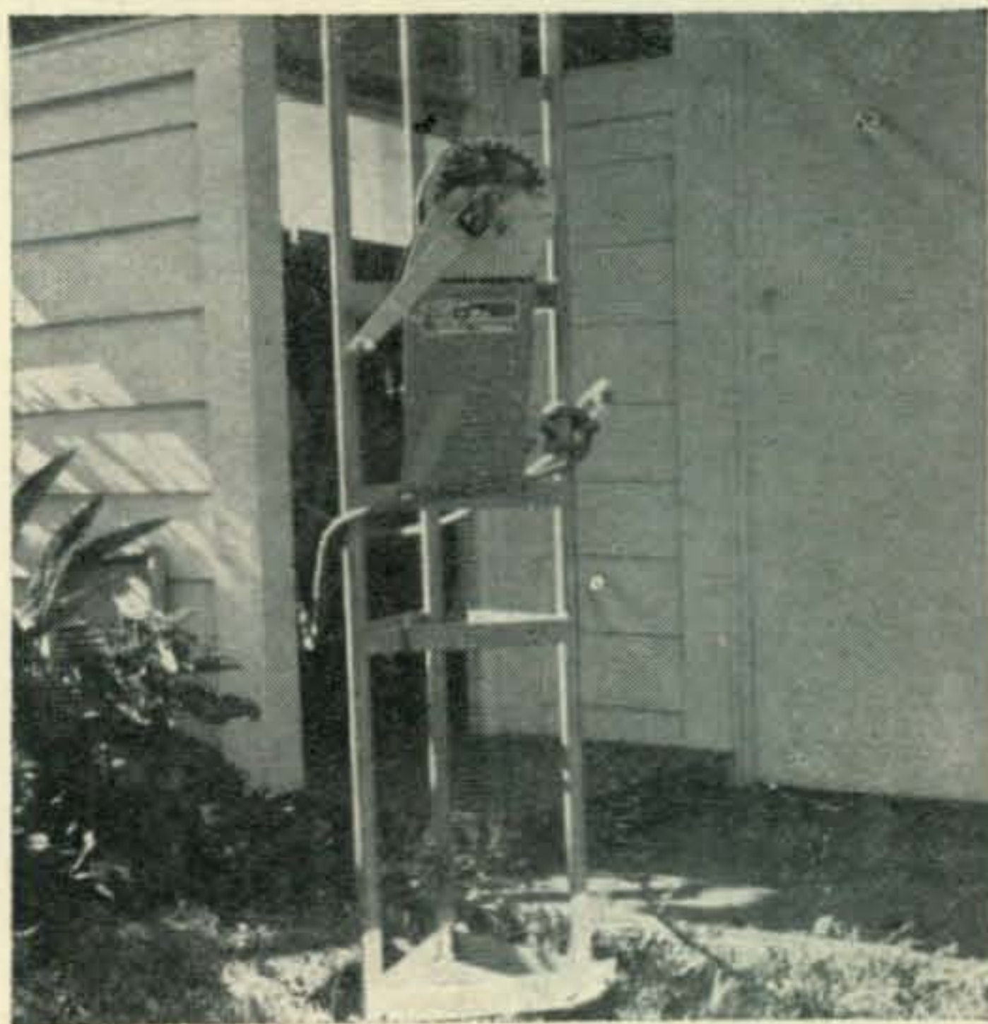
Tower rests on a "Greased Peg" and turns easily.
