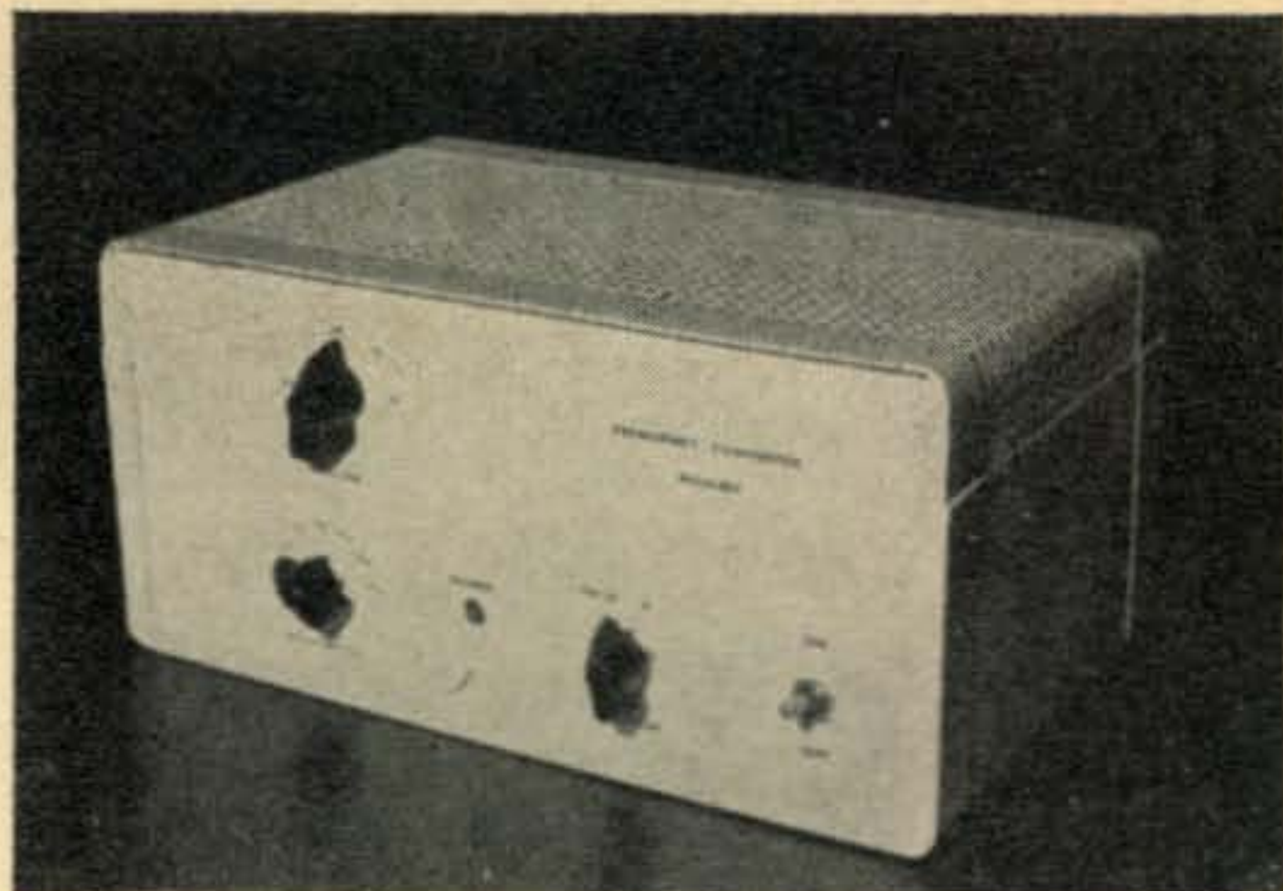
Front view of the converter. The 6 meter unit that shares the enclosure is on the right and the switch next to the ON-OFF toggle shifts power to either converter.
