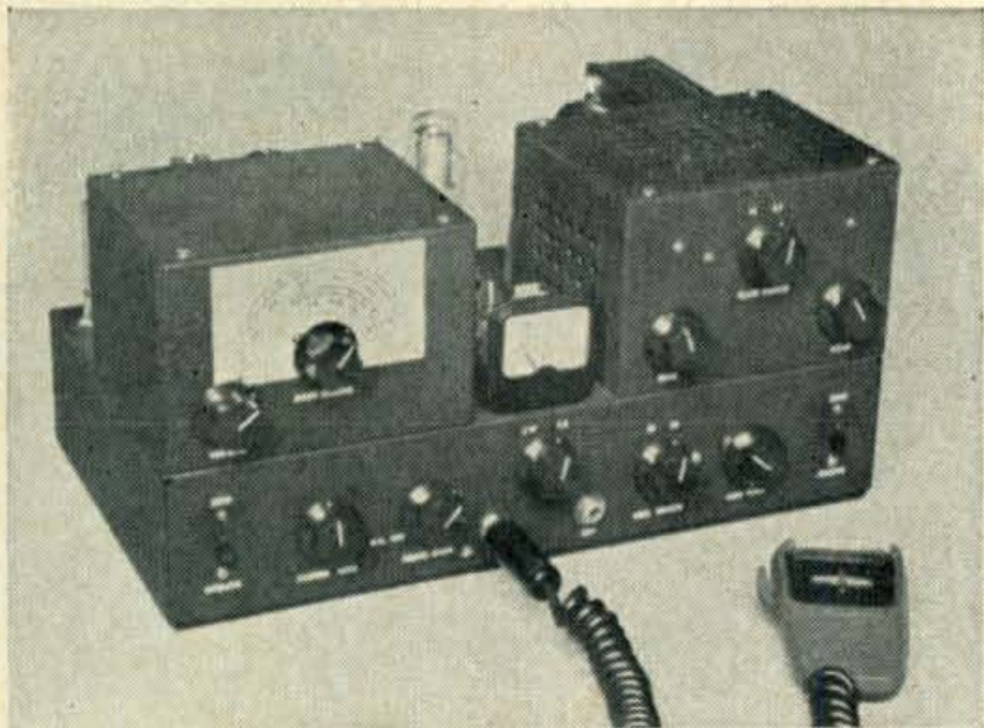
Fig. 1—End result of a three step construction project, the CQ-150 Mark II is a 5 tube s.s.b./c.w. transmitter that features a self-contained power supply, stable v.f.o., push-to-talk relay, bandswitch for 80 or 20 meters, 150 watts p.e.p. input on upper or lower sideband, 150 watts c.w. input.
