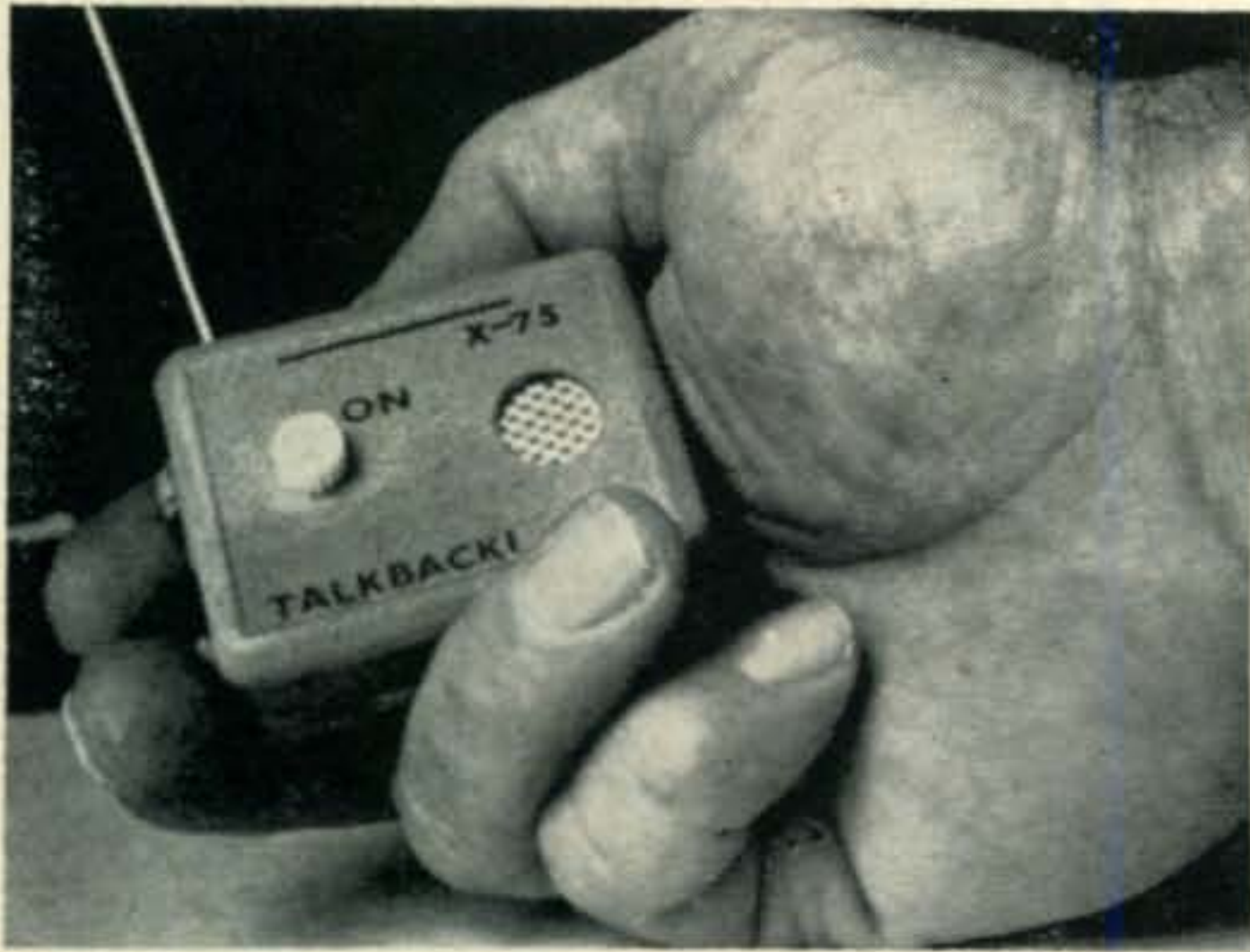
Fig. 8—A typical wireless bug built for operation in the f.m. broadcast band.
