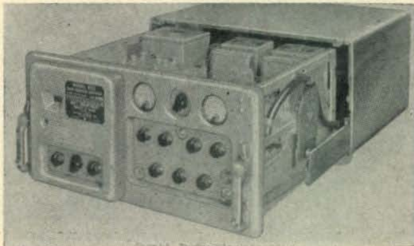
The RDZ receiver, shown here partially withdrawn from its spray-proof cabinet in a u.h.f. unit covering 200-400 mc. The tuning section which can be modified for tuneable operation is behind the aluminum casting which protrudes from the left side of the set. Circuit alterations must be made in the compartment which is reached from access panels beneath the set. A tuning knob can be added to the front panel for tuneable operation.
