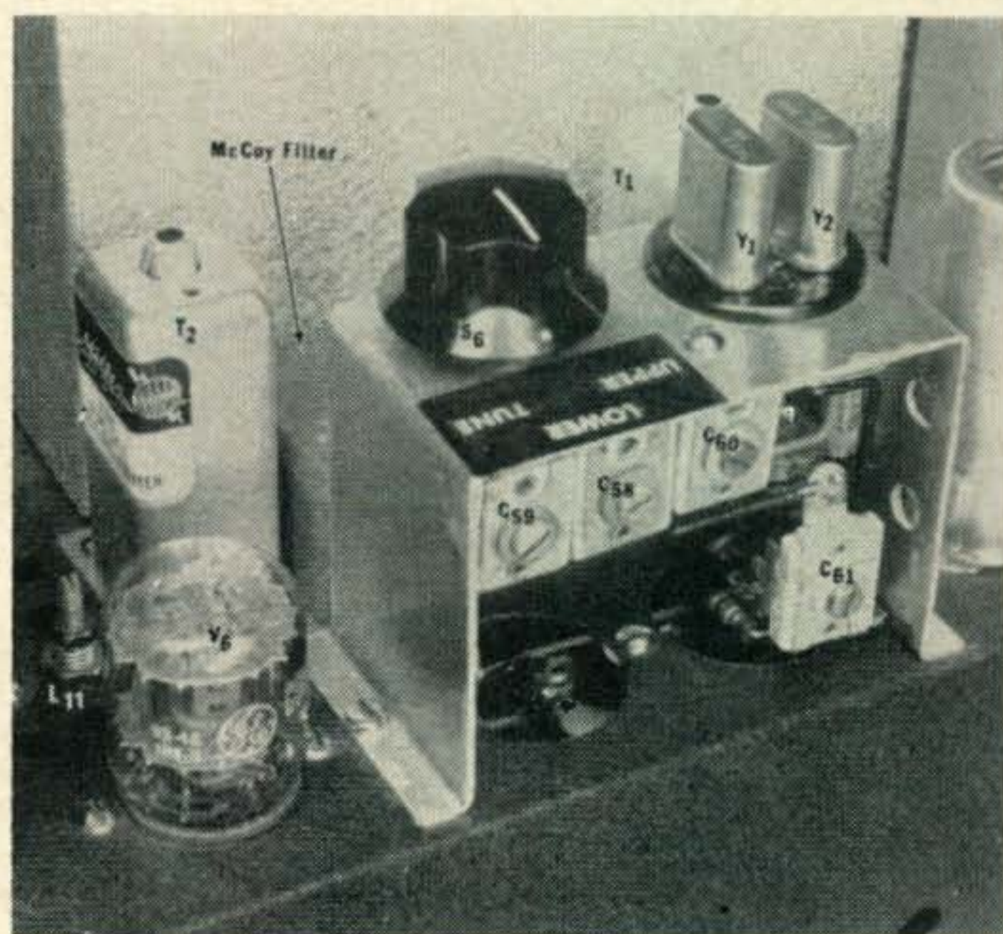
Fig. 26—Rear view of the transmitter showing the bracket that mounts the carrier oscillator components. The McCoy 9 mc filter is located between the rear of the v.f.o. compartment and the U-bracket.
