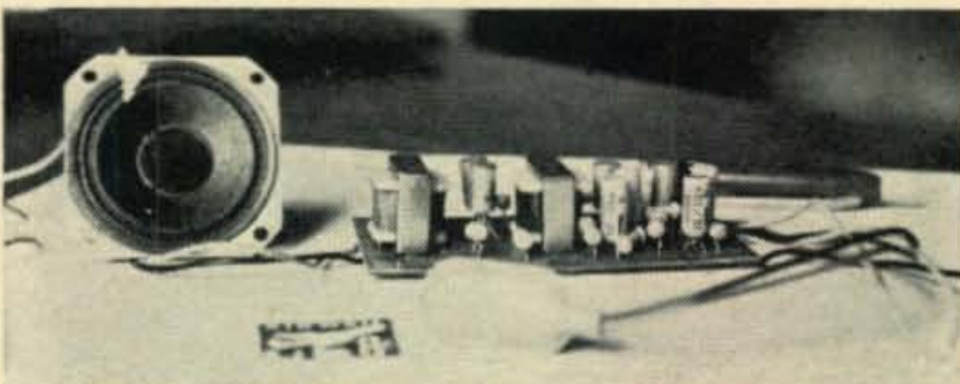
Fig. 6—A transistorized a.f. amp that can be used for listening in. It can use either a tiny mike or the small one inch loudspeaker as a pick up device.
