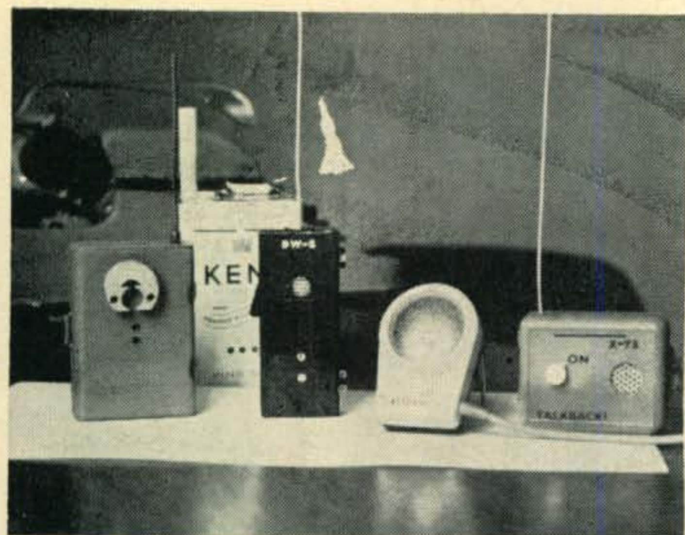
Fig. 1—Sets constructed by the author to show how wireless bugs can be made in different sizes and shapes. Note the magnet on the bug at the far left. This is used to fasten it behind a radiator. The cigarette package also contains a bug. Note the relative size of the bugs as compared to a recording mike, second from the right.
