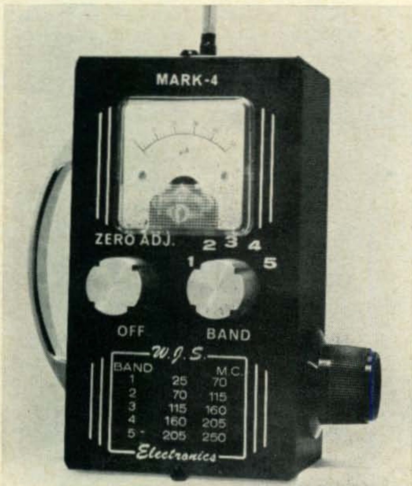
Fig. 9—A professional bug locator made by the W.J.S. Electronics Co. of Hollywood, California. This detector covers from 25 to 250 mc in 5 bands.
