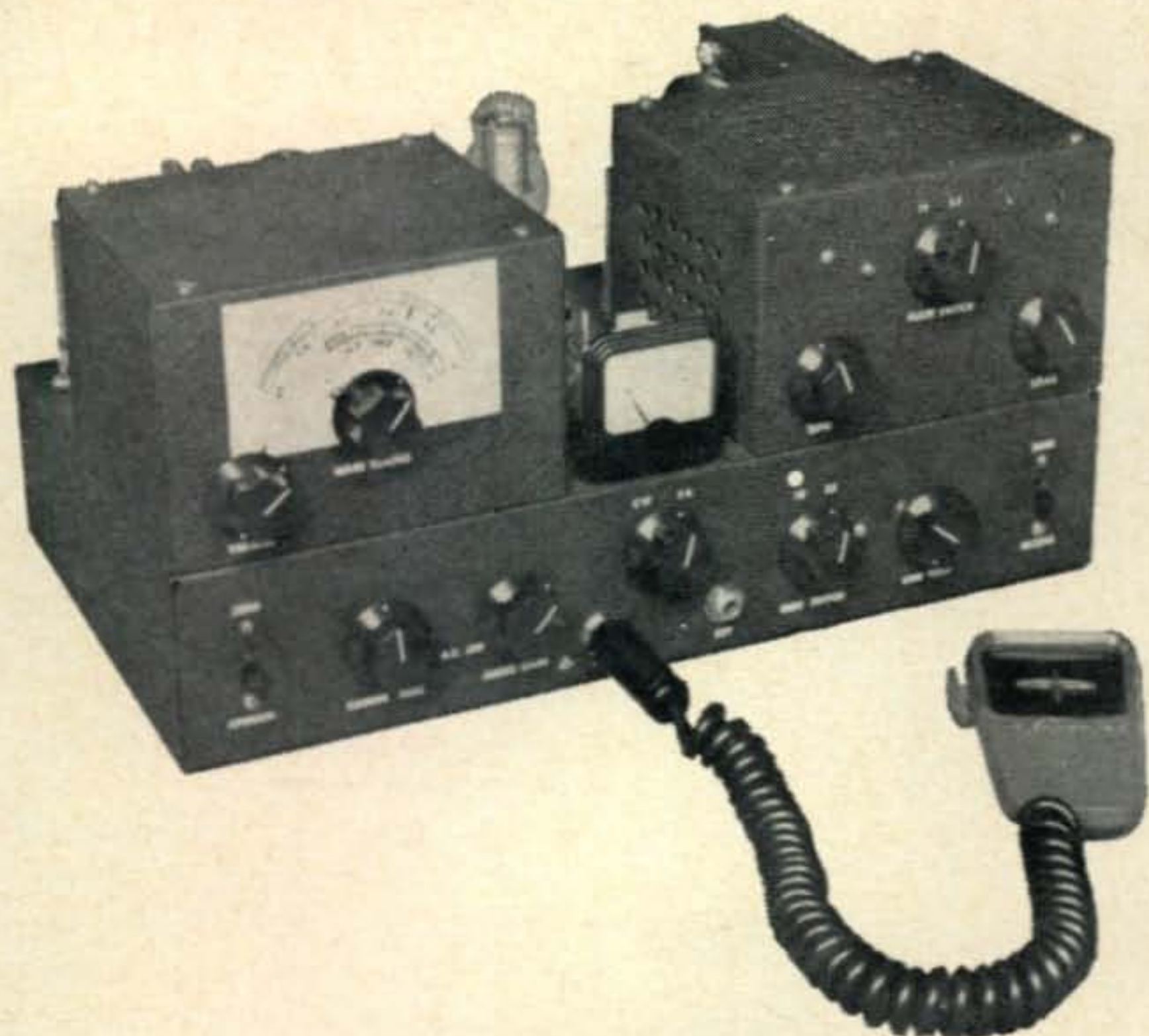
Fig. 19—The front view of the CQ-150 Mark II. The rig is capable of s.s.b. or c.w. operation on 20 or 80 meters.
