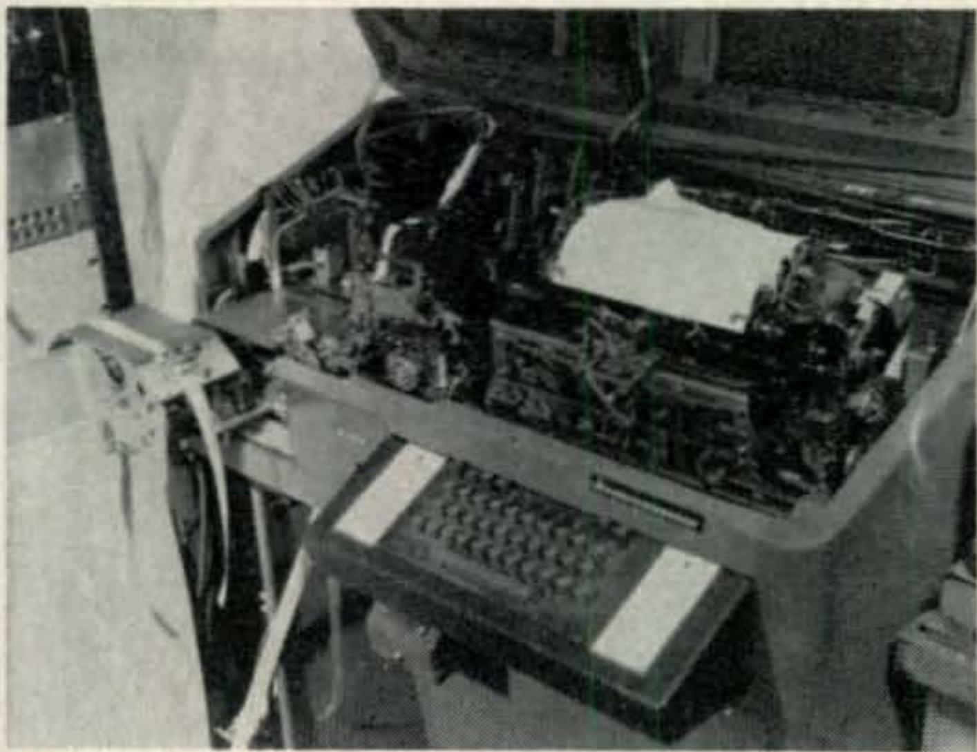
The "Full House" model 28 ASR with LCXD Transmitter-Distributor; Auxiliary Reperforator, with 8-speed Gear Shift, Page Printer with Shift, and Keyboard Perforator.
