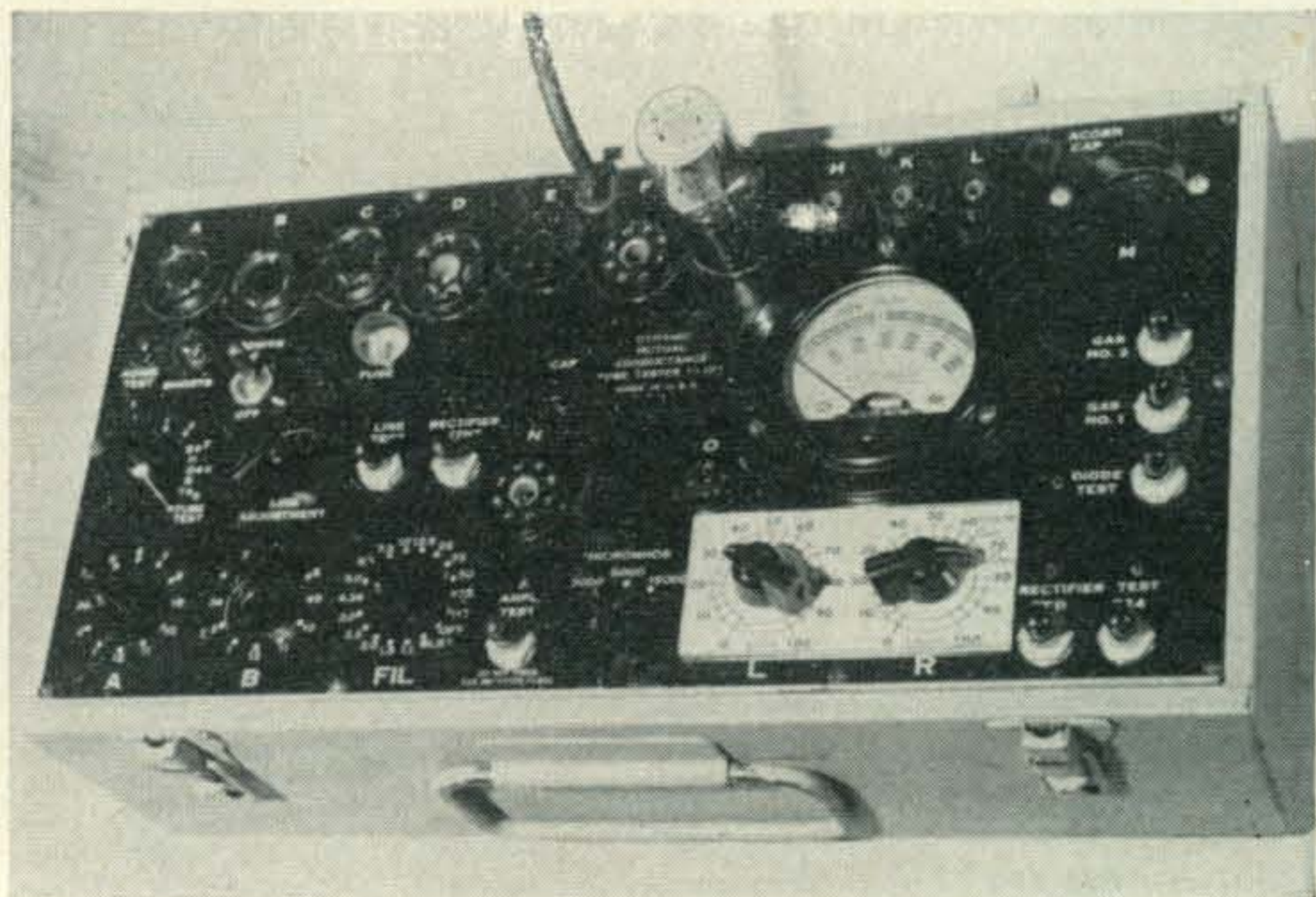
View of a modified I-177 tube tester, a surplus unit found in many ham shacks today.
