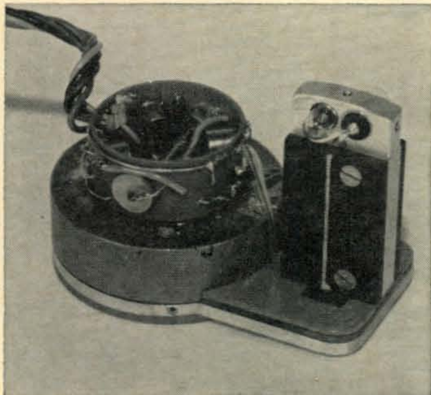
Inside view, showing circular parts board, pedestal and lamp assembly.
