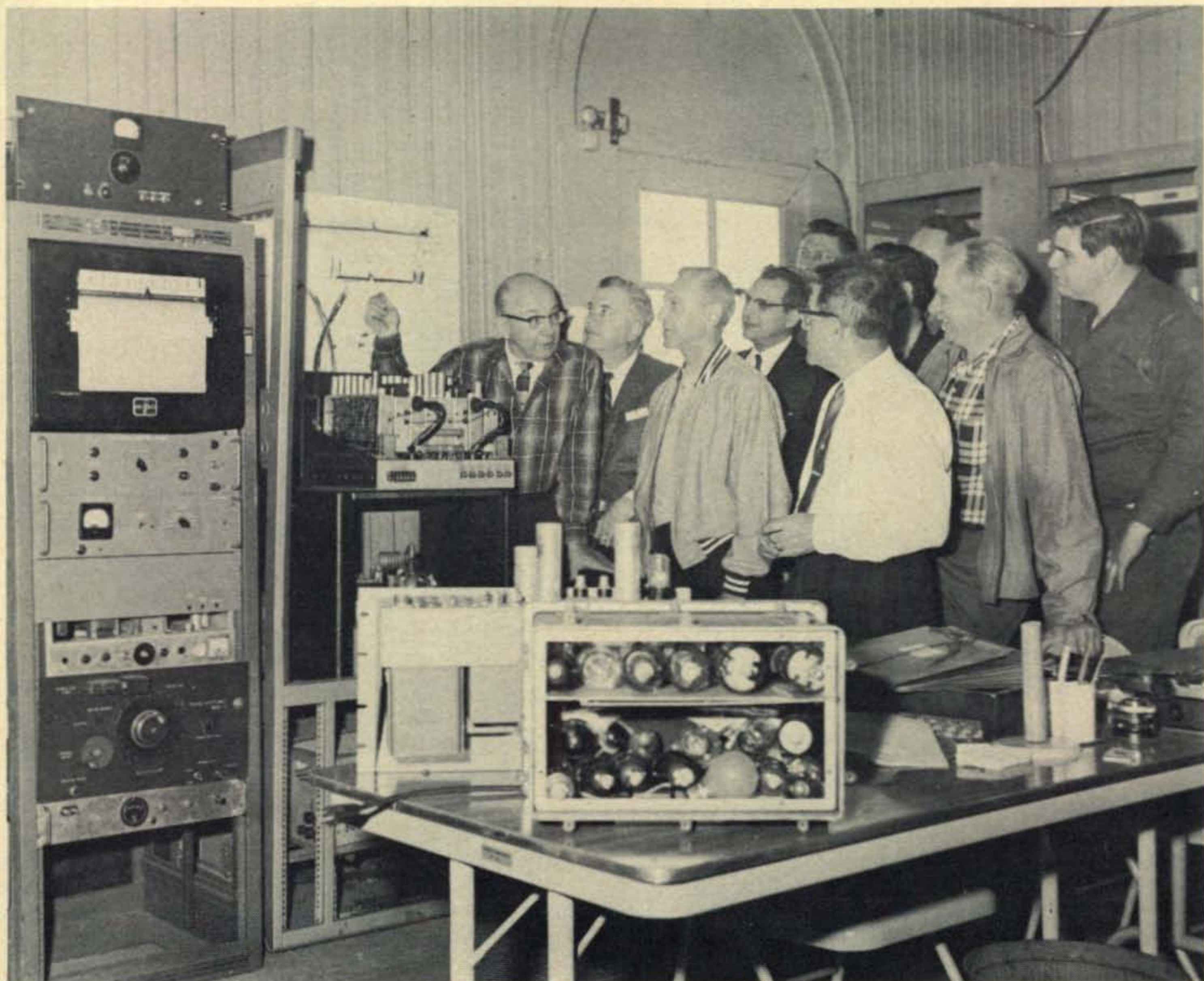
W6OLO/2 and NASTAR members check OSCAR frequency chart. Left-hand panel holds Bristol paper recorder for satellite passes.
