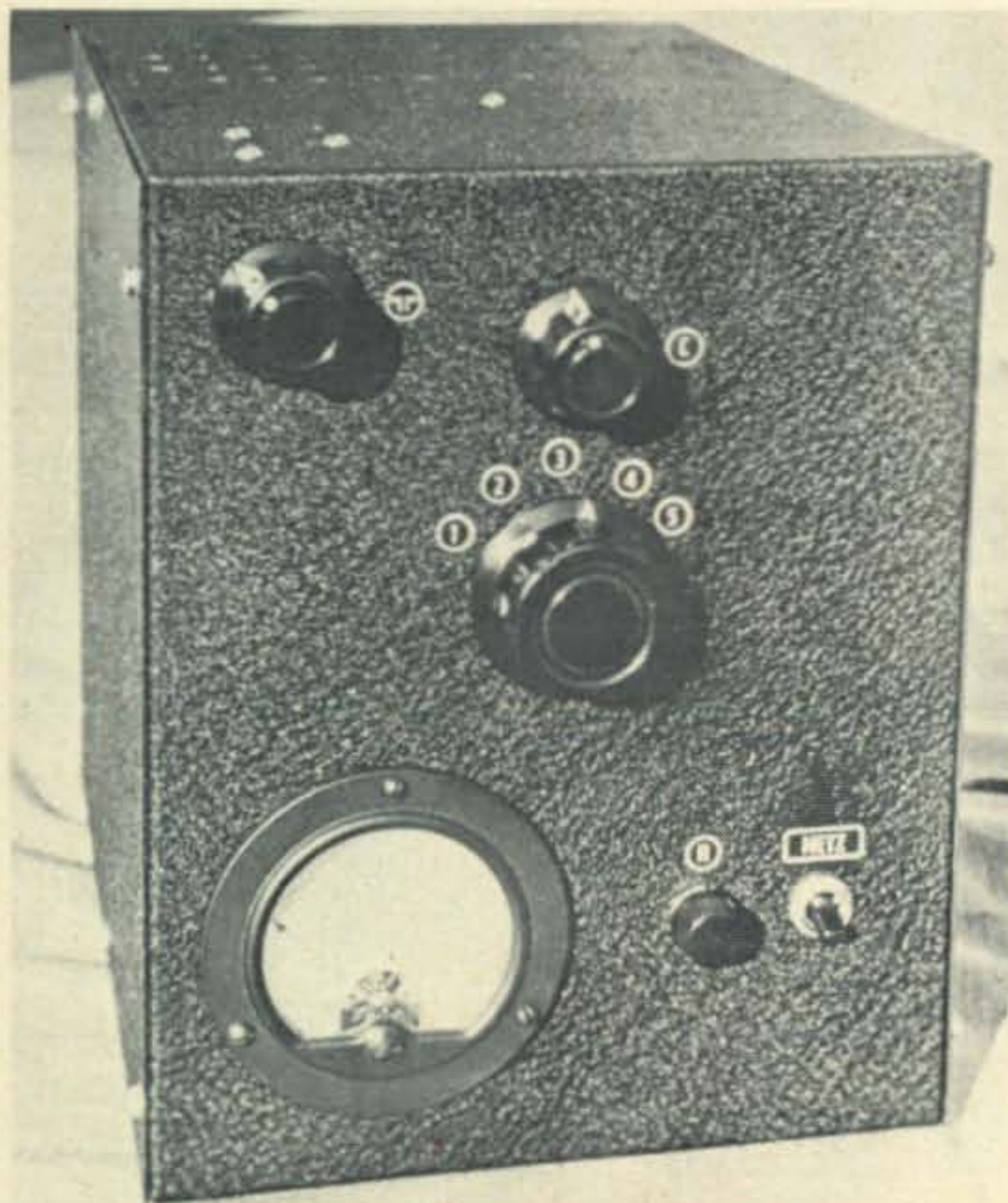
Front view of the Shoebox II linear. Although similar in concept to the earlier Shoebox linear, the Mark II features more flexibility of operation and ease of construction. Inexpensive 6HF5 tubes are used in parallel to deliver as much power as the builder desires.
