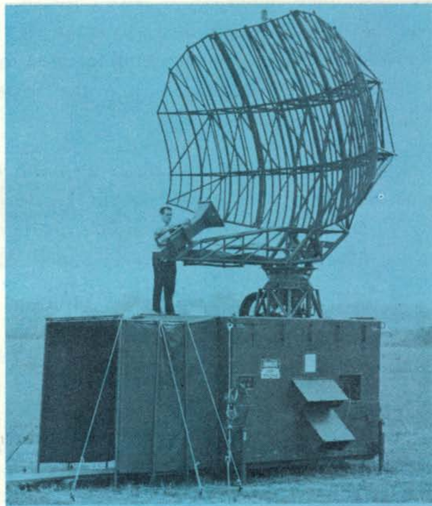
Typical semi-parabolic rotating radar antenna, in this case, that of the AN/TPS-44 Radar Set. Note, next to the man, the size of the "L-Band" waveguide and the horn feed. Photo courtesy of Cardion Electronics Inc.
