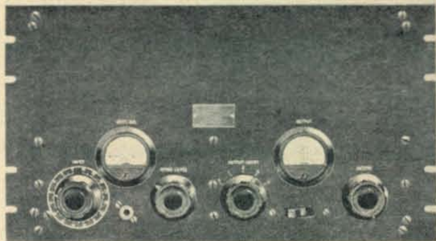
Fig. 5—Boehme recorder drive unit. This piece of equipment converts the audio signal to a d.c. impulse to drive the recorder magnets.
