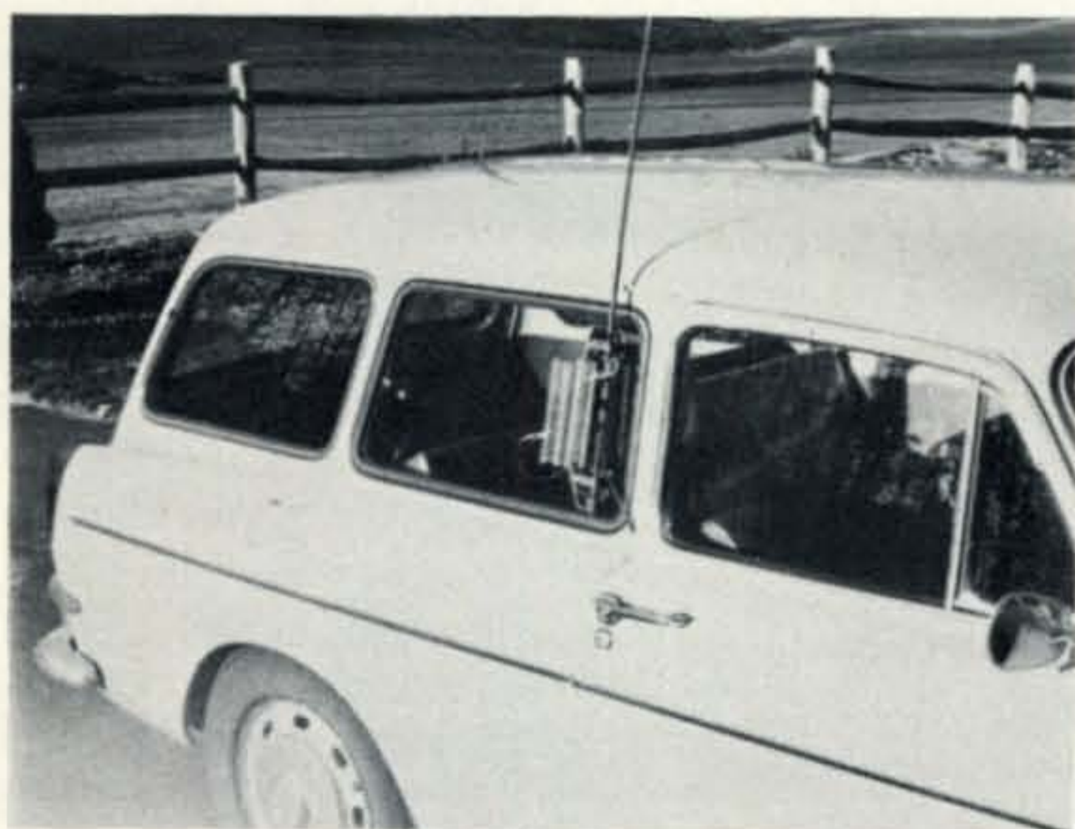
The suction-cup portable antenna mounts quickly on the windowpane of any automobile in a matter of seconds.
