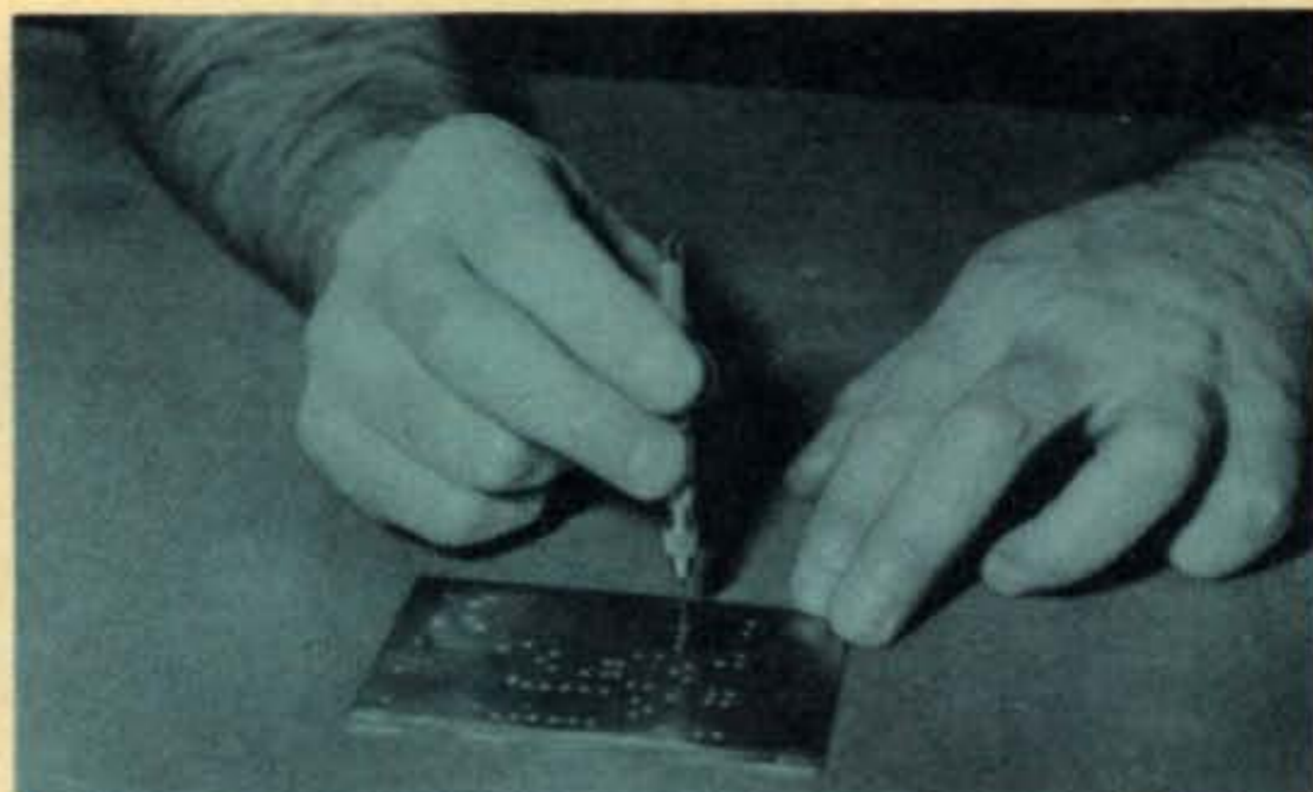
Fig. 5—Drill the locating holes with a #55 drill in a pin vise. A small hand held high speed rotary drill would be better if it is available.
