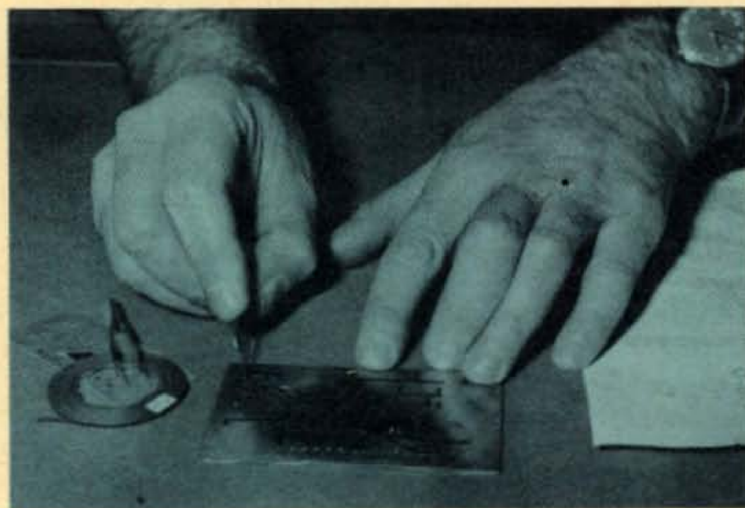
Fig. 6—Run the connections together with 1/16" tape (Lafayette #19C 6813—75¢) and cover the holes with tape (areas not to be etched). Lafayette also has 3/16" disc tapes (#19C 6816—75¢) if you would prefer them. Some constructors prefer to drill after the etch bath but I find the holes a good reminder as they prevent me from forgetting to tape a line to the hole. Every drilled hole must connect somewhere.
