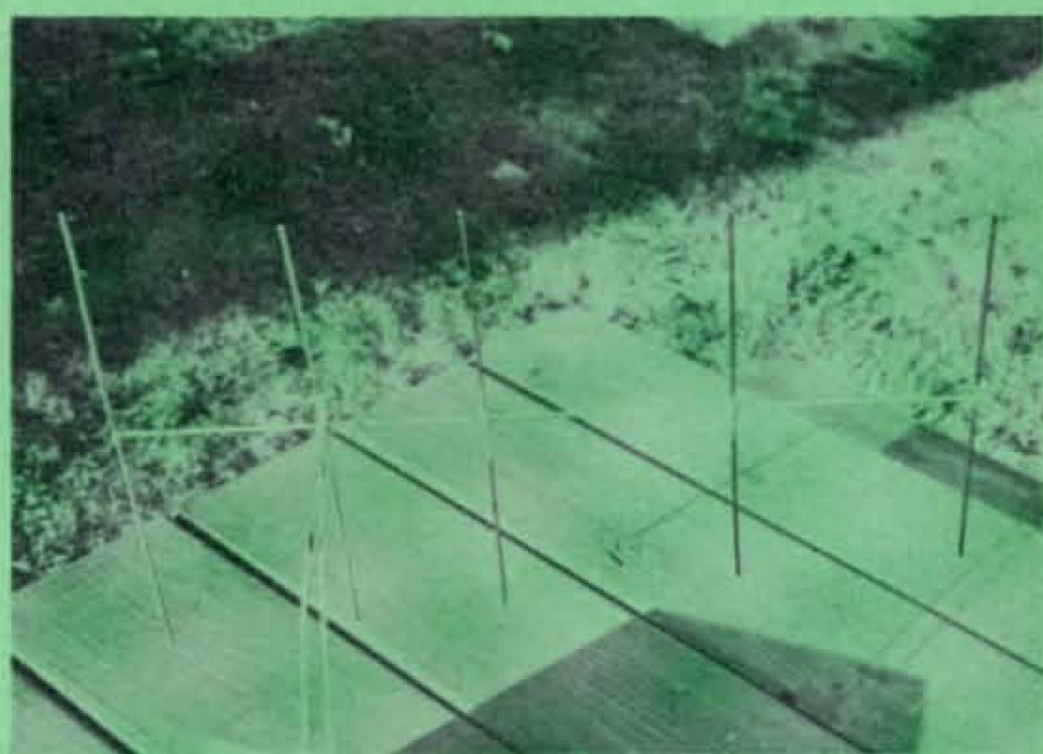
An example of a simple model constructed from stiff wire to study a yagi configuration. This test antenna was cut for 700 mc.
