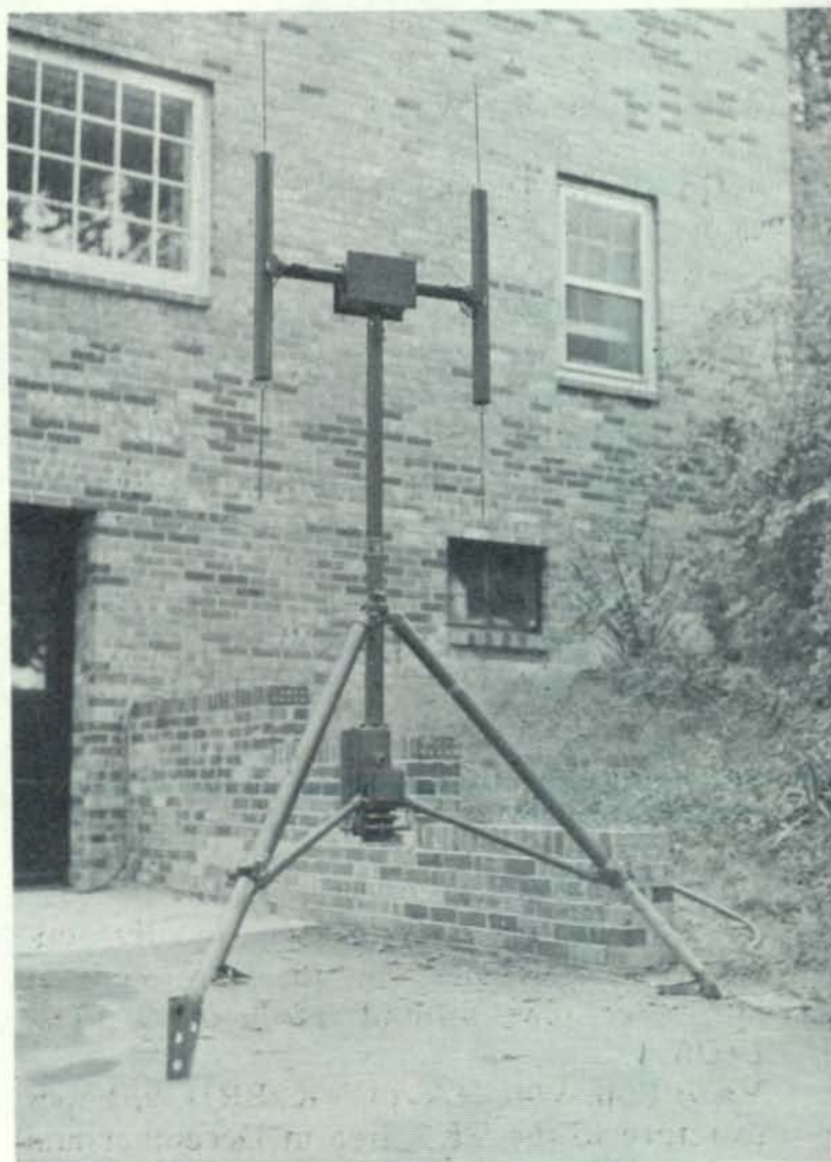
Fig. 1—AN/PRD-7 surveillance antenna, showing 4-element beam mounted on the mast. An additional section of mast is normally used, but was omitted for the photo above. The beam covers 100-200 mc.
