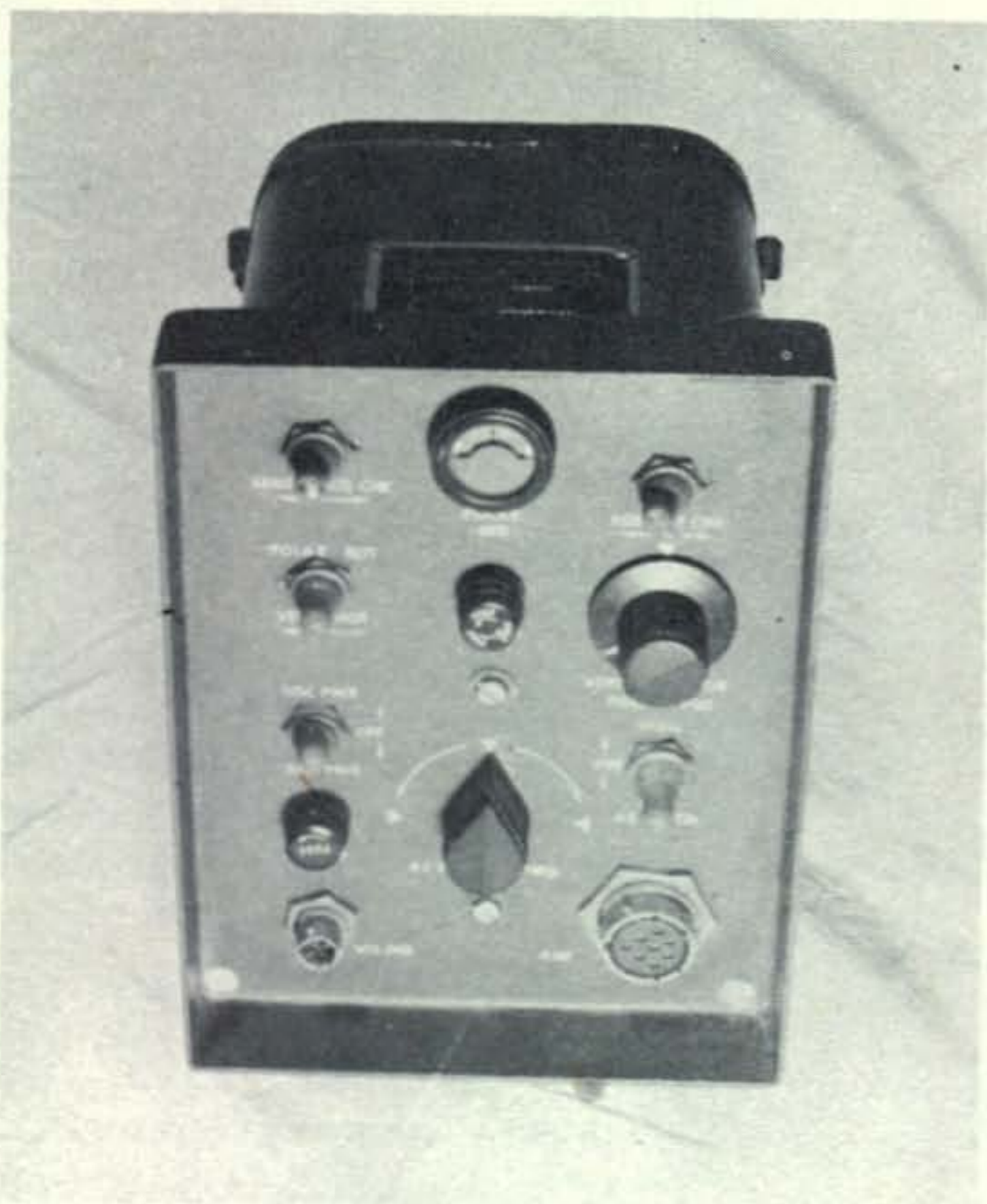
Fig. 2—Control box for AN/PRD-7 antenna. Unit requires 28 volts d.c. and connects through a multi-conductor cable to the antenna itself, providing fuses, switches, azimuth and polarity controls.
