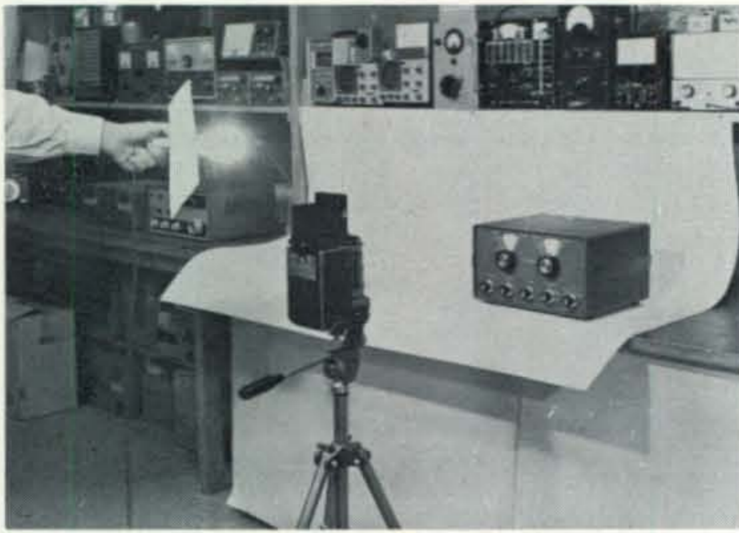
Fig. 8 — Painting-with-light setup. A single hand-held light is continuously moved about the subject during a time exposure. A small piece of cardboard at the rear of the lamp serves as an eye shield.
