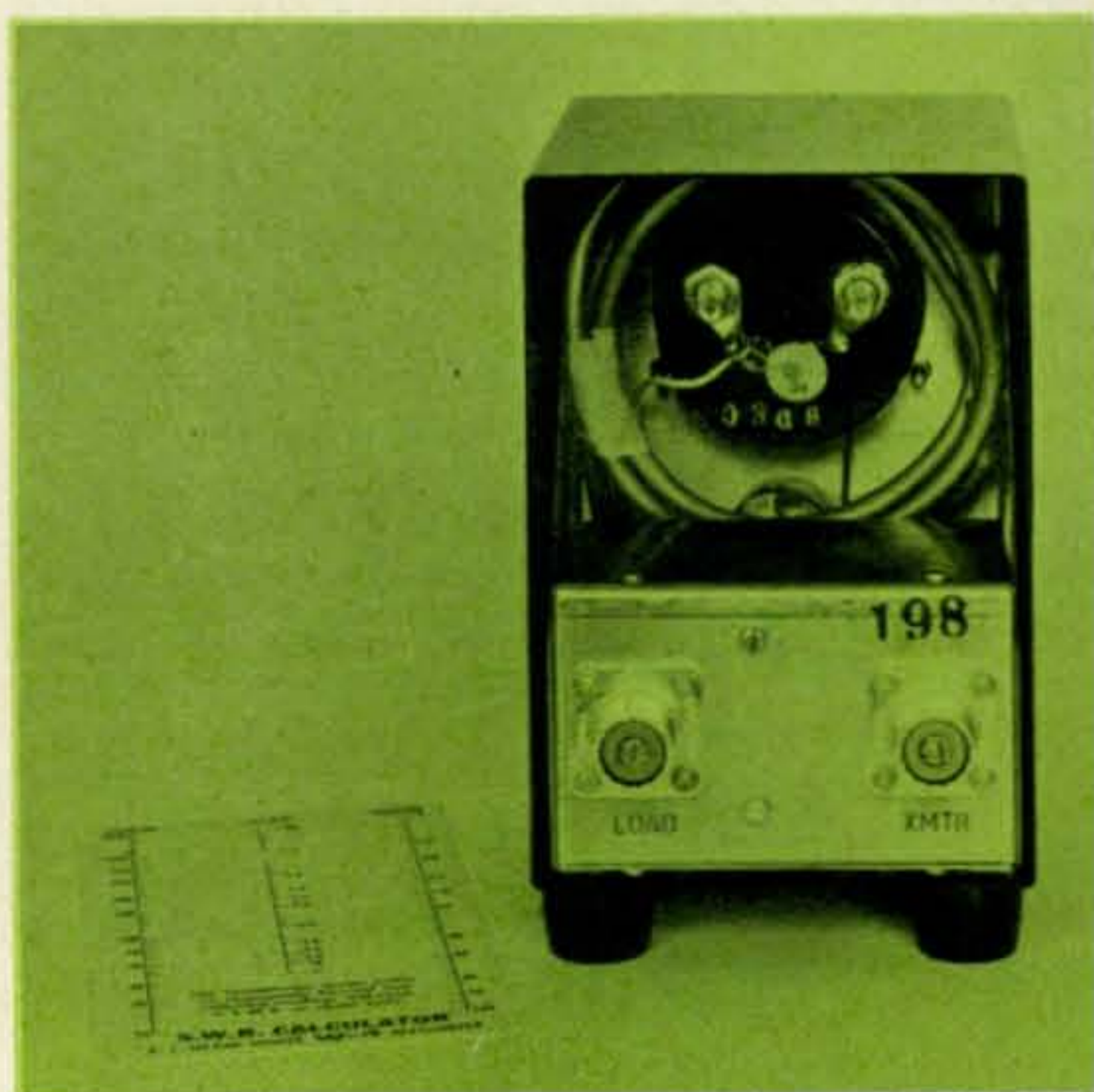
Rear view of the W-4 Wattmeter. The removable sensing coupler mounts in the bottom of the case in the upper part of which may be seen the attached inter-connecting cable coiled up. The s.w.r. calculator is at the lower left.
