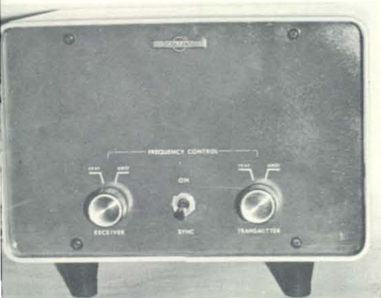
Front view of the new control panel placed in the Collins 312B-3 cabinet.
