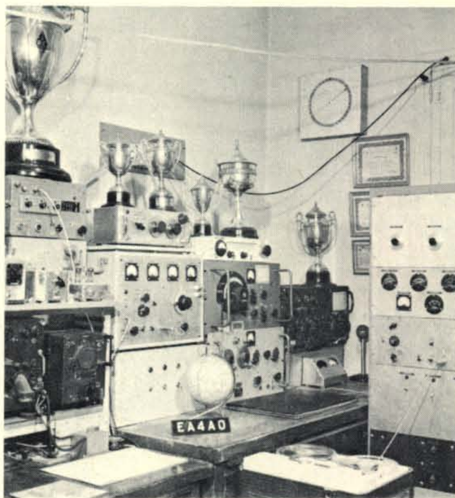
In the rack on the right is the 260 watt, 144 mc. transmitter used by EA4AO to successfully complete more than a half dozen two-way QSOs through OSCAR-3. Two British vhf receivers and a home made vhf transistor receiver are among the equipment on the main table. The trophy's attest to the many contributions made by EA4AO to amateur radio.
