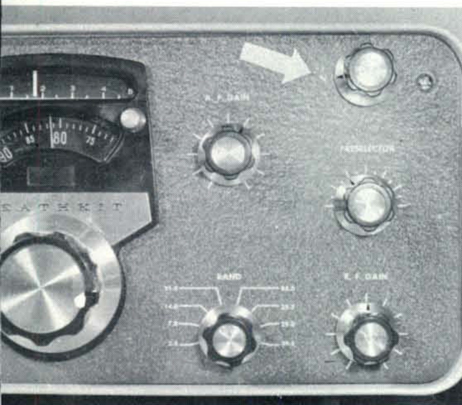
Fig. 1—Location of the preselector control knob added to the Heath SB-300. The pilot light is just to the right of the arrow.
