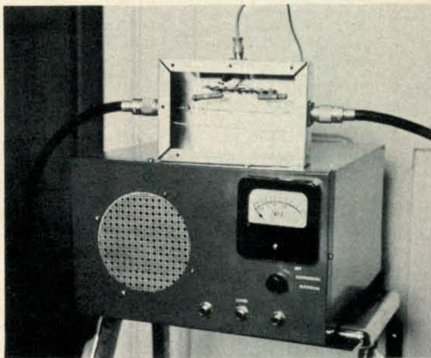
View of the interior of the in-line section placed atop the station speaker housing that also contains the output indicator. Connection is made to the meter by the shielded cable plugged in on top of the unit.
