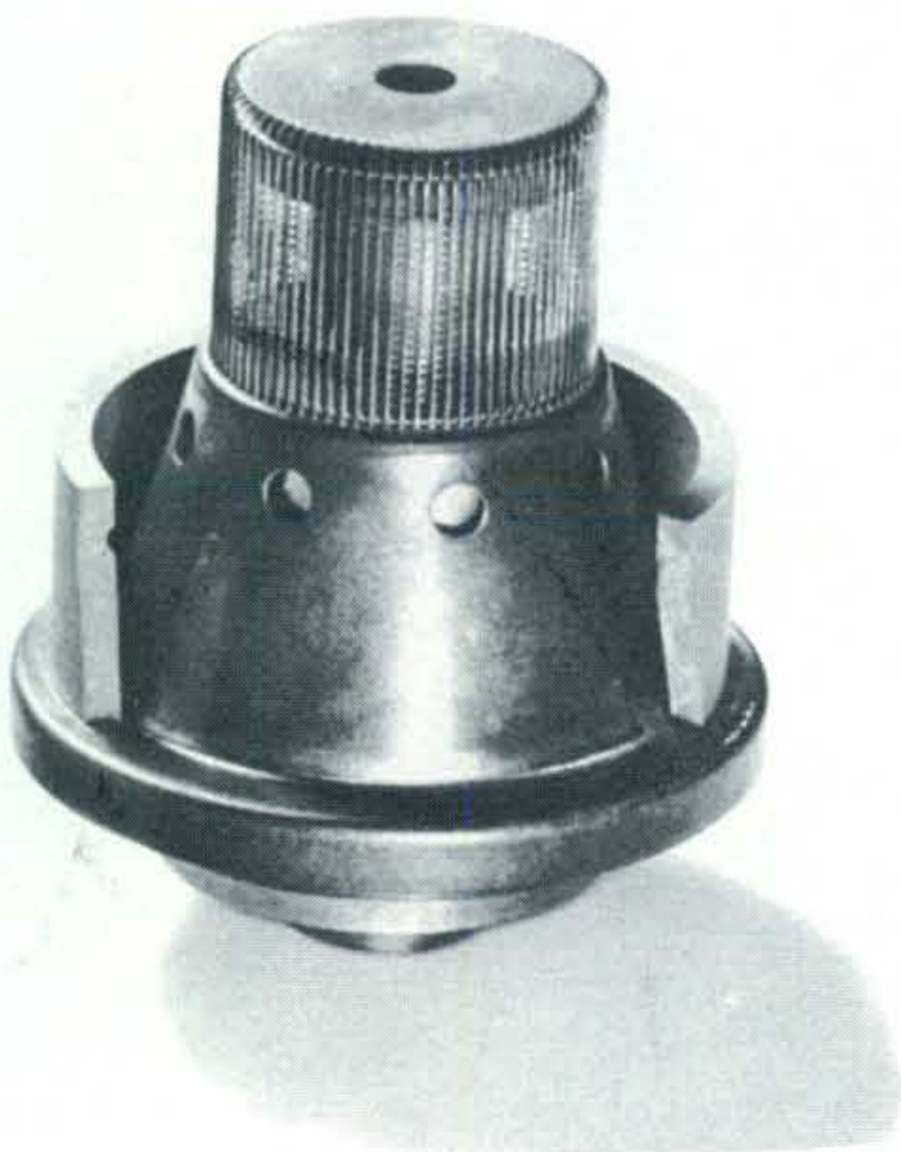
Fig. 3—Partial cutaway of the grid assembly of a CERMOLOX® tube.
