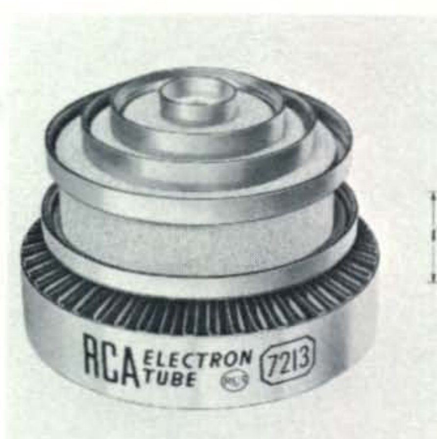
Fig. 4—The 6816 was the first of the tubes with aligned grids and was followed by the 7650 and 7213.
