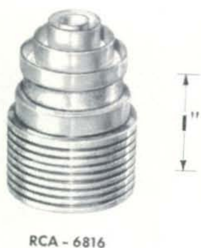
Fig. 4—The 6816 was the first of the tubes with aligned grids and was followed by the 7650 and 7213.
