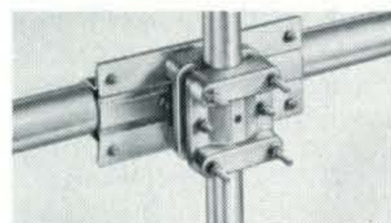
Tilt-head, universal boom-to-mast bracket —all new, cast aluminum bracket accommodates masts from 1 1/4" x 2 1/2". Allows easy tilting for installation, maintenance and tuning, provides mast feed-thru for beam stacking.
