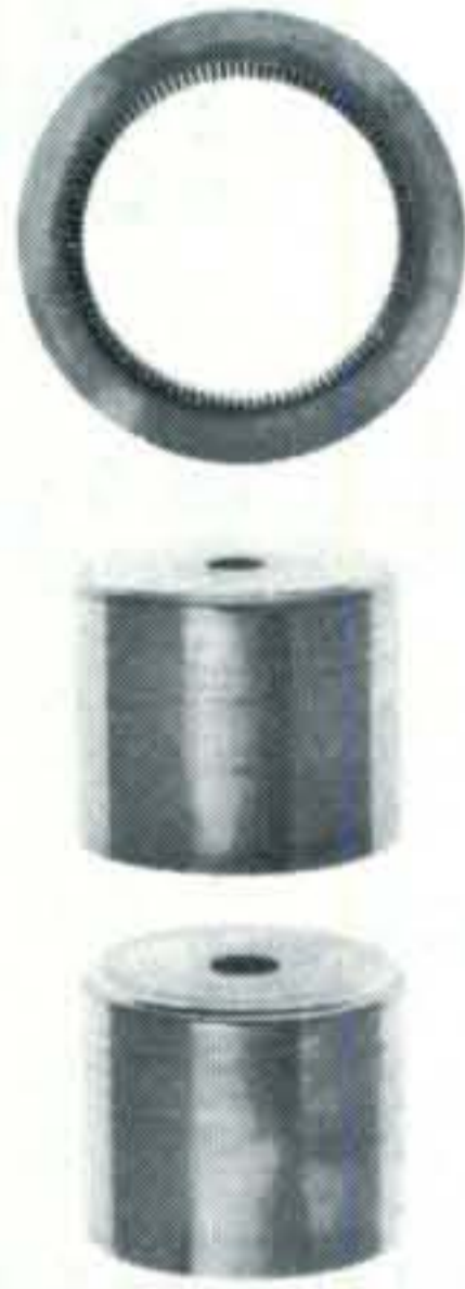
Fig. 2—The electrical discharge machining tool and the G_2 and G_1 grid cups are shown before machining.
