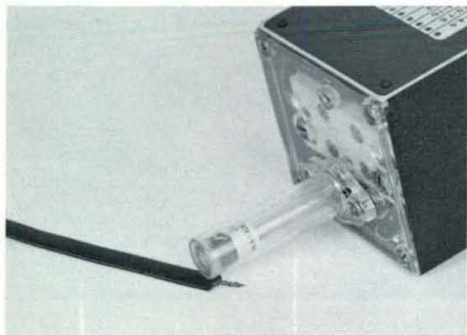
Method of coupling g.d.o. to shorted twin lead.
