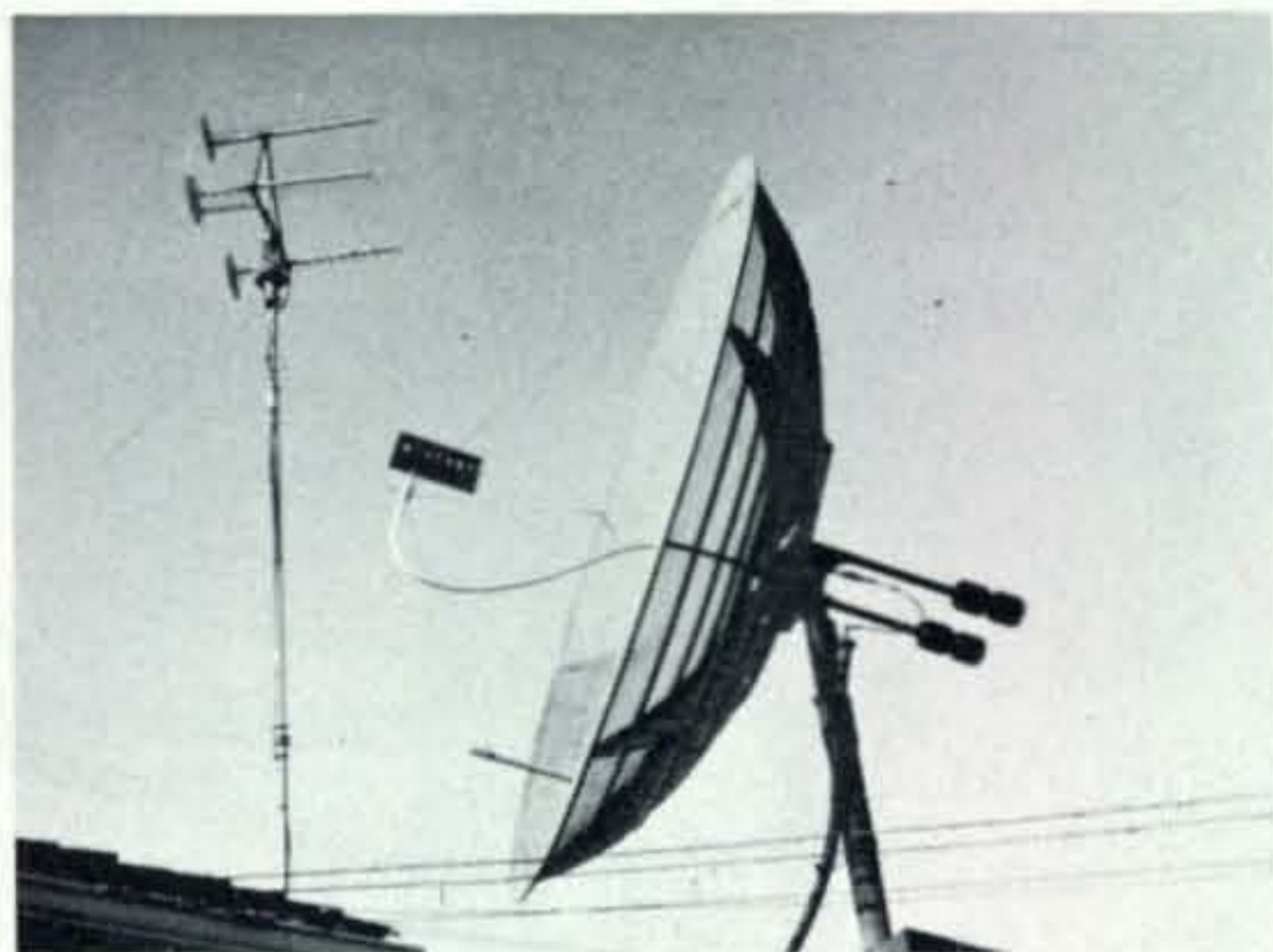
The ten foot parabolic reflector dish shown mounted on a polar mount was used by Peter Laakmann, WB6IOM, to work the Crawford Hill VHF Club, W2NFA, on April 12, 1968. Below, Peter is shown in front of the dish.
