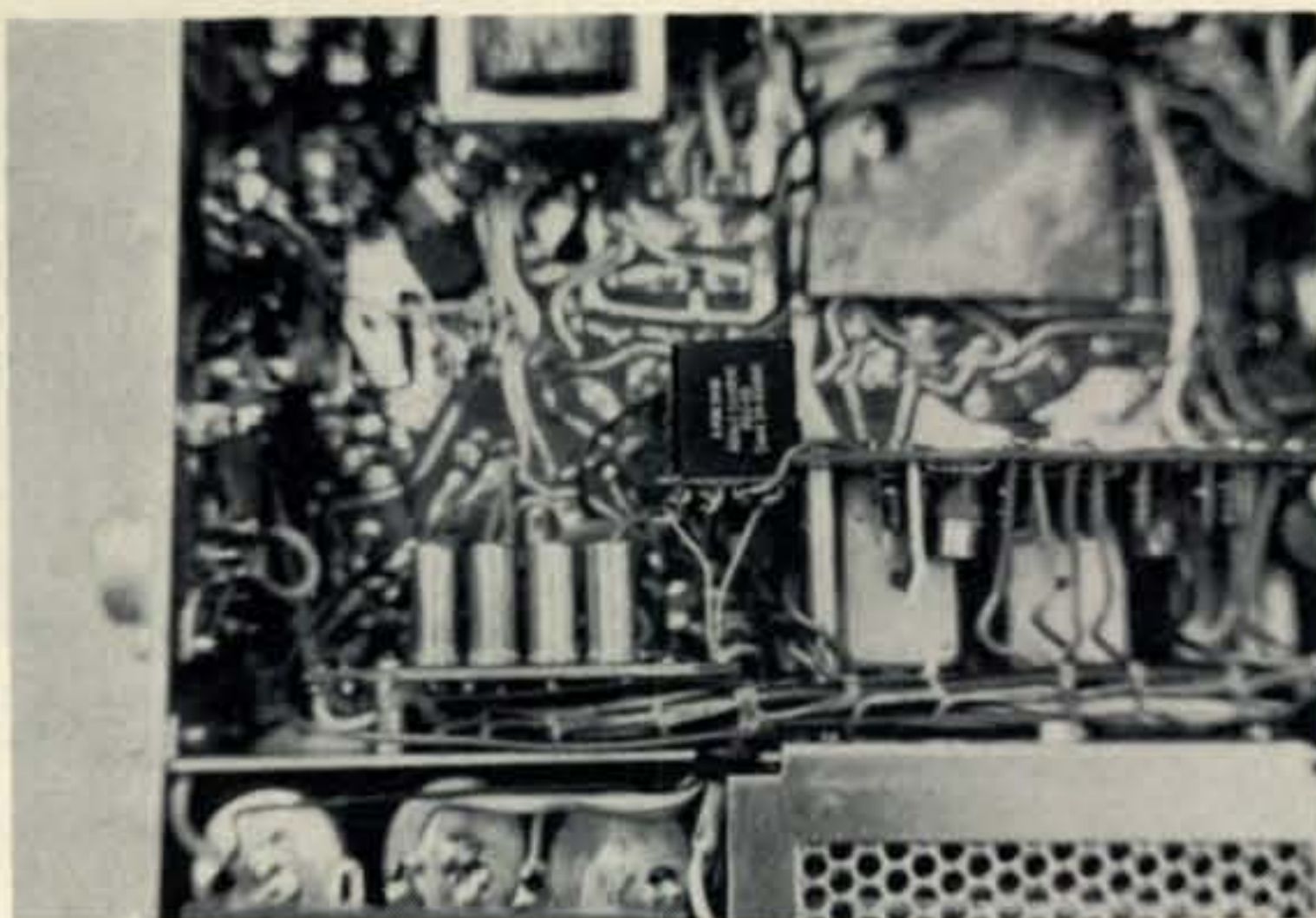
Crystals for c.w. coverage of 15 and 20 meters are mounted on a piece of vectorboard directly below the crystal can relay.
