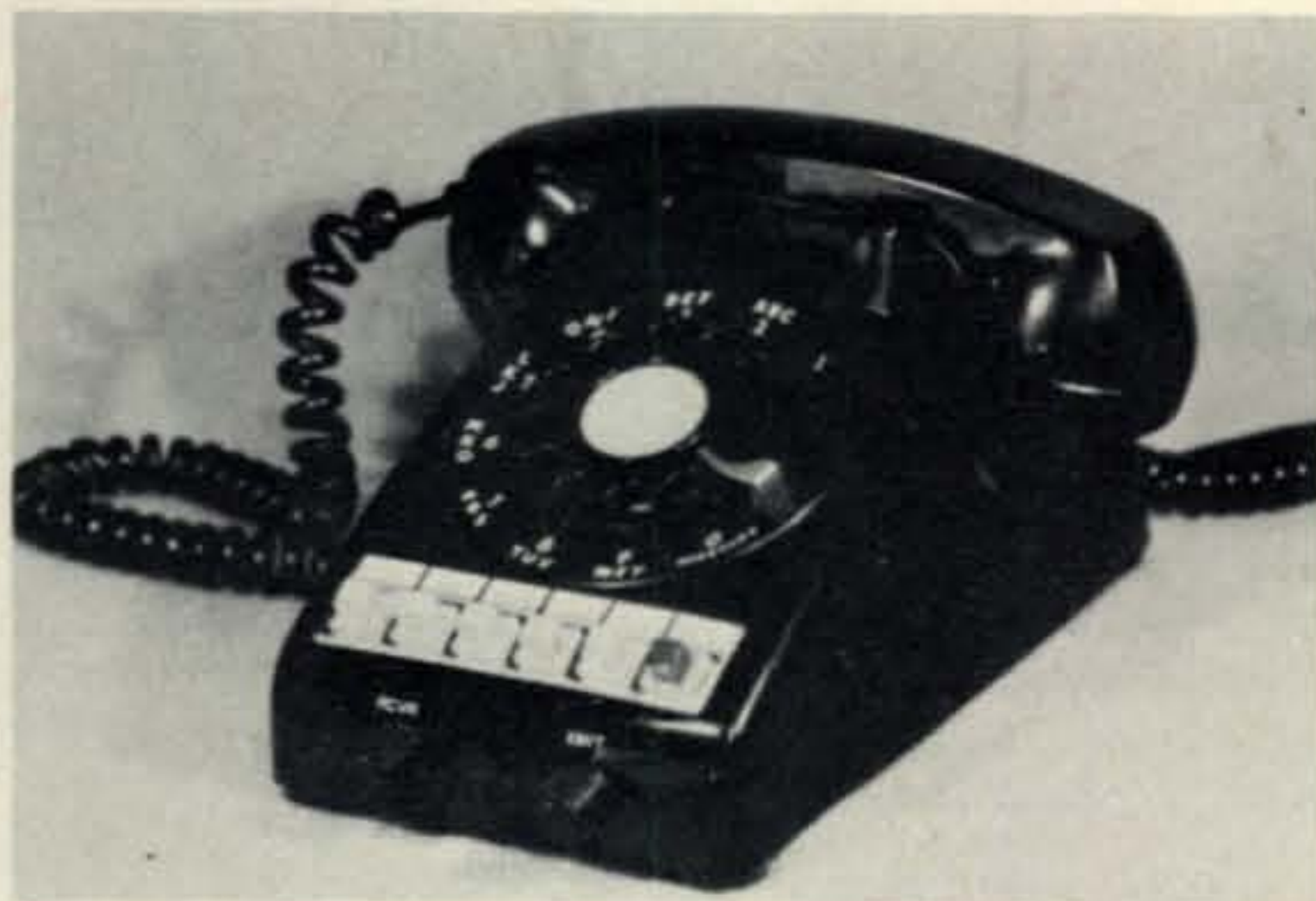
Fig. 13—The complete Phoney patch. The two knobs are the only obvious modifications to the telephone.
