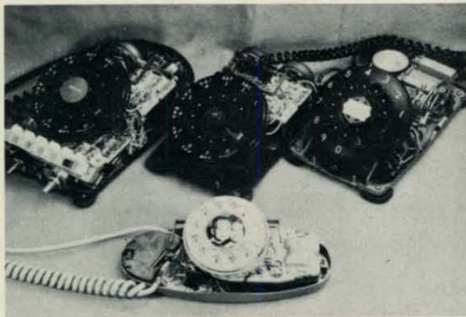
A sampling of the phones which may be modified into Phoney patches. The three larger phones are, from l to r, W.E.564HL, and 518, and the Automatic Electric 802. In front is the W.E.701 Princess.
