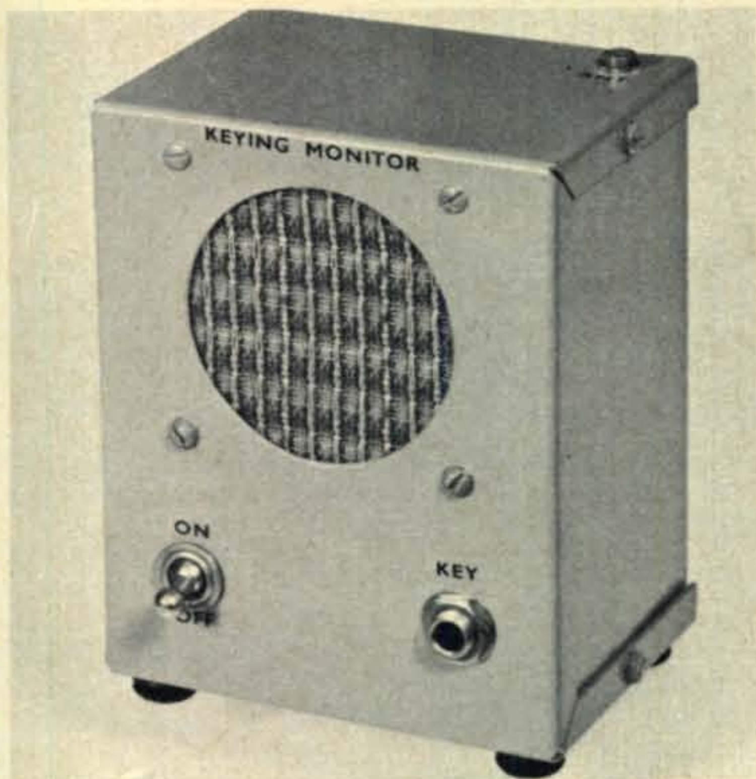
Front view of the completed r.f. actuated keying monitor mounted in a 3×4×5 aluminum Minibox.
