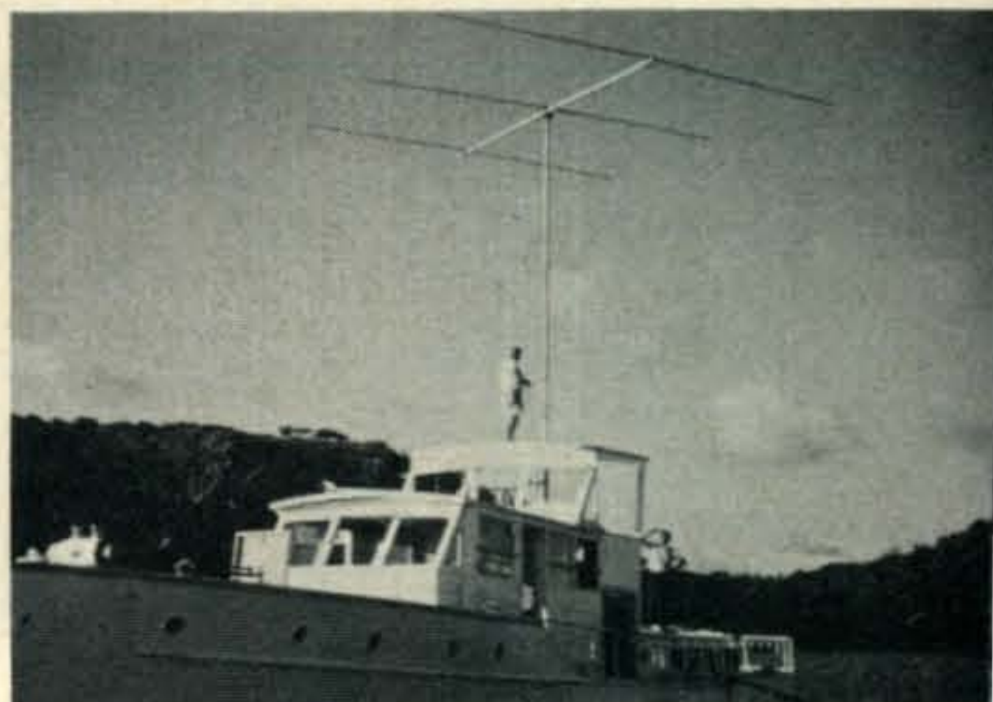
A 15-meter beam was erected atop a beach yacht. PJ3CC mans the feedlines.
