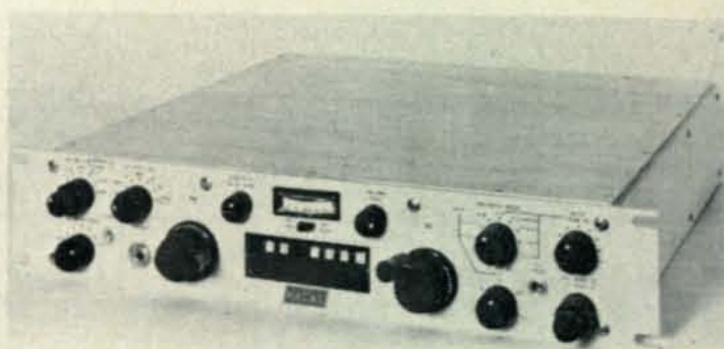
The Racal Co. 217 receiver has digital frequency readout but it is controlled mechanically from the rotation of the MC and KC tuning knobs using veeder root counters.
