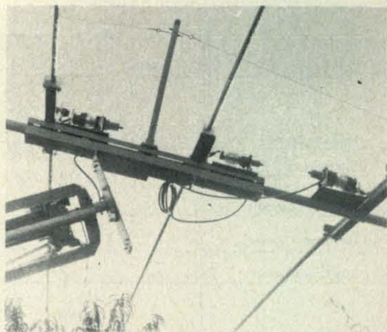
Fig. 7—Photograph showing door hinges on a heavy steel plate permitting the boom to remain horizontal with the tower tilted.
