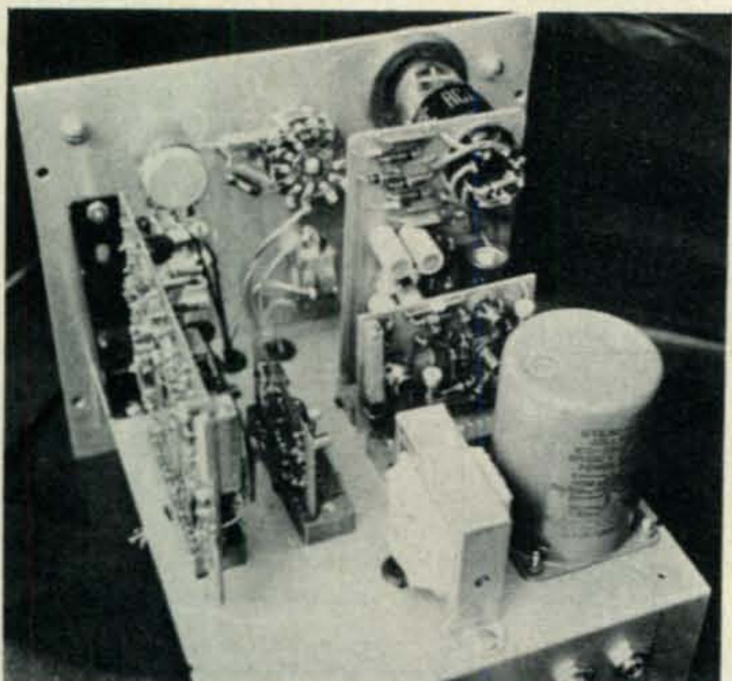
Rear view of the RTTY TU showing the card placement. The front right card is the Indicator-Power Supply with the Output card behind it. The Detector card is on the extreme left and the Trigger card is in the center.
