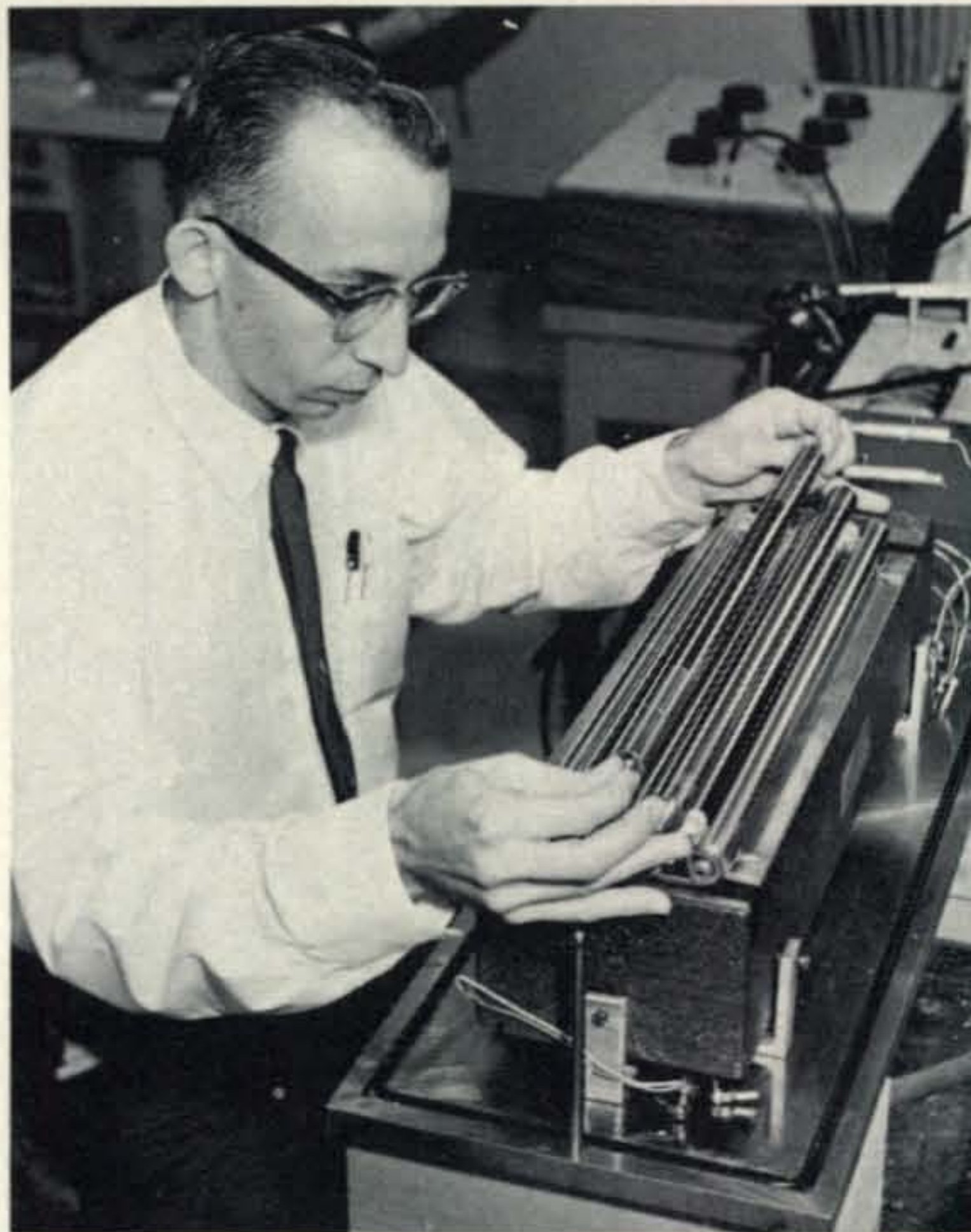
Exactly dimensioned capacitors are used to calibrate the National Reference standard for the ohm. (N.B.S. Photo)
