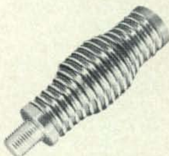
Miniature Spring. Stainless steel. Double tapered design. Handles whips up to 52" long. Accepts \frac{3}{8} " x 24 thread fittings.
