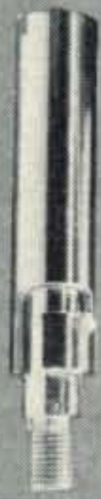
Quick Disconnect. Flip-of-the-wrist removal and attachment of mobile whips. \frac{3}{8} " x 24 thread fittings on both ends for permanent attachments. High-tension spring loading. Heavy chrome plating.
