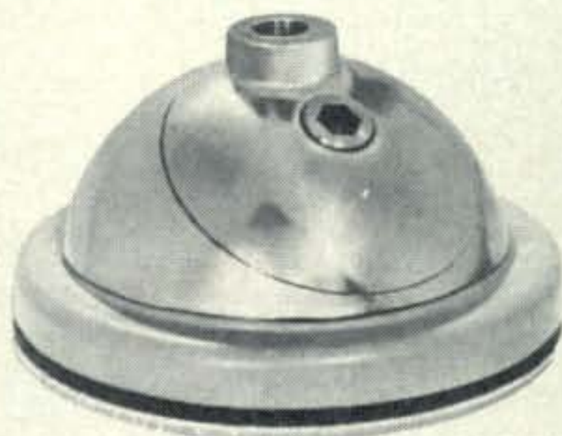
Exclusive Flush Body Mount. Chrome-plated with cyclac base, rubber body washer, heavy-gauge back-up plate. Rugged support. Accepts \frac{3}{8} " x 24 thread fittings.
