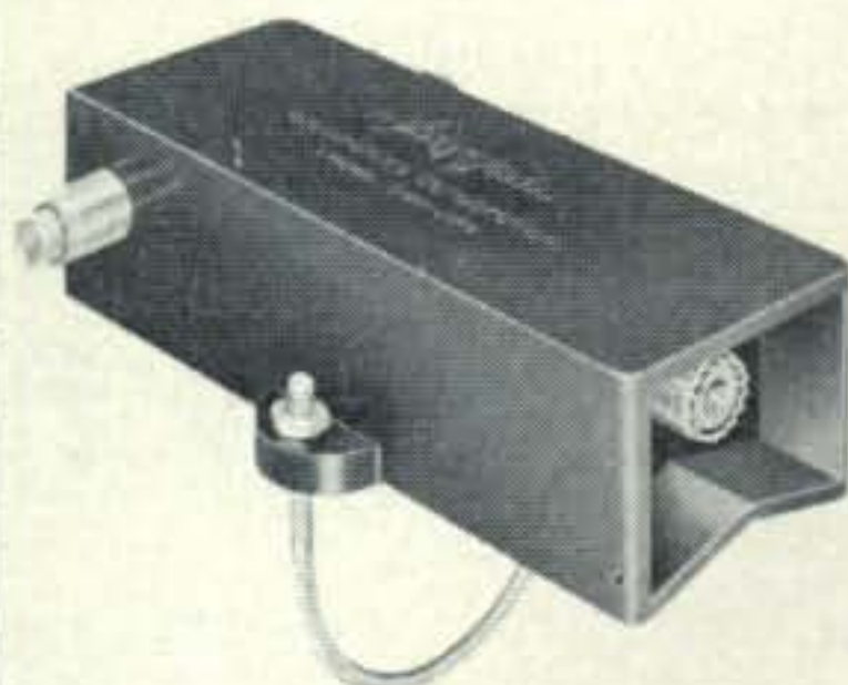
Broad Band Ferrite Balun. For beam, doublet installation. Couples 52 ohm unbalanced system with 52 ohm balanced system. Use with any beam 3 to 30 MHz.
