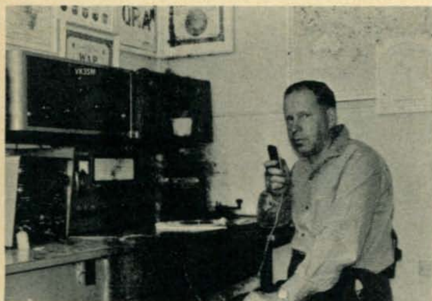
The neat set-up, down-under way, of Allen, VK3SM. On the top row is an antenna switching device, a low pass filter and an Australian Air Force AR-7 receiver. On the bottom row is a homebrew power supply, K. W. Viceroy transmitter, and Drake 2B receiver.
