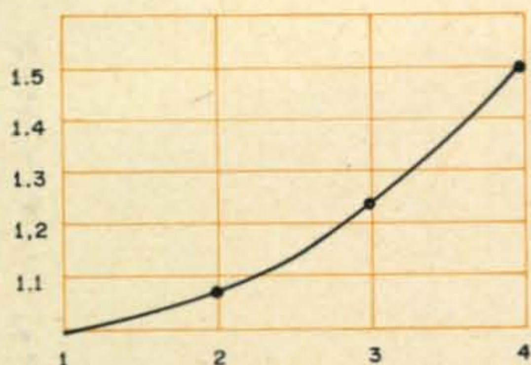
Fig. 2—Graph used to relate various power levels for an amplitude modulated carrier. It is not applicable to s.s.b. transmission.
