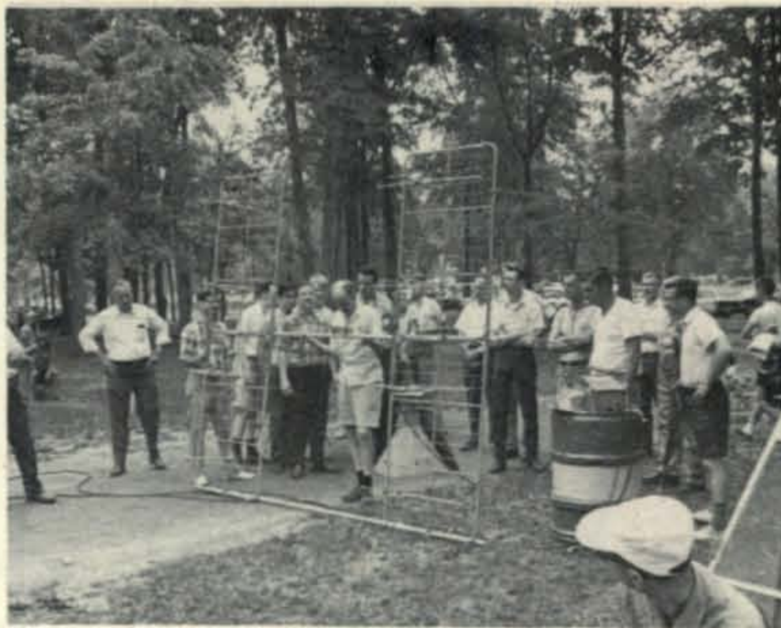
Bill, K2TKN with contest winning 432 mc 48 element collinear yagi array and screen reflector. Picture taken by Rich, K2RIW at Central New Jersey VHF Society's antenna measuring contest.
