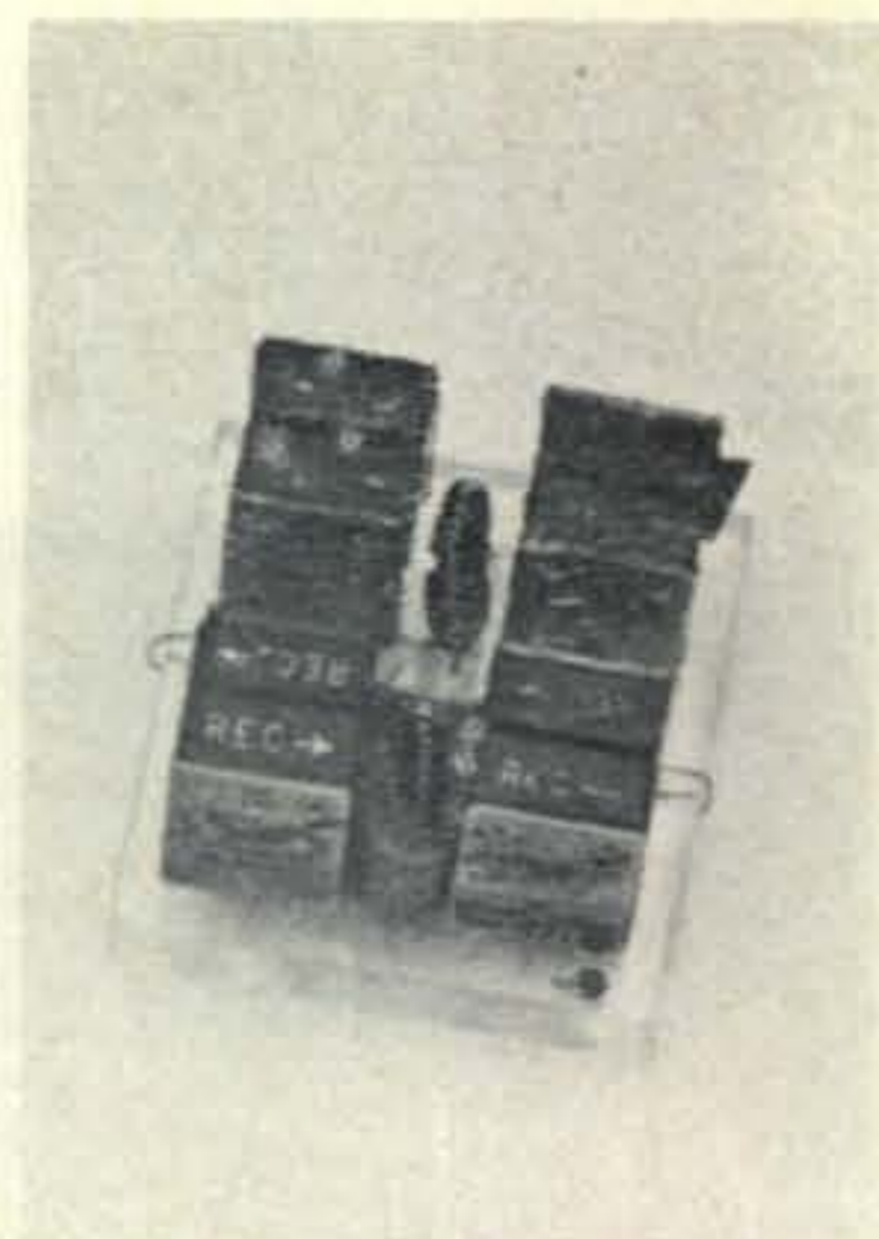
Fig. 2—Top view of the crystal filter and the torroid coils.
