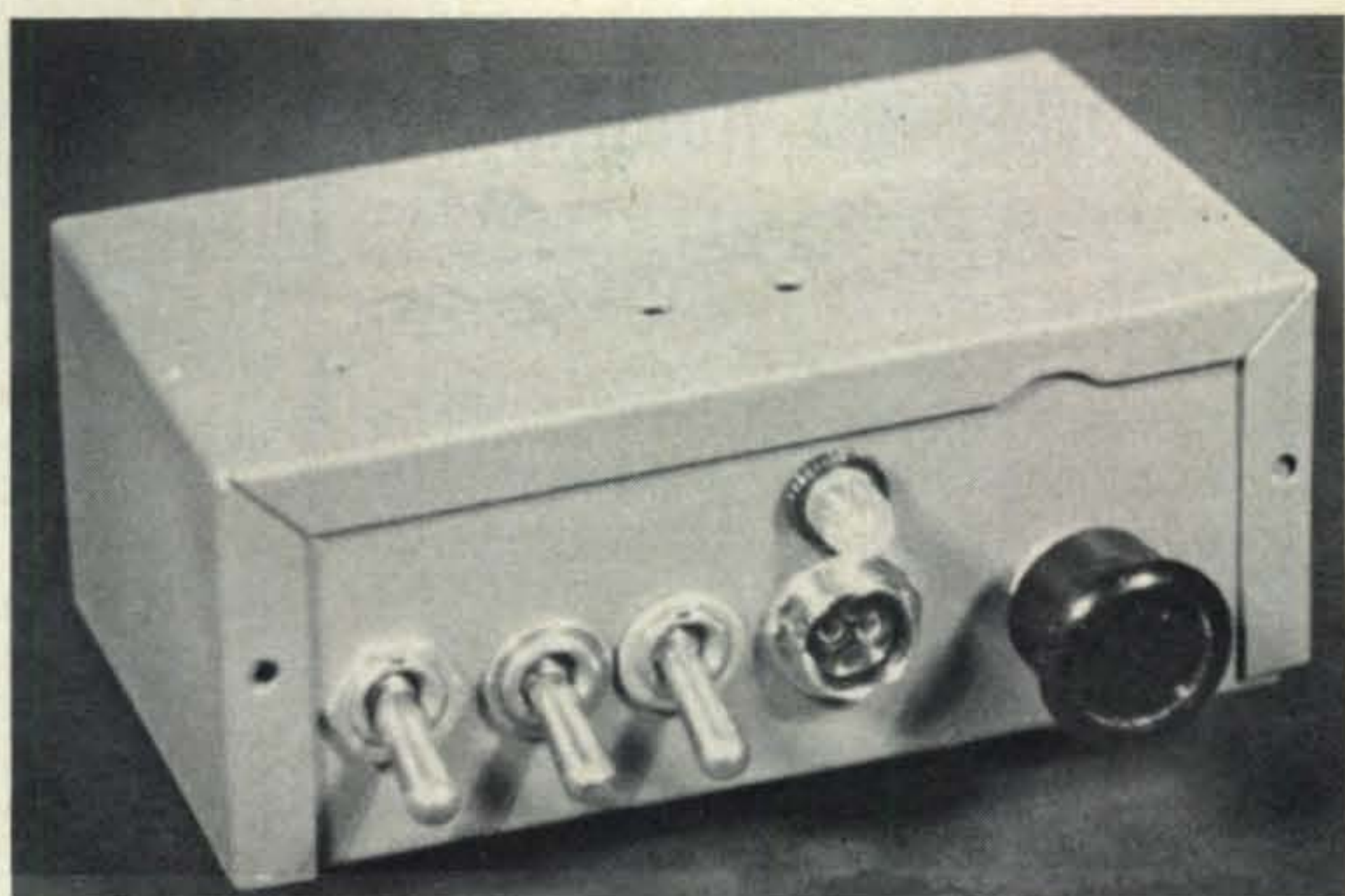
Fig. 7—View of a control head for mobile operation of the Raytheon 21TR11A. The circuit for this unit is shown in fig. 8. The controls are, from l. to r., S_1 , S_2 , spare, Mike, Volume. The neon indicator above the Mike plug indicates the presence of B plus.
